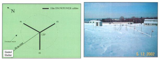
Figure 2 : Star shaped installation of the SNOWPOWER cables
