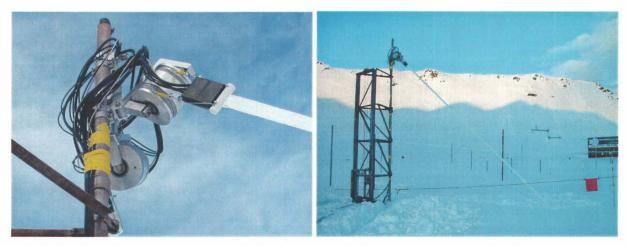
Figure 1 : The cable sensor system at Weissfluhjoch Davos (2550 m): the new suspension of the sloping cable (left), which is now installed in a 45° angle (right).
