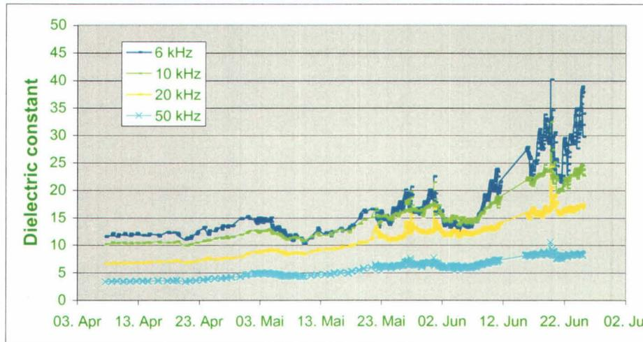
Figure 13 - Dielectric constants at low frequencies (6, 10, 20, 50 kHz) determined with BSI at the Swiss test site
