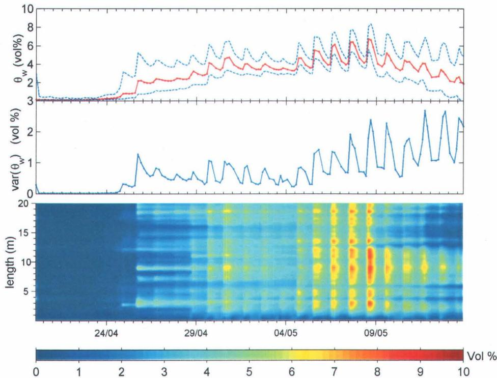
**Figure 16** - Preferential flow patterns detected with the high frequency (TDR) measurements of the SNOWPOWER sensor.
