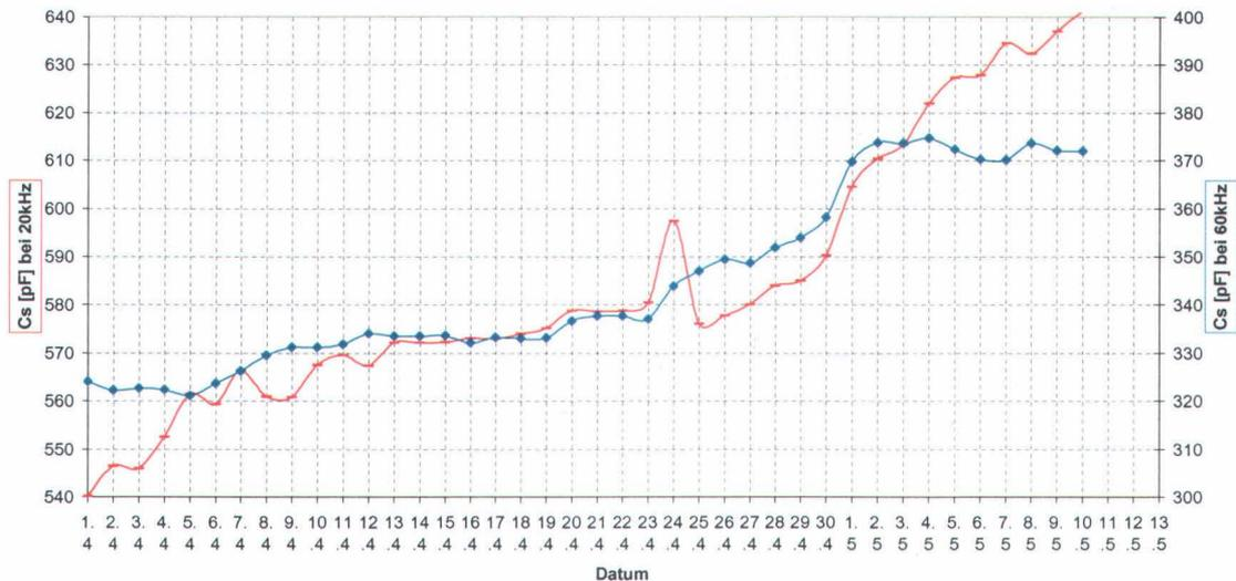
Figure 11 - Measured capacities at 20 and 60 kHz with the first BSI prototype
