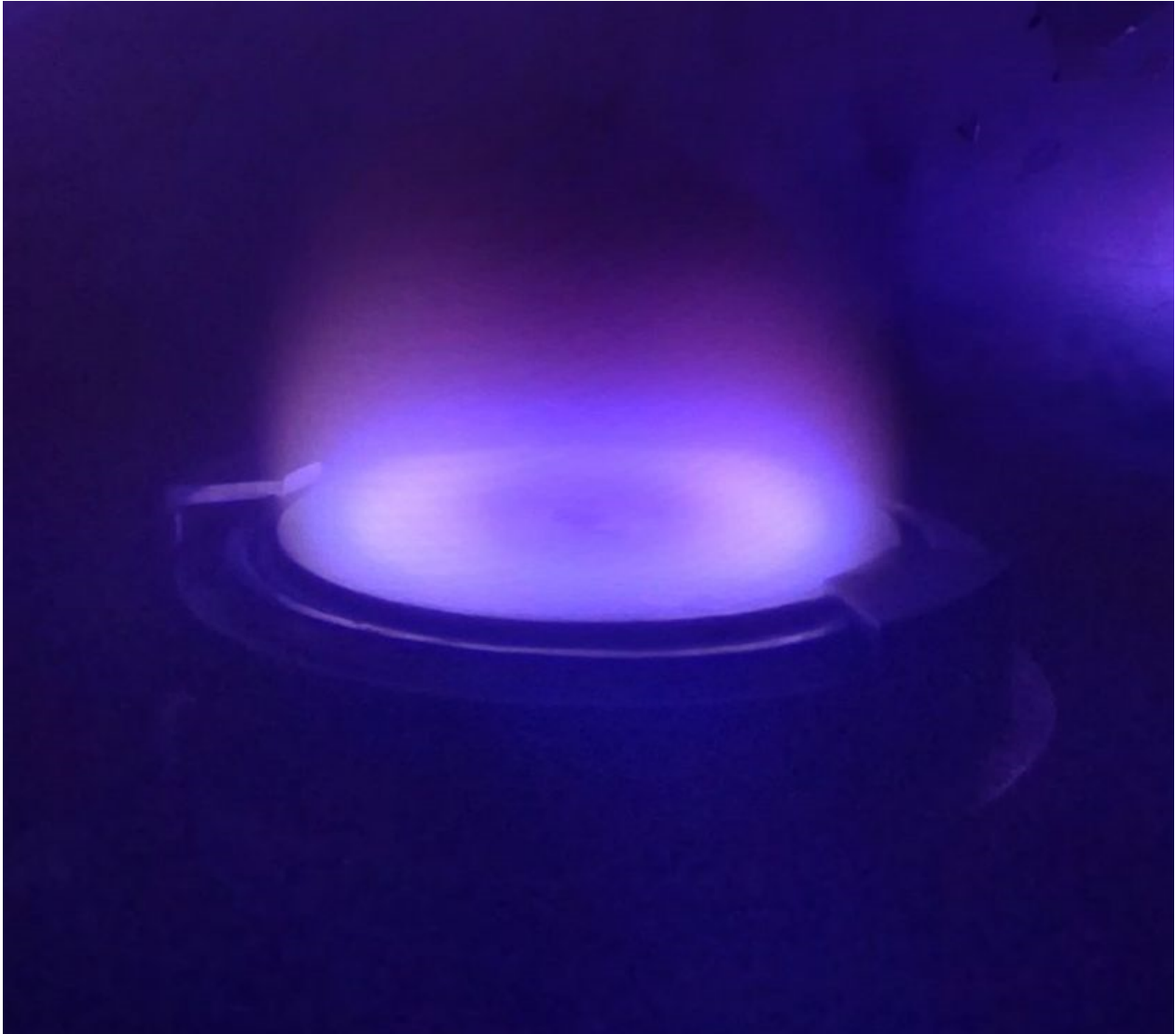
Figure A.2 – View of a toroidal plasma plume produced by a running magnetron-sputtering gun in a vacuum chamber. Adapted from Wikimedia Commons (following CC BY-SA 3.0).
