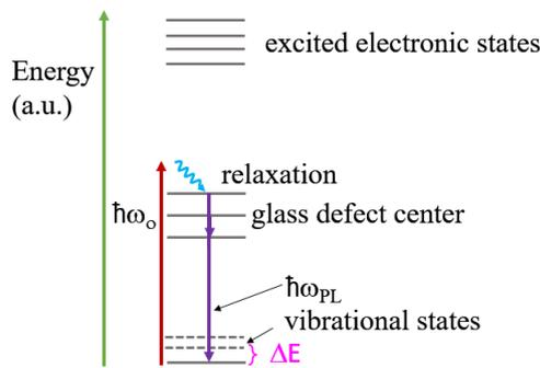
Figure 3.5.1: Jablonski diagram for photoluminescence in glasses. Since the energy of the excitation can be higher than the absorption of the glass defect, relaxation processes (Stokes shift) can occur.
