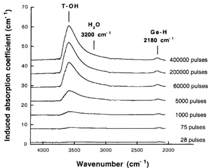
Figure 3.6.11: IR spectra of defect concentrations depending on the pulse rate. The UV exposure leads to the generation of different H-bearings, namely Ge-H ( $2180\text{ cm}^{-1}$ ),  $\text{H}_2\text{O}$  ( $3200\text{ cm}^{-1}$ ?) and T-OH (approx.  $3600\text{ cm}^{-1}$ , T = Si or Ge) [51].
