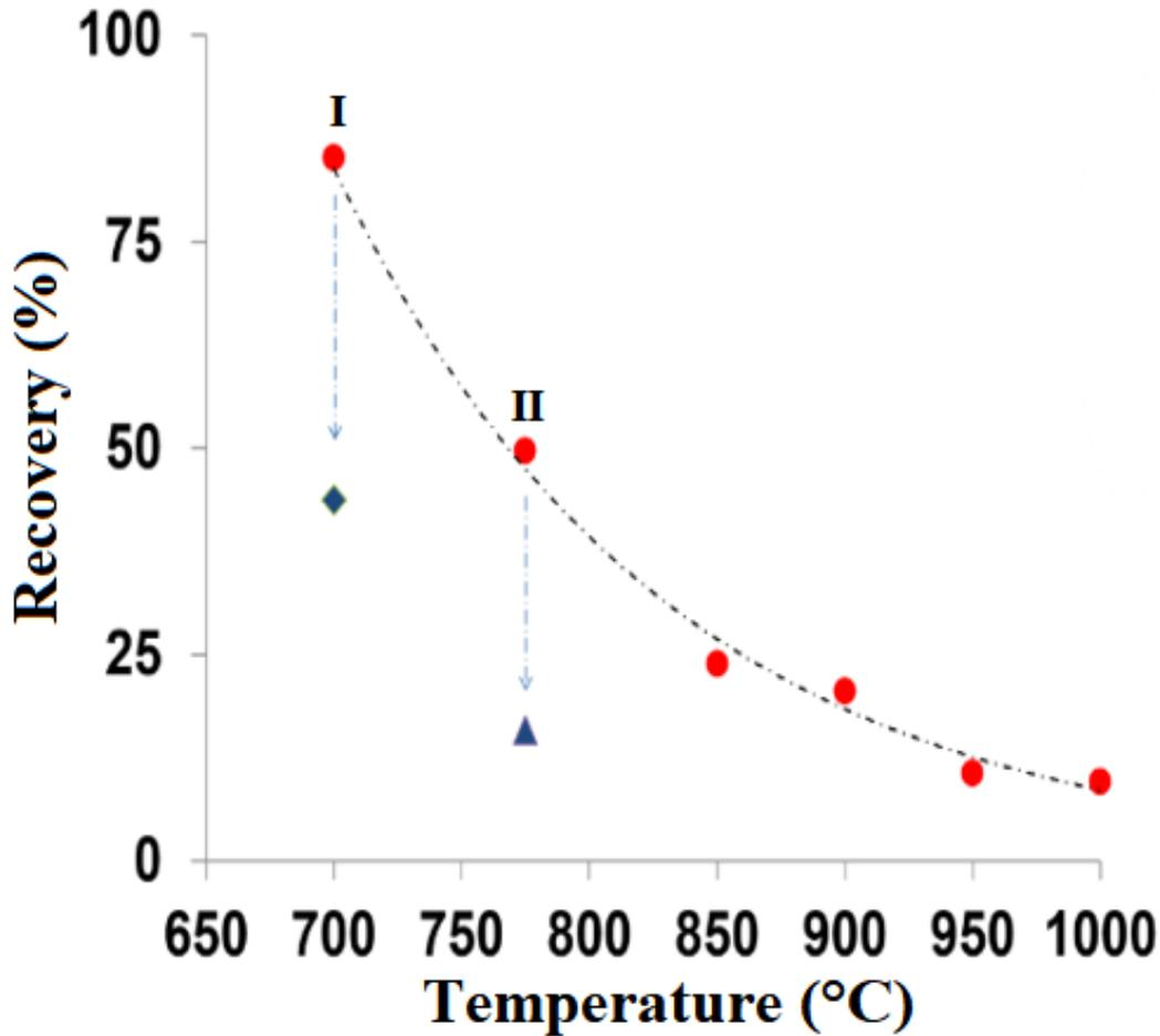
Figure 4.3.2: Recovery as a function of annealing temperature [28]
