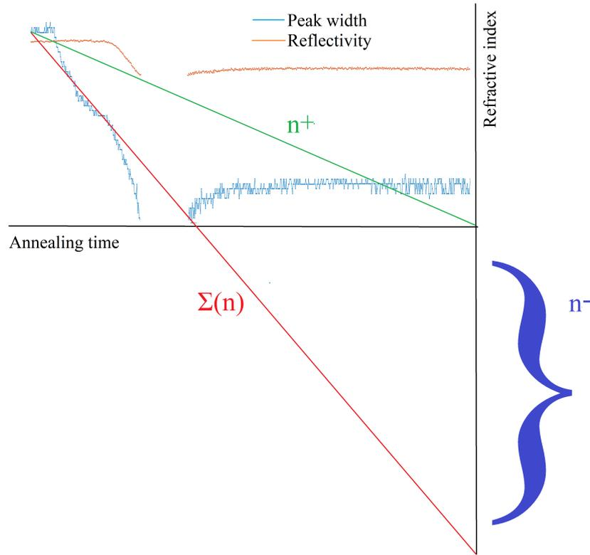
Figure 4.3.7: Schematic representation of the competing-gratings model.
