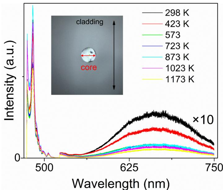
Figure 5.2.7: Raman and emission spectrum of a pristine PS1250/1500 fiber studied between ambient and 900 °C upon excitation by 473 nm light in the core. The inset shows the microscope image of the fiber cross-section with a core and the surrounding cladding [97].
