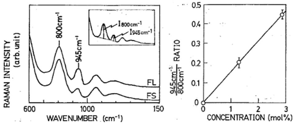
Figure 3.6.3: Left: Section of a Raman spectra for fluorine doped glasses with different fluorine concentrations (FL= 2.8 mole% and FS= 1.3 mole%). The peak around  $945\text{ cm}^{-1}$  is related to the Si-F bond. Right: Correlation of the intensity ratio to the doping concentration [91].
