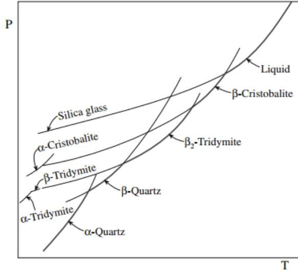
Figure 1.3.2: Phasediagram of SiO<sub>2</sub>. At atmospheric pressure, different polymorphs are possible depending on the temperature [32].
