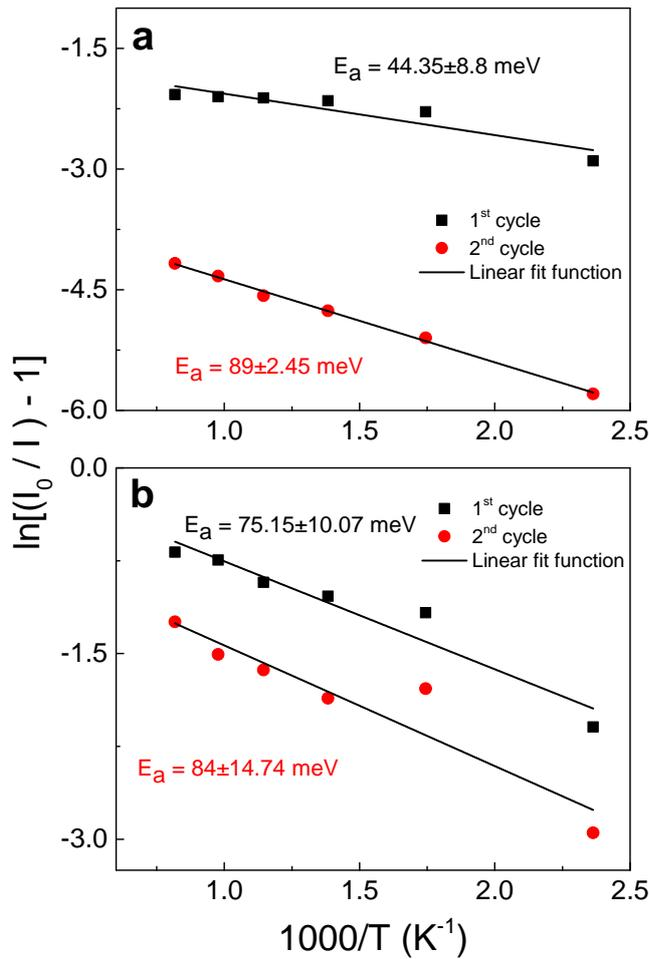
Figure 5.3.8: Arrhenius plot of PL intensity between ambient and 950 °C for (a) grating in SMF28 fiber and (b) SMF28 pristine fiber [97].
