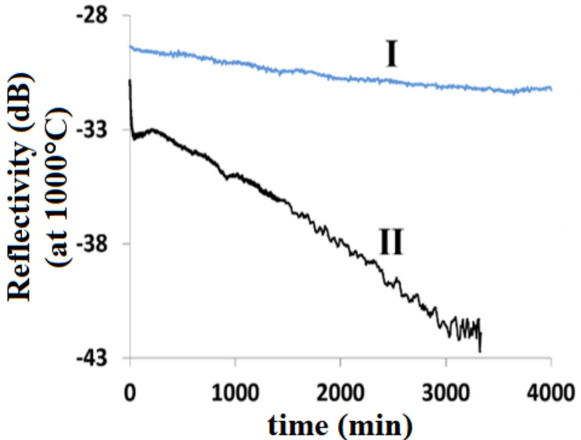
Figure 4.3.3: Recovery stability as a function of annealing time during regeneration, the plots labelled "I" and "II" correspond to the data points in figure 4.3.2 [28].
