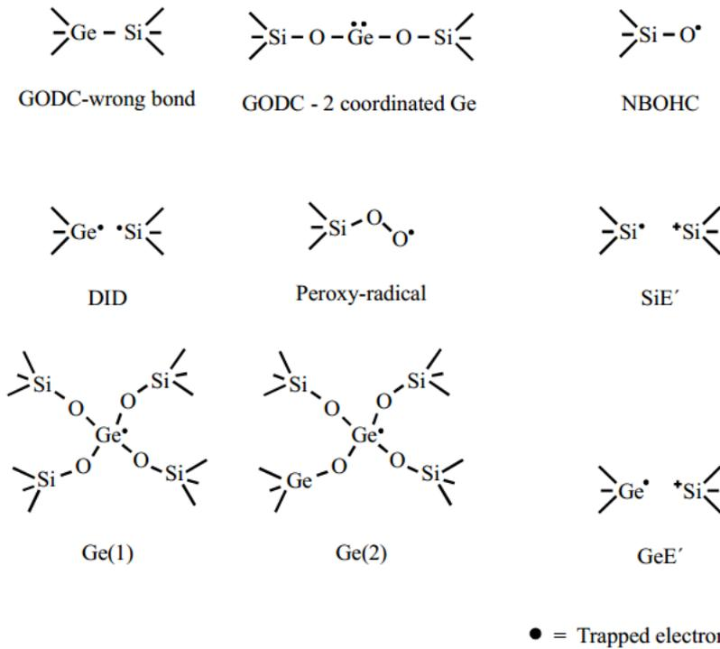
Figure 1.4.1: Different types of defects which are related to the photosensitivity in optical glass fibers [29].
