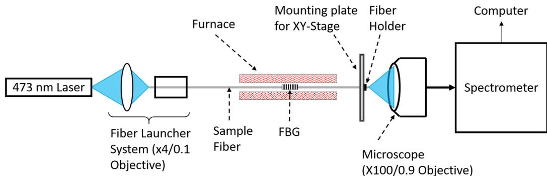
Figure 5.1.1: *In situ* measurement setup consisting a 473 nm diode pumped solid state (DPSS) laser, a Thorlabs fiber launcher, a high temperature furnace, a confocal microscope and the Horiba spectrometer with the CCD camera.
