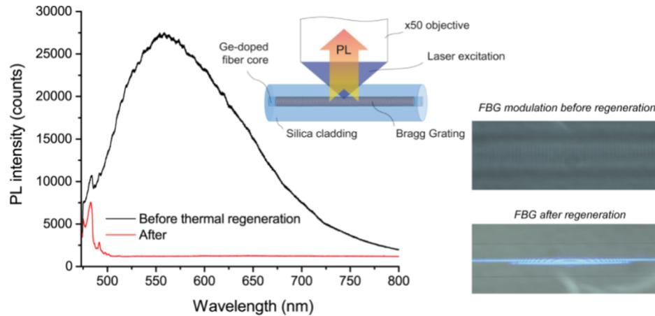
Figure 5.3.3: Left: Decrease of the PL around 550 nm after thermal regeneration. Top: Measurement setup for the PL measurements. Right: Light scattering out of the fiber before and after regeneration [28].
