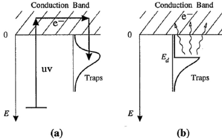
Figure 2.2.2: Illustration of the trapping (a) and depopulation (b) process of electrons. The traps can be emptied due to the demarcation energy  $E_d$ . Thermal depopulation is proposed for shallow traps ( $E < E_D$ ) while deeper traps ( $E > E_D$ ) remain populated [10].
