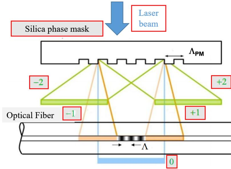
Figure 2.1.2: Schematic of a phase mask approach. The numbers within the red box in the figure represent the diffraction orders. The symbols  $\Lambda$  and  $\Lambda_{PM}$  are the period of the grating and that of the silica phase mask, respectively. Figure is adapted from the reference [60].
