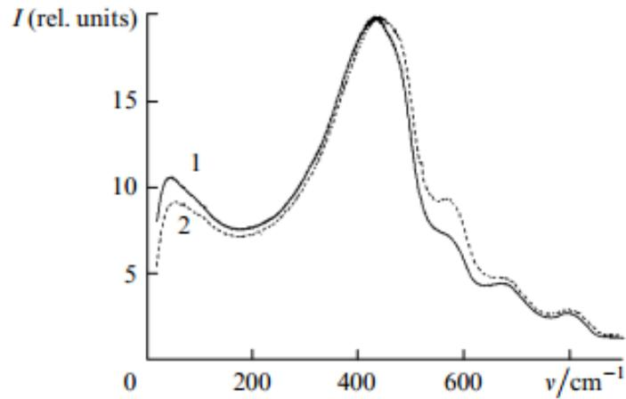
Figure 3.6.4: Densification of highly doped optical fibers after irradiation (2) with the second harmonic of an Ar ion laser. With increasing lasershots, the intensity of the D1 and D2 defects in the Raman spectrum increases [93].
