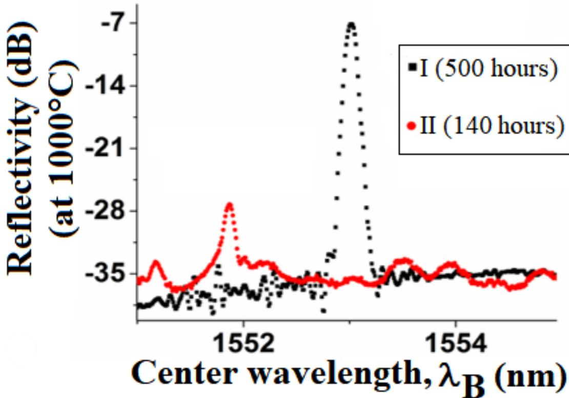
Figure 4.3.4: Long-term stability test of grating reflectivity [28]. A higher signal to noise ratio of RFBG (regeneration performed at 700 °C, black curve compared to regeneration performed at 775 °C, red curve) is obtained from the post-thermal stability tests conducted at 1000 °C.
