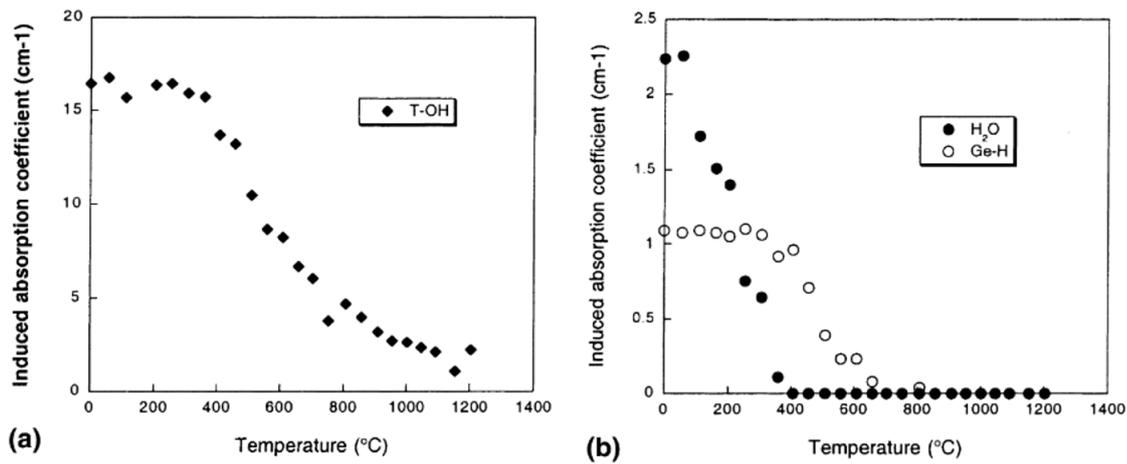
Figure 3.6.13: Temperature stability of UV-induced H-bearings in hydrogen loaded fibers. (a): Temperature stability of hydroxyl compounds (Si-OH and Ge-OH, respectively). Hydroxyl related compounds are stable until 400°C and subsequently decrease with increasing temperature. (b): Temperature stability of molecular water (H<sub>2</sub>O) and germanium hydride (GeH). Molecular water shows a rapid initial decay with increasing temperature while GeH is stable up to approx 400°C [51].
