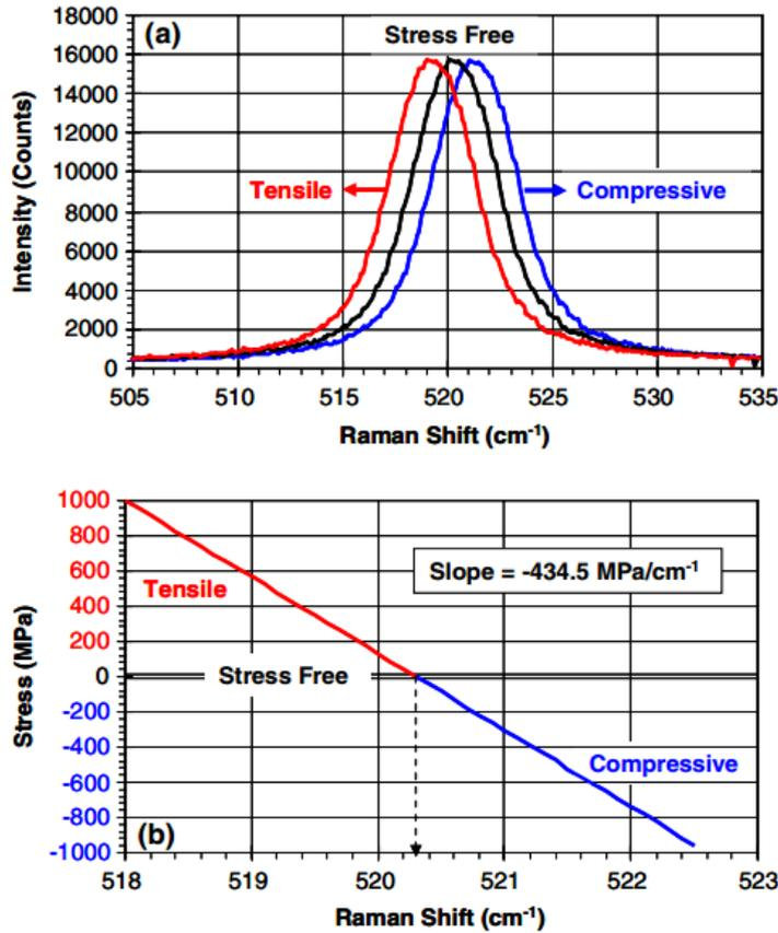
Figure 3.4.4: Stress measurements in a silicon sample. A shift in the Si-Si Raman peak position represents tensile (negative shift) or compressive (positive shift) stress [89].
