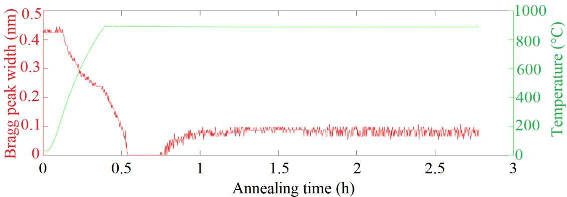
Figure 4.2.2: Peak width (red) as function of annealing time and temperature.
