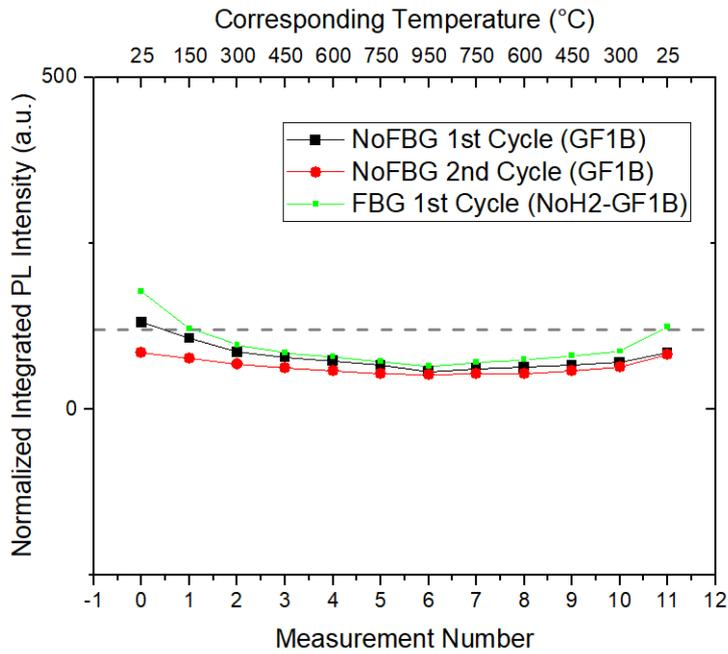
Figure 5.3.6: A non-hydrogen loaded FBG in a GF1B fiber (green line) shows a small amount of PL (compared to bare fibers). With increasing temperature the PL of the FBG decays and is fully erased around 150 °C.
