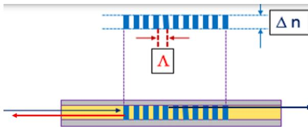
Figure 2.1.1: Illustration of a fiber Bragg grating. An incoming lightsource (e.g. the interrogator laser) will be reflected around the Bragg wavelength while every other wavelength is transmitted.
