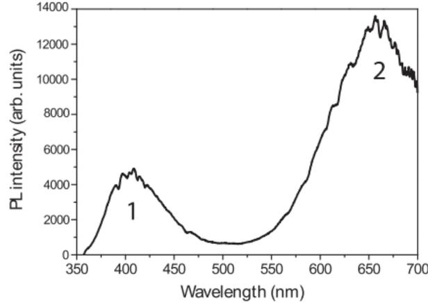
Figure 5.3.1: PL of a Ge-doped fiber excited with 355 nm. Two PL peaks are observable after excitation. (1) at  $\approx 400$  nm belongs to ODC and (2) at  $\approx 650$  nm belongs to NBOHC [1].
