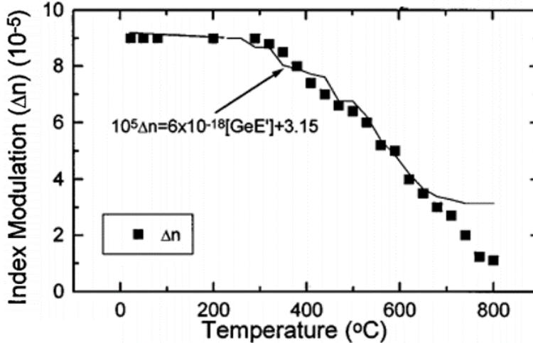
Figure 2.2.1: Thermal decay of the GeE' defect (solid line) and index modulation (dots), respectively [48]. With increasing temperature, the GeE' defects as well as the index modulation decreases.
