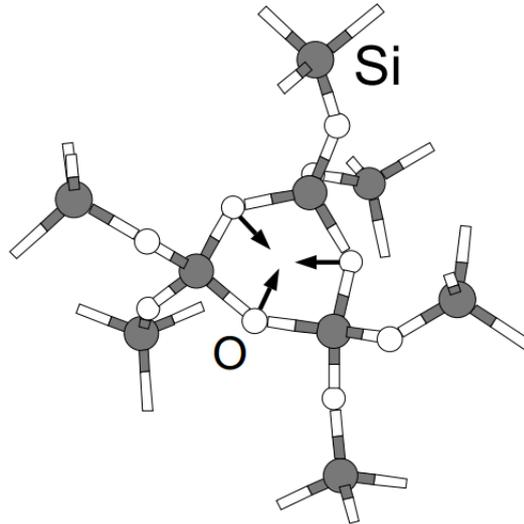
Figure 3.4.3: 3-fold ring in vitreous silica network. The black arrows illustrate the breathing motion of the 3-fold silica ring [88].
