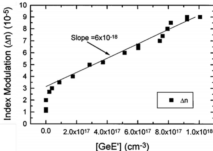
Figure 1.4.3: Correlation between the amount of GeE' centers and the change of the RI during UV inscription (Laser fluence of 300 J/cm<sup>2</sup>) [48].
