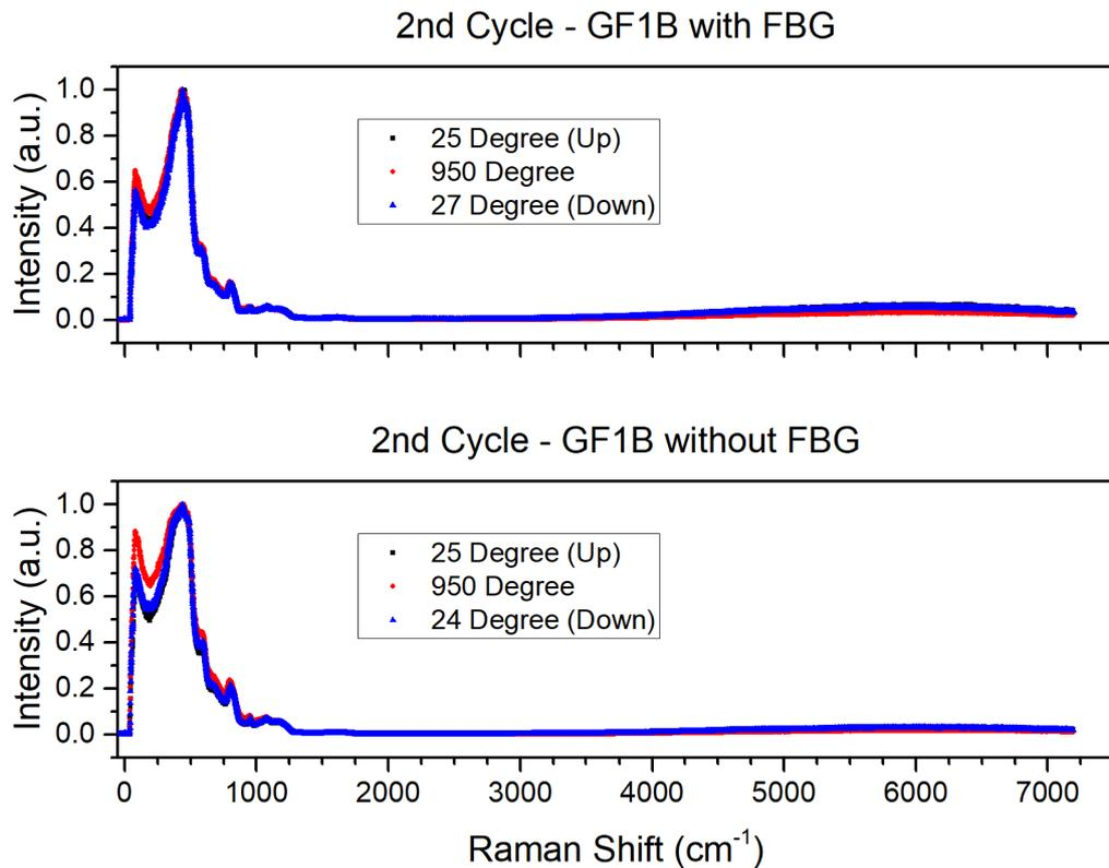
Figure 5.2.11: 2<sup>nd</sup> regeneration cycle of the GF1B fiber. The top graph shows the 2<sup>nd</sup> cycle of the fiber containing a FBG. Here, photoluminescence was not observable anymore. For comparison, the bottom graph shows the 2nd regeneration cycle of the bare fiber. The colors are the same for both graphs and indicate room temperature at beginning (black), regeneration temperature (red) and room temperature at the end (blue).
