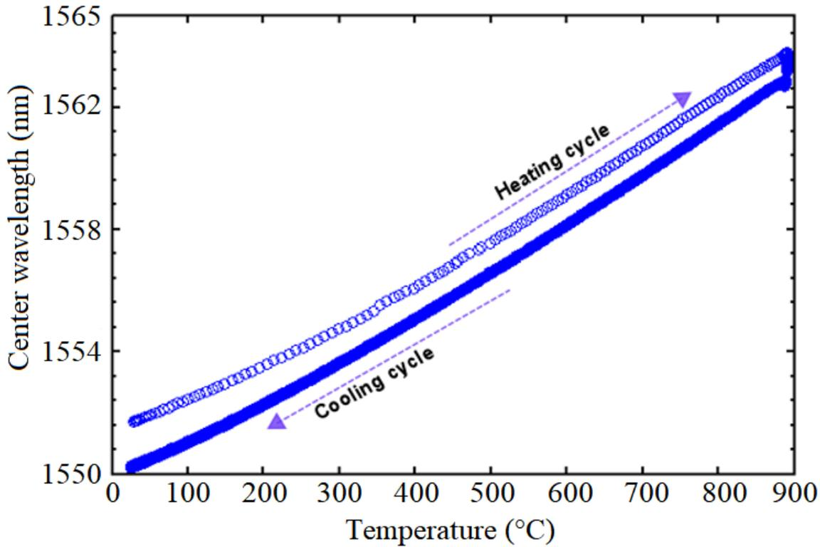
Figure 4.3.1: Central wavelength as function of temperature.
