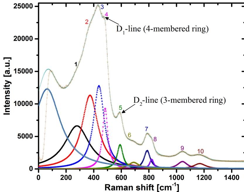
Figure 5.2.2: Raman scattering spectrum at ambient temperature with deconvolution of Lorentzian lineshape (peaks correspond to the identifications in iXFiber sample presented in Table 5.2.3) [97, 98].
