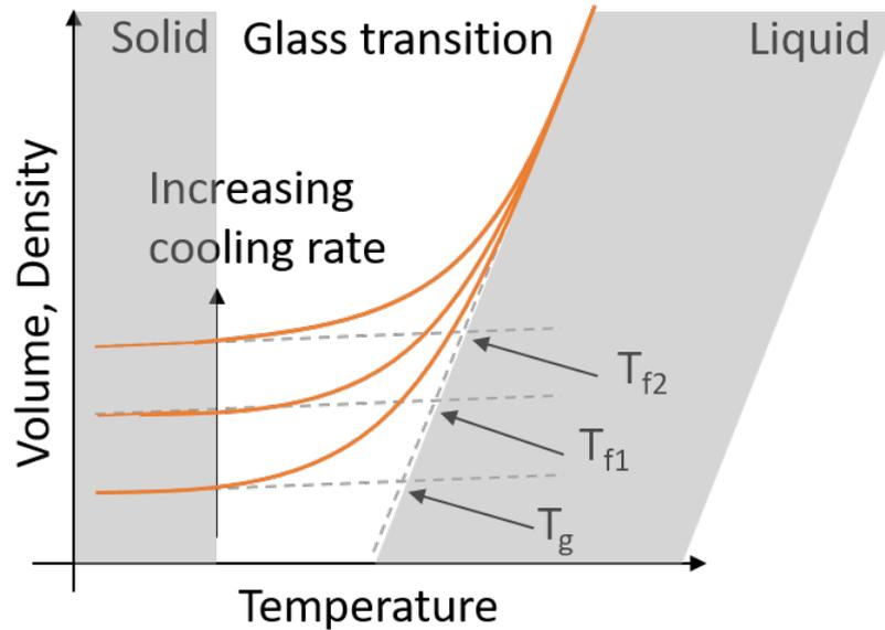
Figure 1.3.4: Dependency of the glass parameters on the temperature during the cooling process. As the temperature decreases the glass goes from its liquid state to the glassy state. The extrapolated lines of both states indicate the glass transition temperature for the minimal cooling rate and the fictive temperature for higher cooling rates [23].
