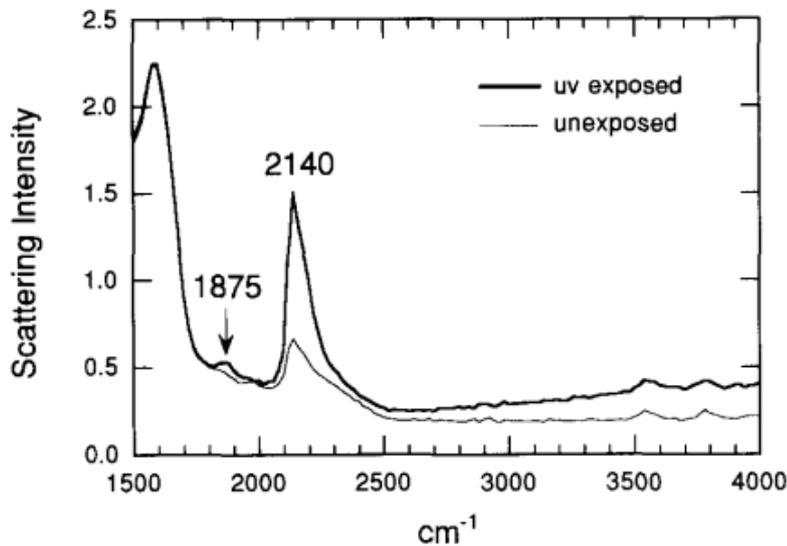
Figure 3.6.9: Raman spectra of a hydrogen loaded fiber before and after UV exposure (x-axis displays the Raman shift). After UV exposure, two new peaks are observable. The peak at  $2140 \text{ cm}^{-1}$  is assigned to  $\text{GeH}_2$  whereas the peak at  $1875 \text{ cm}^{-1}$  is not yet assigned to any vibrational mode [56].
