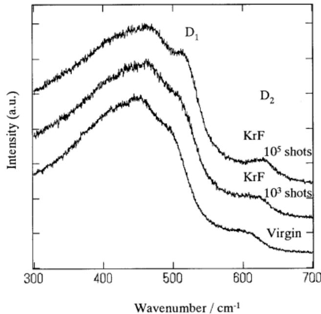
Figure 3.6.5: Densification of glass disks after irradiation with a KrF laser. With increasing lasershots, the intensity of the D1 and D2 defects in the Raman spectrum increases [94].
