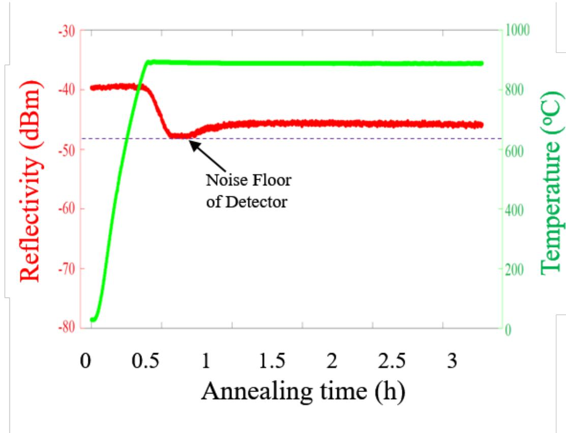
Figure 4.2.1: Reflectivity (red) as function of annealing time and temperature [a semi-log graph]. The time at which the reflectivity reaches to its minimum value corresponds to minimum detectable reflectivity or the detector’s noise floor which also means that it is not the the absolute FBG reflectivity that is important but it is rather the signal to noise ratio with which the Bragg signal is measured that matters.
