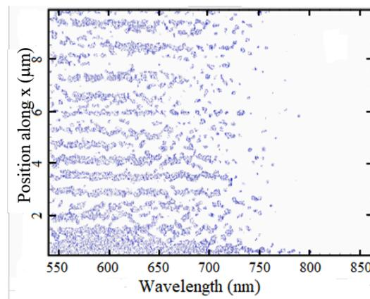
Figure 5.3.2: Spatial intensity PL map of the 650 nm peak. One can see the spatial periodicity of the NBOHC which equals the grating period of  $\Lambda \approx 0.5 \mu\text{m}$  [1].
