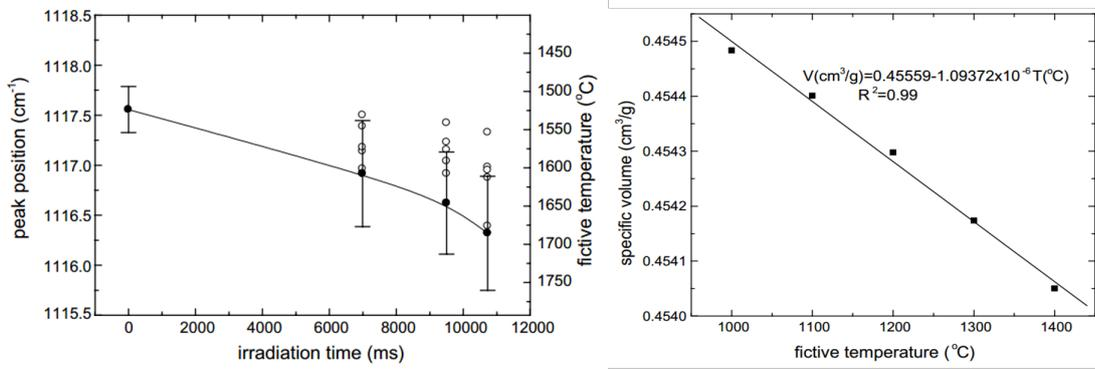
Figure 3.6.6: Left: Increase of the fictive temperature and shift of the IR peak with increasing laser pulses, respectively. Right: Correlation between the specific volume with fictive temperature [52].
