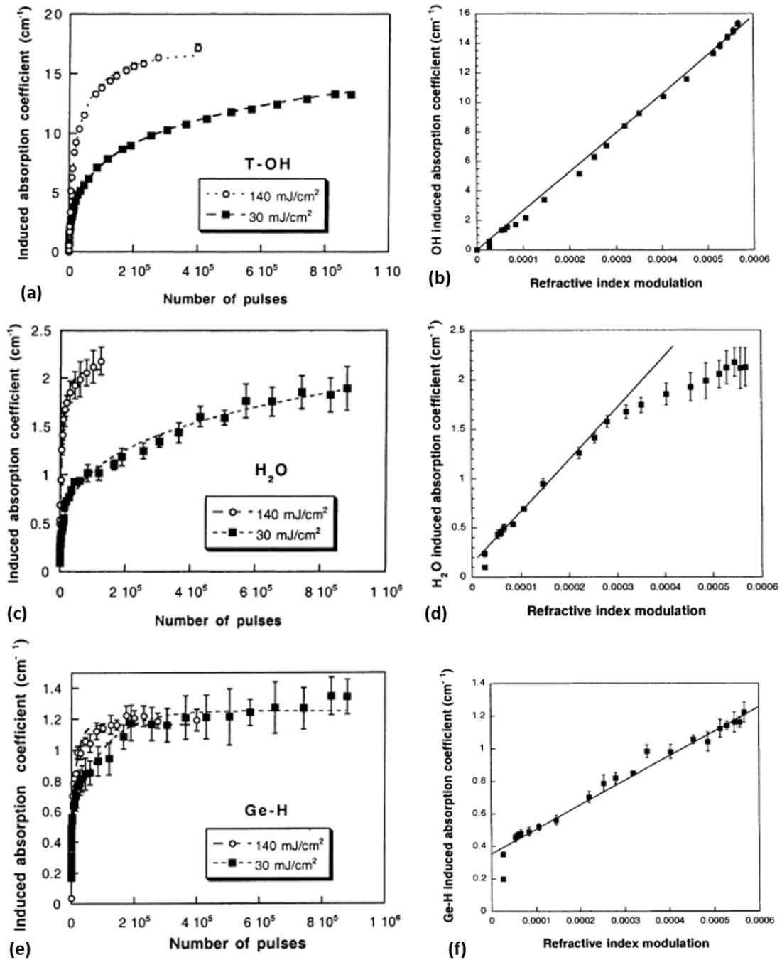
Figure 3.6.12: Left: IR peak intensity of H-bearing concentration depending on the number of laser pulses. Right: Increase of the refractive index modulation with increasing H-bearing concentration. Here, the data from the 140 mJ/cm<sup>2</sup> was used [51].
