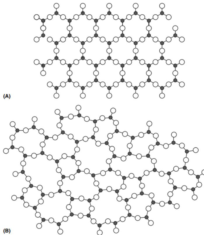
Figure 1.3.1: 2-dimensional structure of crystalline silica **(A)** and amorphous silica **(B)**. White circles represent silicon  $4+$  ions whereas black dots represent oxygen  $2-$  ions [32].
