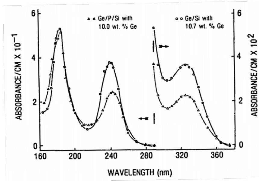
Figure 1.4.2: Different UV absorption bands in germania doped silica (10.7 wt.% Ge, circles) and germanium phosphosilicate (10 wt.% Ge, triangles) [46].
