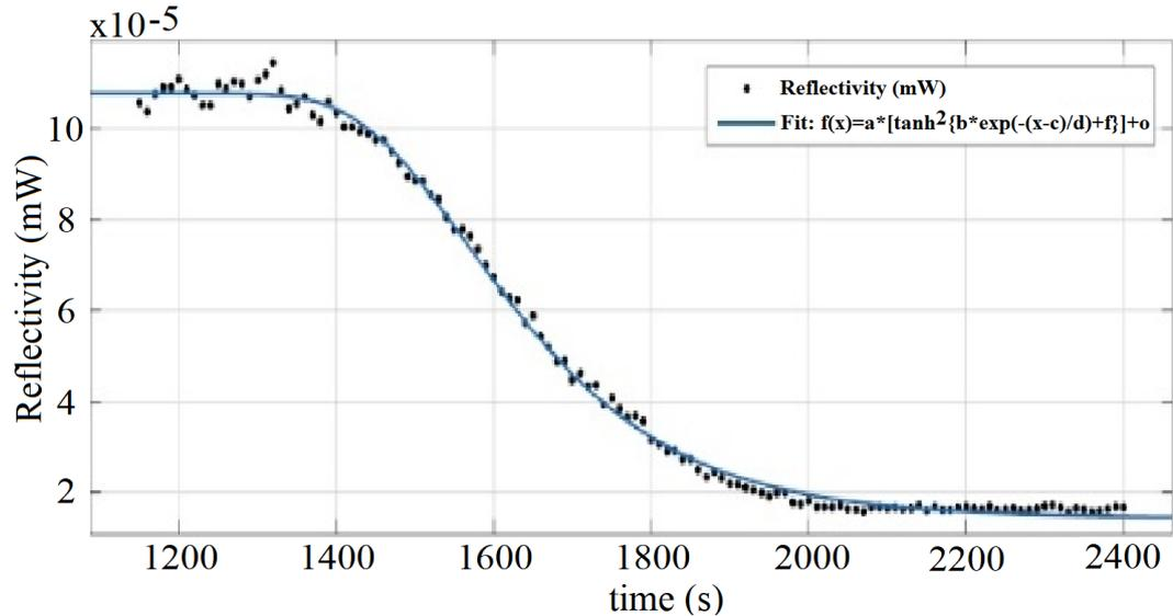
Figure 4.2.3: The  $\tanh^2$  behavior of the reflectivity as function of time, showing the initial decay of FBG with the data set cut at  $t = 2400$  s as it hits the noise floor before the regeneration (Here, the reflectivity in y-axis is transformed into a linear scale from figure 4.2.1).
