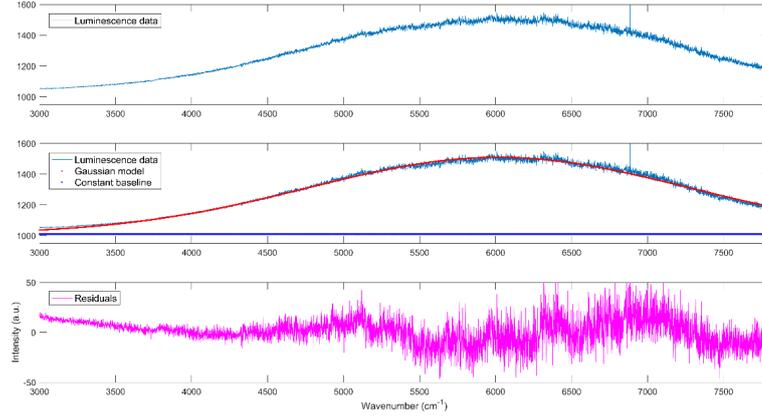
Figure 5.3.7: Spectral shape of the emission band (upper panel) fitted to a single Gaussian curve (middle panel) showing the fit residual (lower panel) [97].
