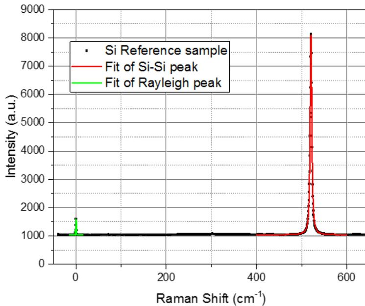
Figure 5.2.1: Calibrated Si-Raman spectrum:  $520.7\ \text{cm}^{-1}$  band is assigned to the Si-Si bond and  $0\ \text{cm}^{-1}$  to the suppressed Rayleigh scattering.
