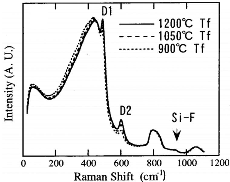
Figure 3.6.8: Raman spectra of fluorine doped glasses with increasing fictive temperature. Densification can be seen by the increase of the D1 and D2 defect as well by a smaller main peak [40].
