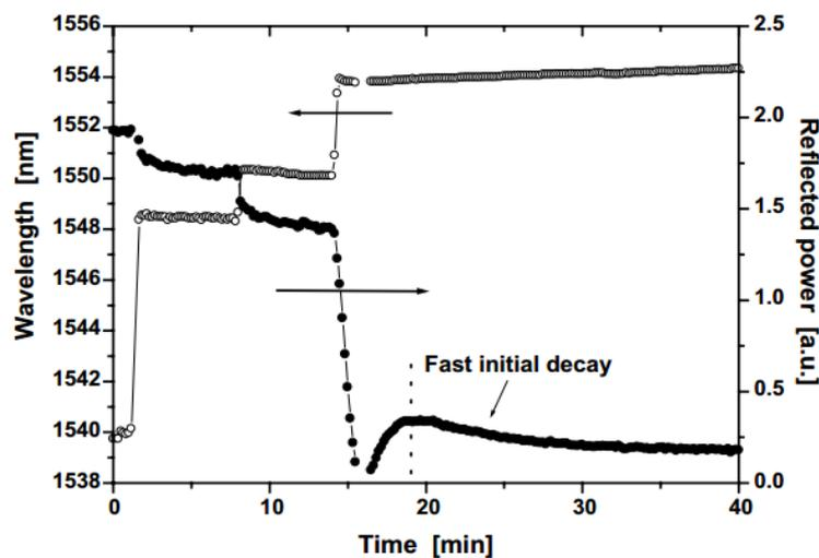
Figure 2.2.4: Regeneration behavior of a  $\text{H}_2$ -loaded SMF28 fiber observed by Fokine after heating from room temperature ( $\lambda_B \approx 1540$  nm) to  $600^\circ\text{C}$  ( $\lambda_B \approx 1548$  nm),  $700^\circ\text{C}$  ( $\lambda_B \approx 1550$  nm), and  $1000^\circ\text{C}$  ( $\lambda_B \approx 1554$  nm). The regeneration occurs after approx. 15 minutes where the reflected power is below the noise level and afterwards arises again to its maximum after 18 minutes [8].
