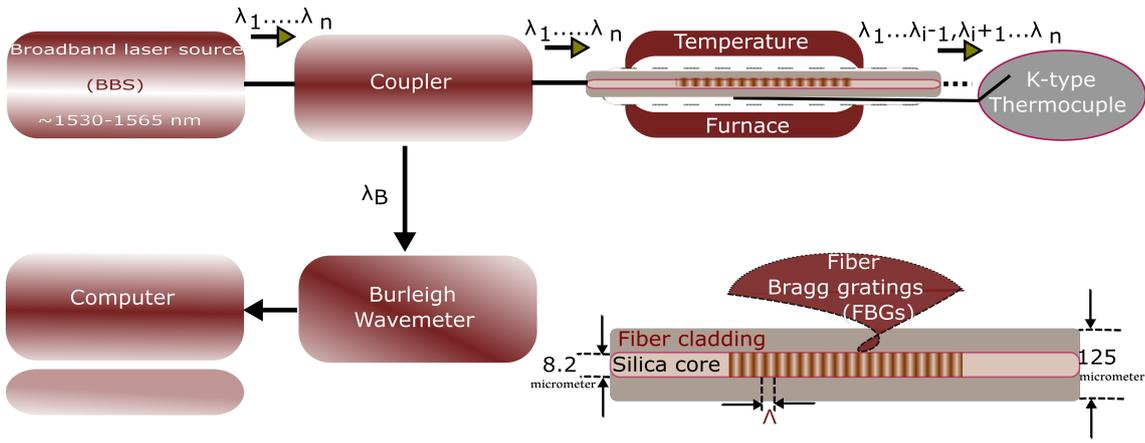
Figure 4.1.1: Setup used to measure fiber Bragg grating reflectivity.
