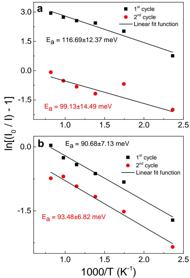
Figure 5.3.9: Arrhenius plot of PL intensity between ambient and 950 °C (repeated cycles) for (a) grating in GF1B fiber and (b) GF1B pristine fiber [97].
