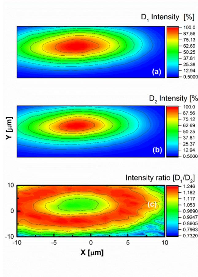
Figure 5.2.5: Raman intensity map across a fiber end of a)D1 band, (b)D2 band and (c)D1 and D2 ratio. The intensities of the two components are obtained from spectral deconvolution [98].
