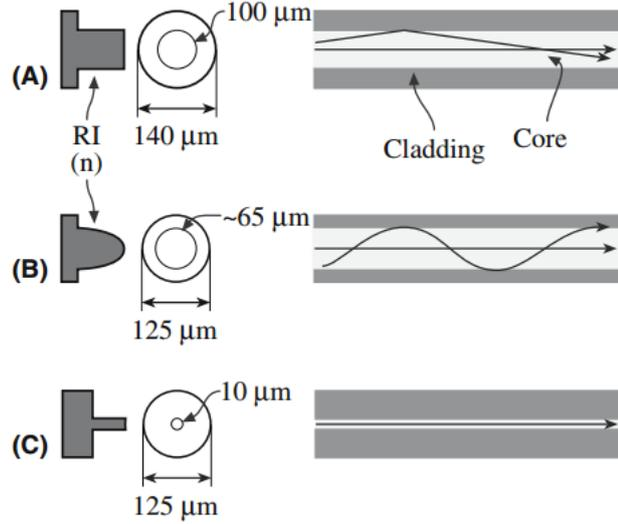
Figure 1.2.1: Different types of TIR in glass fibers, their typical RI distribution and dimensions. **(A)**: Multi mode (MM) step index fiber, **(B)**: Gradient index (GRIN) fiber, **(C)**: Single mode (SM) fiber [32].
