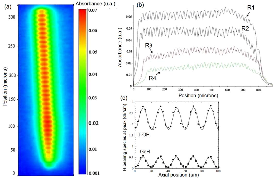
Figure 3.6.14: Spatially resolved FTIR measurements of H-bearing generation in hydrogen loaded fiber preforms. Plot (a) shows the 2D distribution of all H-bearings combined. Plot (b) shows the intensity cross-section of plot (a) for different inscription parameters. Plot (c) shows the spatially and compoundend resolved intensity of the H-bearings [11].
