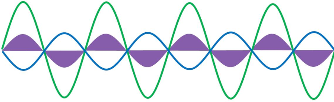
Figure 4.3.6: Schematic illustration of antiphase gratings. This is to note here that in reality the periodic gratings would show only one half of the index modulation because of the UV writing procedure.
