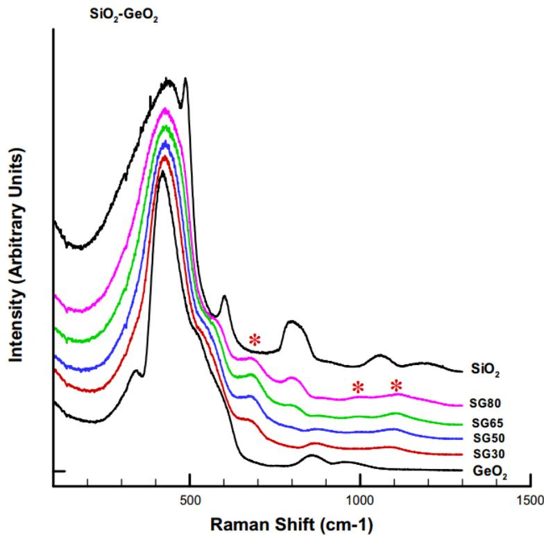
Figure 3.6.1: Raman spectra for silica, germania and mixed glasses. The numbers stand for the content of silica in percent and the red stars indicate the Ge-O-Si bonds which are not present in pure silica and germania, respectively [27].
