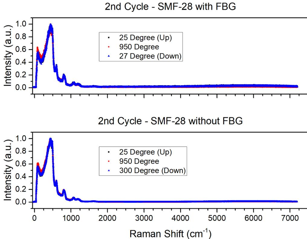
Figure 5.2.9: 2<sup>nd</sup> regeneration cycle of the SMF-28 fiber. The upper graph displays the signal for the fiber containing a FBG. Here, the black curve is the initial spectrum at room temperature, the red curve is the spectrum at the regeneration temperature (950 °C) and the blue curve is the final spectrum back at room temperature. The bottom graph shows the regeneration of a bare fiber without FBG. The curve colors and temperatures are the same as for the top graph.
