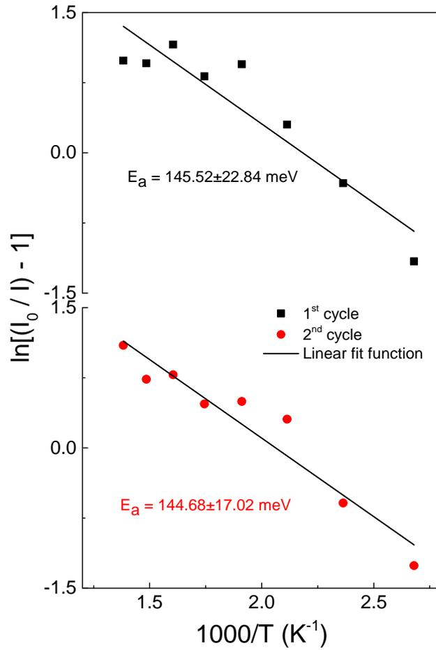
Figure 5.3.10: Arrhenius plot of PL intensity between ambient and 950 °C (repeated cycles) for PS1250/1500 pristine fiber [97].
