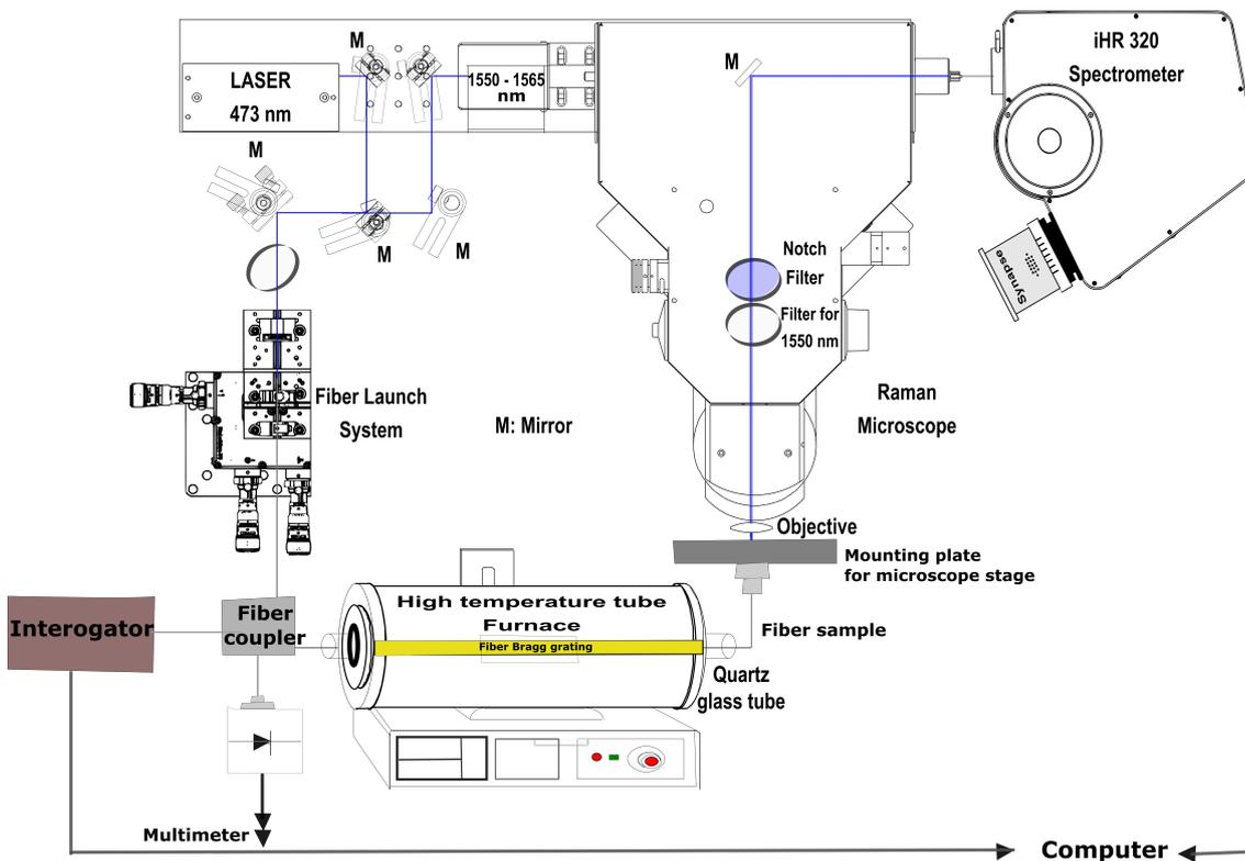
Figure 6.0.1: Improved measurement setup. A 90/10 fiber coupler allows simultaneous measurements of the Raman signal and the laser power. Additionally, the reflected power of the FBG and the Bragg wavelength during the Raman measurements can be measured by an interrogator system.
