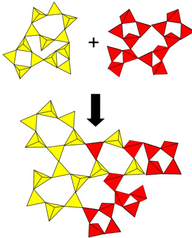
Figure 1.3.3: Formation of mixed rings out of silica (yellow) and germania (red). As the bottom picture illustrates, 6-membered mixed rings are formed, while losing 3- and 4-membered rings from silica and germania, respectively [27]. Note that this is for illustration and 4-membered rings are very unstable hence they are not very present in the glass network [39].
