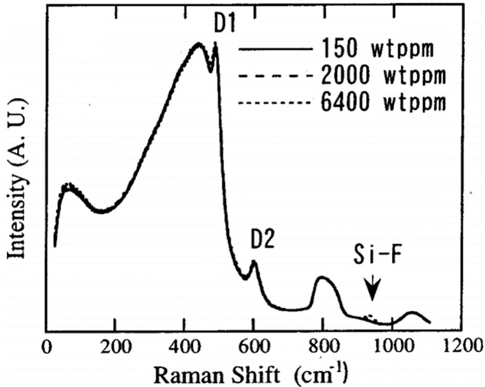
Figure 3.6.2: Raman spectra for fluorine doped glasses with different fluorine concentrations. The peak around  $945\text{ cm}^{-1}$  is related to the Si-F bond [40].
