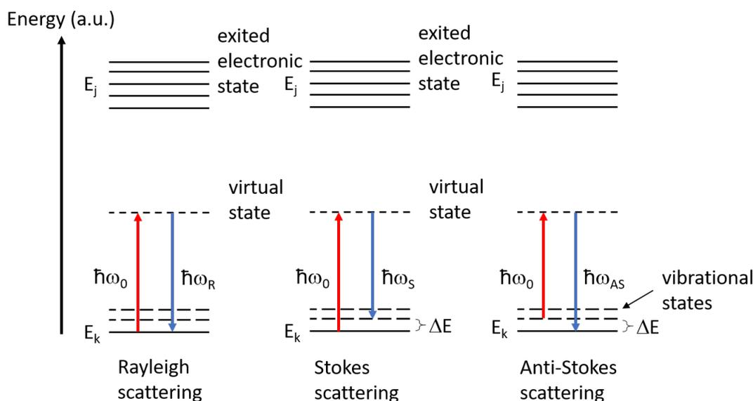
Figure 3.4.1: Different types of scattering. Elastic scattering ( $\Delta E = 0$ ) is the most common process. The inelastic scattering is less likely than Rayleigh due to the dependence on vibrational states (factor  $\approx 10^8$  [84]).
