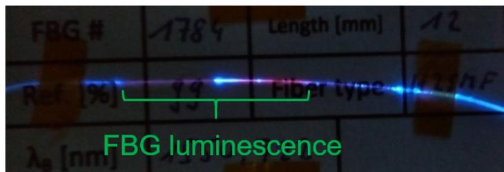
Figure 5.2.6: A strong luminescence of about 15 mm length can be observed at the location of the FBG. Additional but less intense red PL can be observed all over the uncoated area [97].
