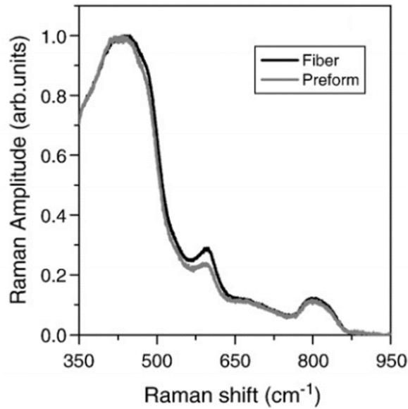
Figure 3.6.7: Raman spectra for a fiber preform (grey line) and the final fiber (black line). Densification can be seen by the increase of the D1 and D2 defect as well by a smaller main peak [22].
