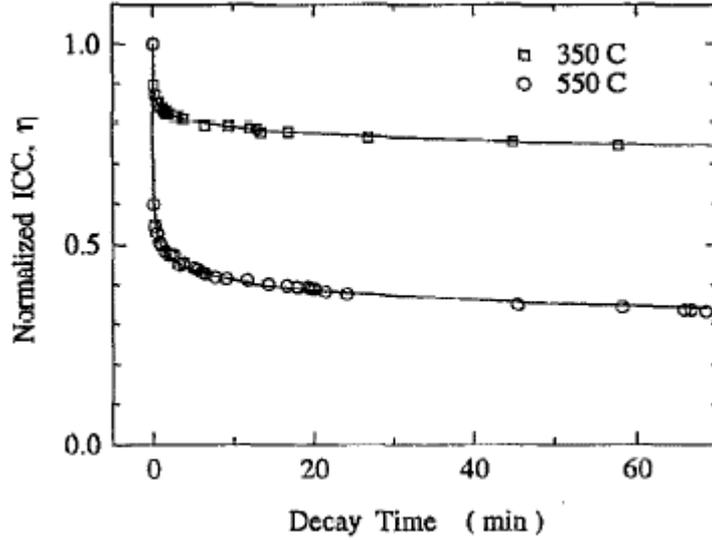
Figure 2.2.3: Experimental (circles and squares) decay experiment from Erdogan et al. at constant temperatures with applied power law model (solid line). Because of the power law model, the gratings show a stronger decay at the beginning and less decay after longer dwell time [10].
