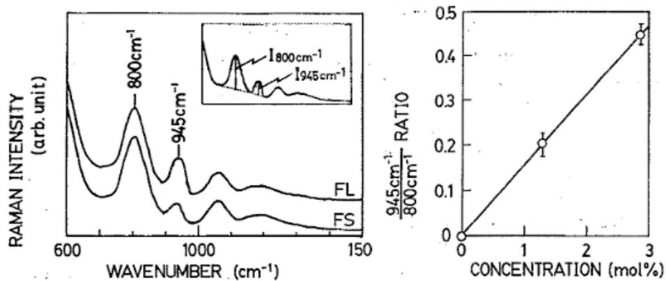
Figure 5.2.13: Left: Section of a Raman spectra for fluorine doped glasses with different fluorine concentrations (FL= 2.8 mole% and FS= 1.3 mole%). The peak around  $945\text{ cm}^{-1}$  is related to the Si-F bond. Right: Correlation of the intensity ratio to the doping concentration [91].
