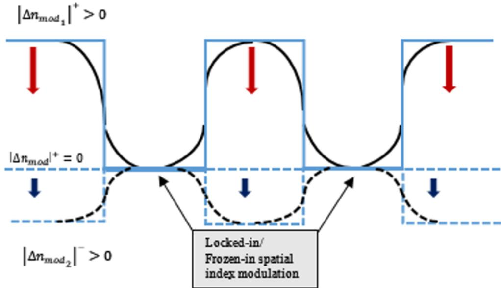
Figure 4.3.8: Schematic illustration of the competing gratings.
