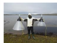
Bubble traps for ebullition flux
