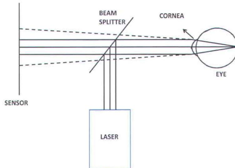
Figure 14. Modified homodyne interferometry to measure the fundus pulsations.
