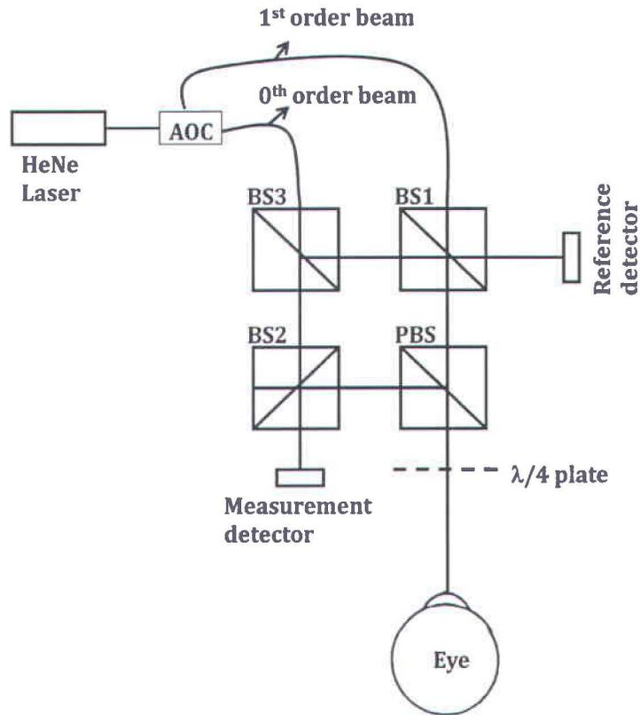
Figure 16. Layout of the heterodyne interferometer.
