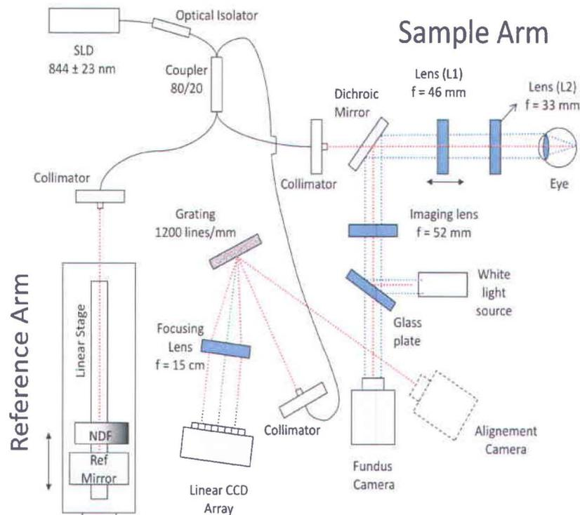
Figure 21. Schematic of the designed system based on Fourier domain low coherence interferometry to measure the ocular dynamics in a rat
