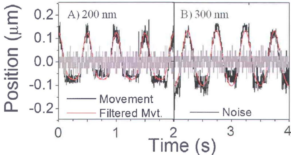
Figure 24. Small movements measured with FD-LCI system.
