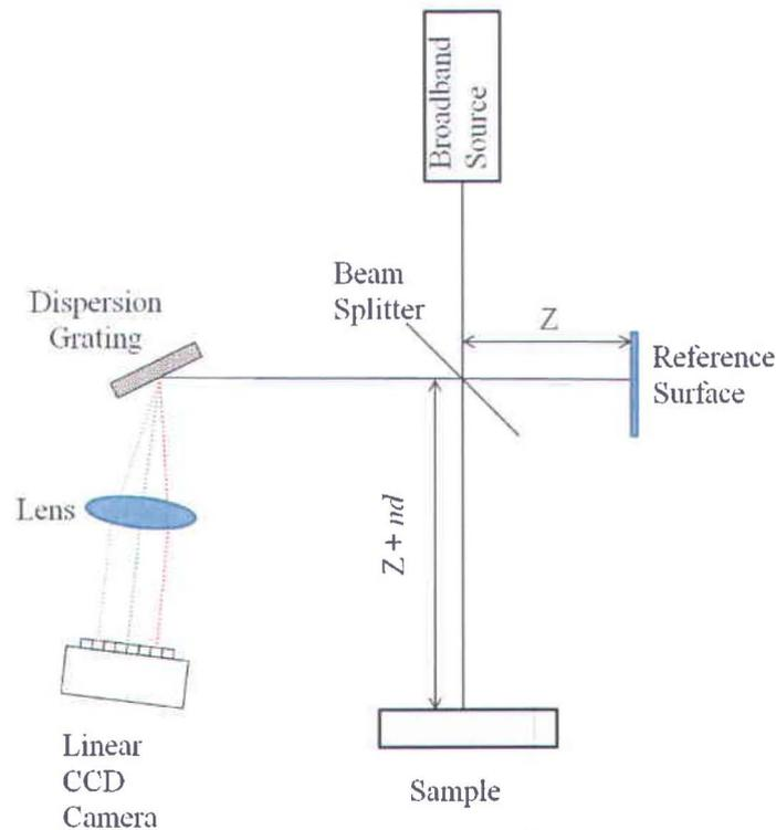
Figure 20. Schematic of the Fourier (Spectral) domain low-coherence interferometric system.
