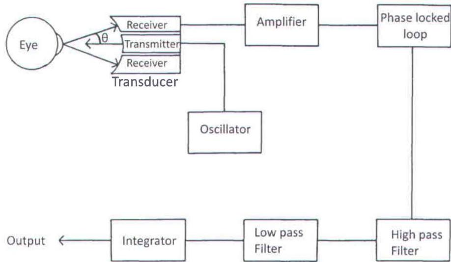
Figure 11. Schematic of the Ultrasound Transducer system to measure corneal displacement.
