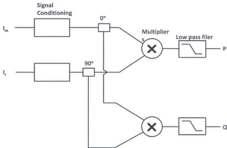
Figure 17. Demodulation technique used in heterodyne interferometer system.
