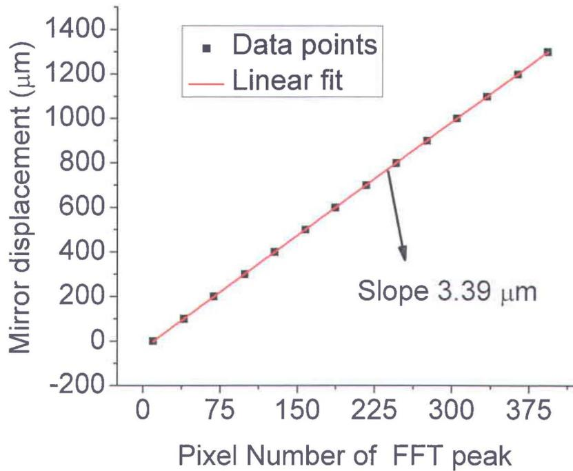
Figure 22. System calibration curve.
