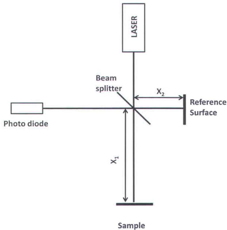
Figure 13. Schematic of the homodyne Michelson interferometer.
