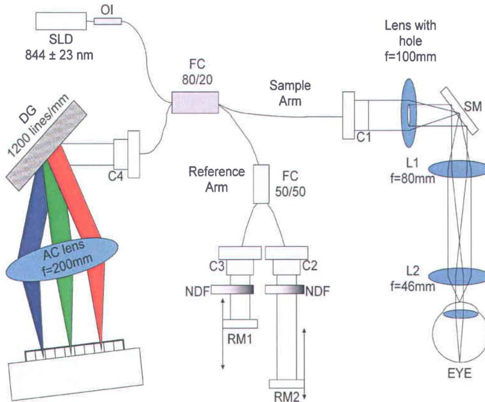
**Figure 28. Schematic of the optical system developed to measure the corneal and retinal movements simultaneously.**
