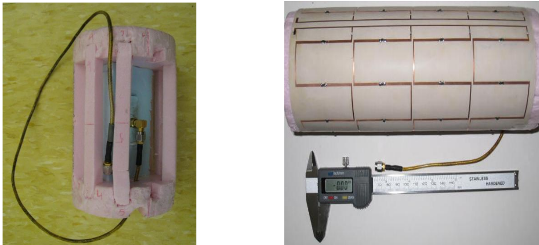
Fig. 5-12 Photo of fabricated switched-beam reconfigurable antenna.
