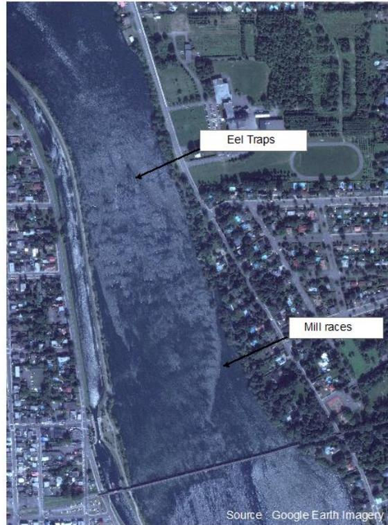
**Figure 1-11** Man made structures in the Saint-Jean-sur-Richelieu bed-rock shoal area.
