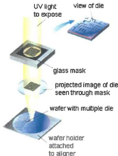
**Figure 2.1** Schematics of optical lithography process. UV light passes through the glass mask plate (reticle) and projects the image onto the silicon wafer covered with thin photo-sensitive film ([www.ncnanotechnology.com/public/features/TNLC.asp](http://www.ncnanotechnology.com/public/features/TNLC.asp))
