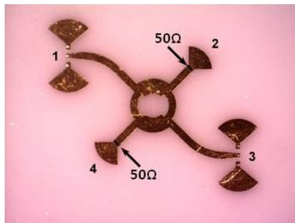
Figure 2.2 - Microphotograph of the branch-line coupler
