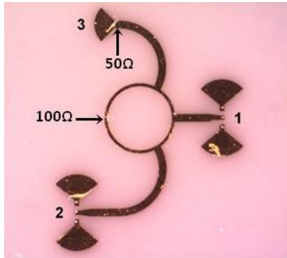
Figure 2.10 - Microphotograph of the Wilkinson power divider/combiner.
