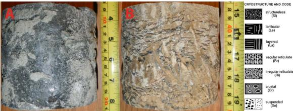
Fig. 1. A) Silty ice-rich permafrost sample with a suspended cryostrucure, B) coarse sand permafrost sample with a lenticular cryostructure base on the north-american cryostructure classification proposed by Murton and French (1994).
