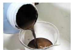
Fig. 1. The Repairing Material (Asphalt Emulsion).
