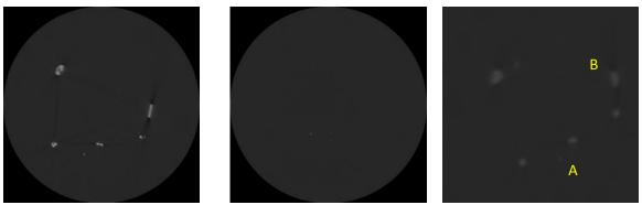
**Fig. 1.** Two CT scans of the same set of gold grains embedded in quartz and epoxy, and surrounded by quartz powder. Left image field of view is 10 mm; center is 50 mm, and the right image is a zoom-in of the center image.
