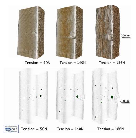
**Fig. 3.** In situ tensile testing of a steel laser weld system, at three levels of tension. Cracking initialized from a rough surface feature, as well as elongation of interior voids, are visible as the load is increased. (In collaboration with Sandia National Laboratory)
