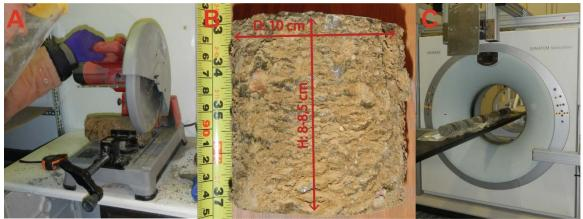
**Fig. 2.** A) Permafrost cores are cut with a concrete saw at a temperature of -18°C B) Final dimension of a sample.C) .The Siemens Somatom 64TM scanner allowed a fast data acquisition, thus keeping the frozen state of the samples.
