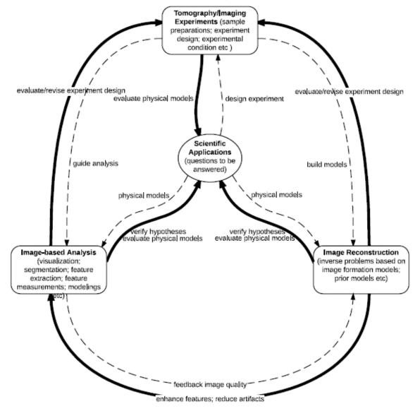
**Fig. 1.** Tomography experiment workflow. From each of three steps around scientific applications, the information of the system in study is obtained at certain level. Evaluations of such information at each step can help to revise or improve the experiment design and data analysis, and verify the hypotheses on the system.
