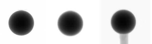
**Fig. 1.** Real projection of an AI sphere taken at HECTOR (right), simulated projection without (left) and with (middle) spot correction.
