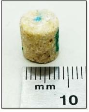
**Fig. 2.** Standard mini-plug sample for microCT and SEM studies.
