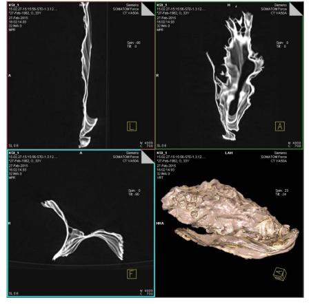
Figure 4: Three orthogonal cross sections and a volume rendering of the reconstructed oyster sample.
