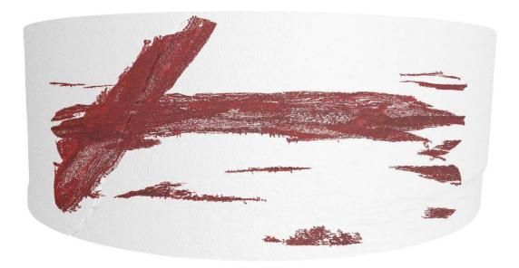
Fig. 2. Transparent 3D view of the L300 CT data. Cracks are segmented (red colour).
