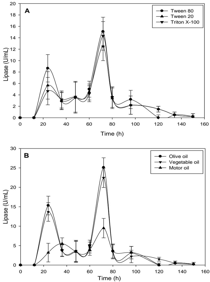
**Figure 6.1** Lipase activity in the presence of surfactants and oils as inducers (A: in the presence of surfactants, B: in the presence of oils)
