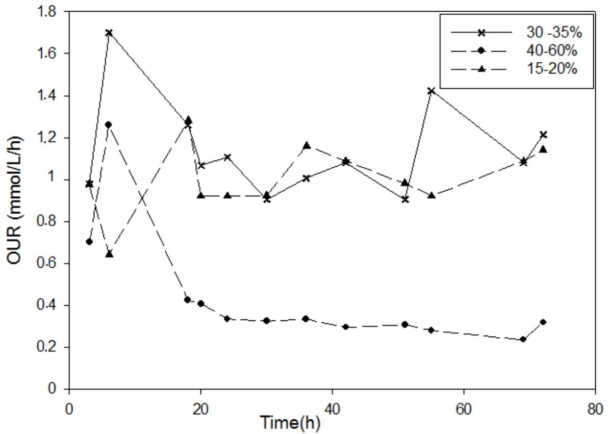
**Figure 4.2** Oxygen uptake rate (OUR) profile of *Y. lipolytica* in crude glycerol at different oxygenation levels (Culture conditions: incubation temperature =  $28 \pm 0.5^\circ\text{C}$ , initial pH =  $6.5 \pm 0.2$ , crude glycerol = 100 g/L)
