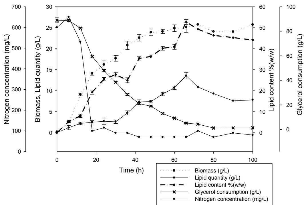
**Figure 3.3** Cell growth and lipid accumulation for *Y. lipolytica* SM7, Culture was performed in the original optimized medium comprising 89 g/L crude glycerol, 0.54 g/L NH<sub>4</sub>OH, pH = 6.5 ± 0.3, Temperature = 28 ± 0.5°C
