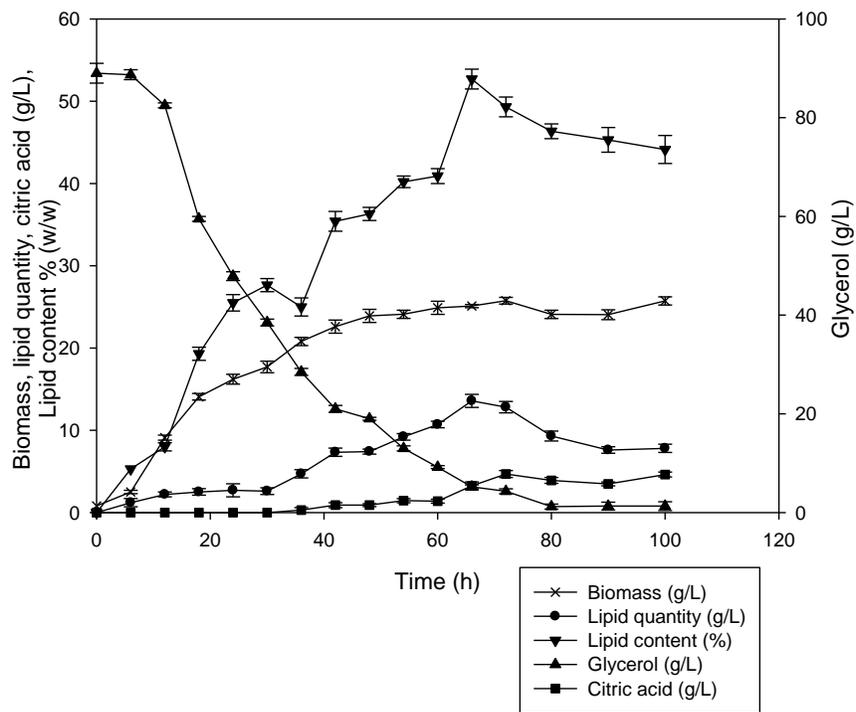
**Figure 5.4** Batch bioreactor fermentation at C/N 75. Crude glycerol was used as a carbon source (89 g/L)
