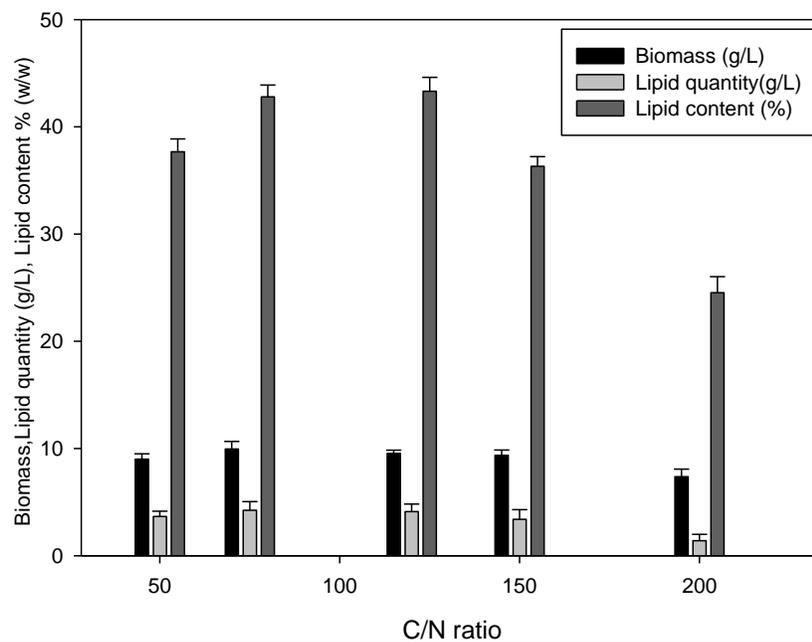
**Figure 5.2** The effect of C/N on the growth and lipid production in *Y. lipolytica*, cultured in shake-flasks (Conditions: T = 28°C, pH = 6.5, 180 rpm, 72 h)
