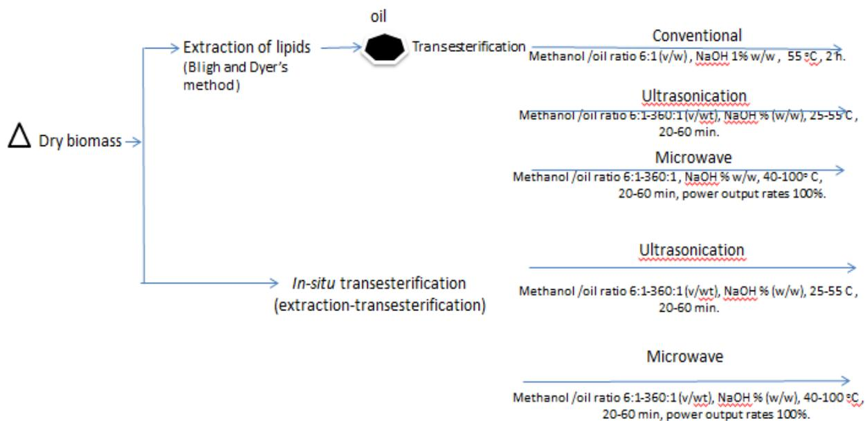
**Figure 7.1 Schematic representation of different transesterification methods**
