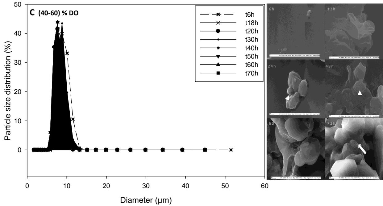
**Figure 4.4** Lipid accumulation of *Y. lipolytica* batch culture under different oxygenation levels. Left, Particle size distribution of fermentation broth. Right, SEM analysis (Arrowhead denotes typical bud scarring, and arrows show areas of lumpy cell wall charact of cells. Scale bar: 1  $\mu\text{m}$ )
