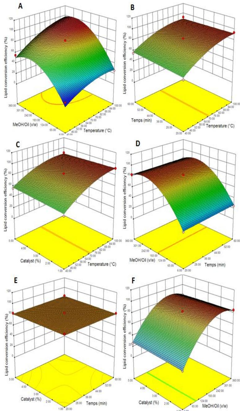
**Figure 7.2** Response surface plots showing binary interaction of different variables. The interaction between: (A) methanol/oil ratio (% v/w) and temperature (°C); (B) temperature (°C) and time (min); (C) catalyst amount (%) and temperature (°C); (D) methanol/oil (% v/w)
