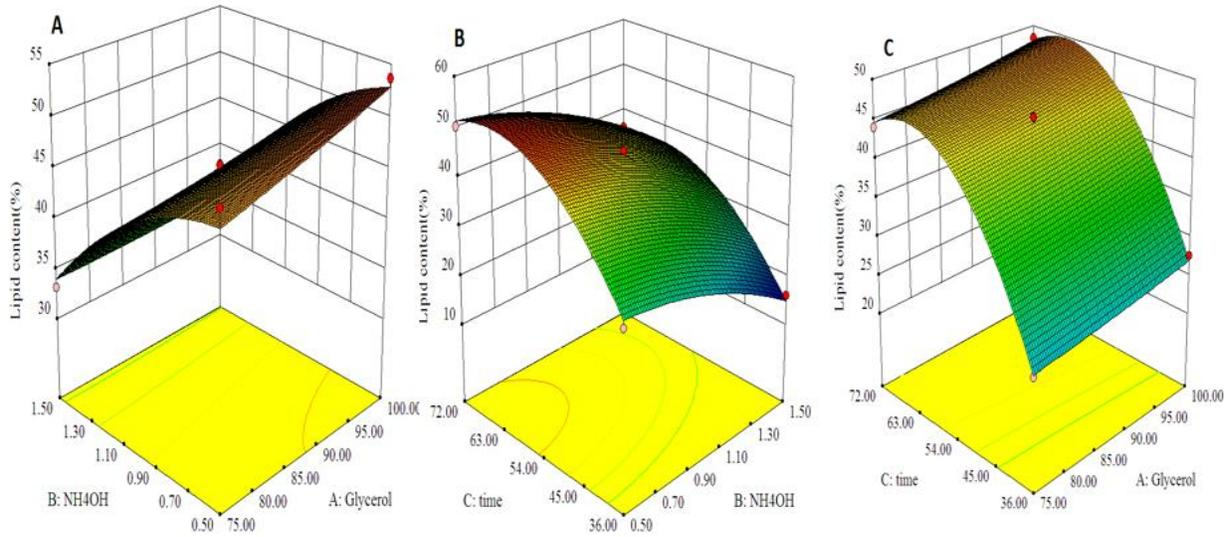
**Figure 3.1** Response surface plots showing binary interaction of different variables. The interaction between (A) NH<sub>4</sub>OH concentration and glycerol concentration, (B) glycerol concentration and fermentation time, (C) fermentation time and glycerol concentration
