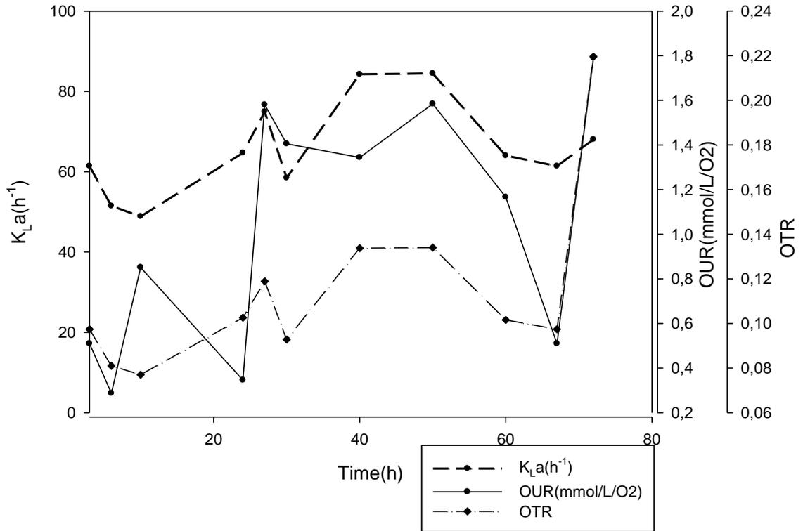
**Figure 3.4** Variation of  $K_{La}$ , OUR and OTR in 5 L fermenter. Culture was performed in the optimized medium on 89 g/L crude glycerol, 0.54 g/L  $NH_4OH$ ,  $pH = 6.5 \pm 0.3$ , Temperature =  $28 \pm 1^\circ C$
