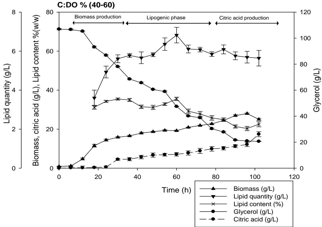
**Figure 4.1** Evolution of biomass concentration, lipid concentration, citric acid, glycerol consumption (g/L) and lipid content% (w/w), under different oxygen concentrations (Culture conditions: incubation temperature =  $28 \pm 0.5^\circ\text{C}$ , initial pH =  $6.5 \pm 0.2$ , crude glycerol = 100 g/L)
