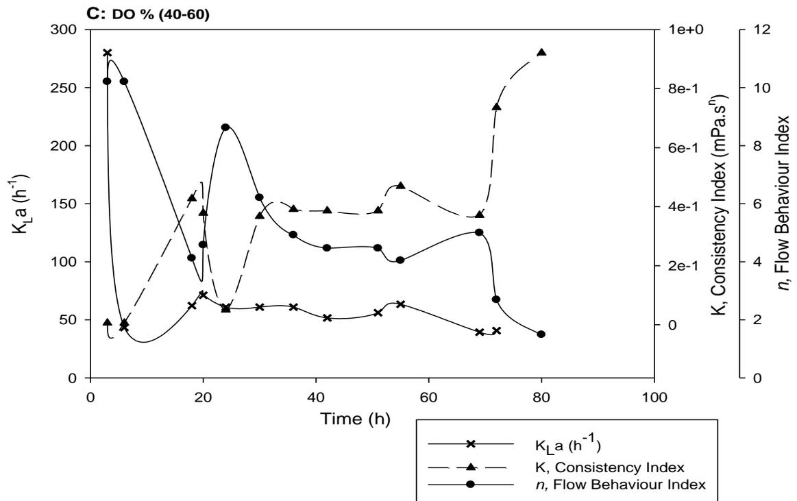
**Figure 4.3** Rheological profile of *Y. lipolytica* at different  $k_L a$  (Culture conditions: incubation temperature =  $28 \pm 0.5^\circ C$ , initial pH =  $6.5 \pm 0.2$ , crude glycerol = 100 g/L)
