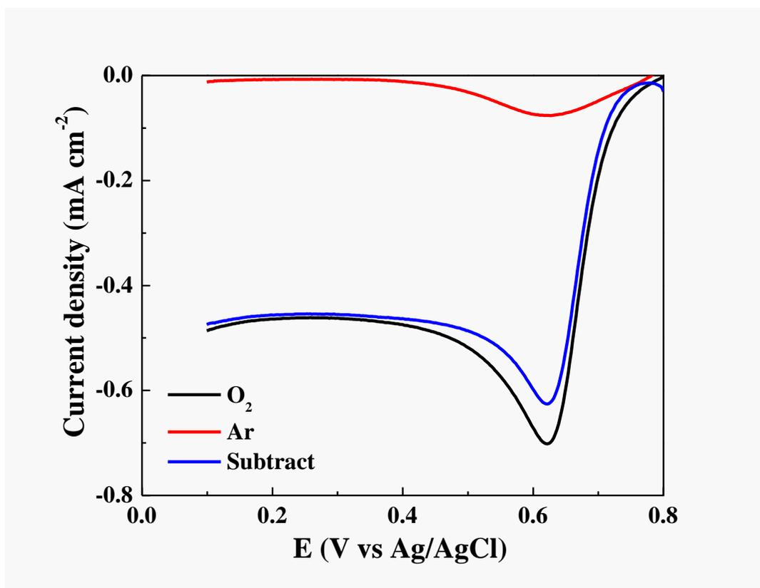
Figure S3: Correction of LSVs from the residual current present 0.5 M H<sub>2</sub>SO<sub>4</sub> argon-saturated before saturation of the solution with oxygen. Potential scan rate of 5 mV s<sup>-1</sup>.
