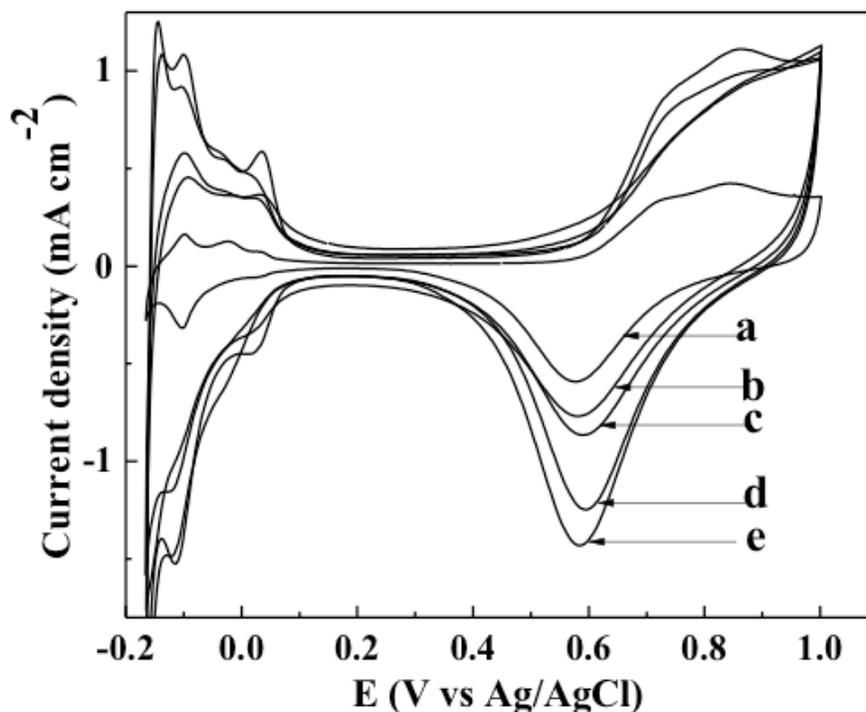
**Fig. 5** Cyclic voltammetry in 0.5 M H<sub>2</sub>SO<sub>4</sub>-argon purged solution with a potential scan rate of 50 mV s<sup>-1</sup>. (a) CP/Pt; (b) CP/(TiO<sub>2</sub>)<sub>2THE</sub>/Pt; (c) CP/(TiO<sub>2</sub>)<sub>0.5THE</sub>/Pt; (d) CP/(TiO<sub>2</sub>)<sub>UV</sub>/Pt; and (e) CP/(TiO<sub>2</sub>)<sub>10mTO2</sub>/Pt electrodes.
