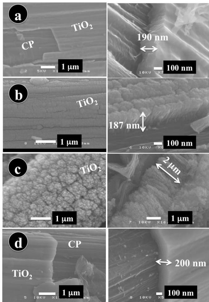
**Fig. 1** Top view and corresponding cross-section SEM micrographs PLD-synthesized  $\text{TiO}_2$  films onto carbon paper substrate. (a)  $(\text{TiO}_2)_{\text{UV}}$ ; (b)  $(\text{TiO}_2)_{0.5\text{THe}}$ ; (c)  $(\text{TiO}_2)_{2\text{THe}}$  and (d)  $(\text{TiO}_2)_{10\text{mTO}_2}$ .
