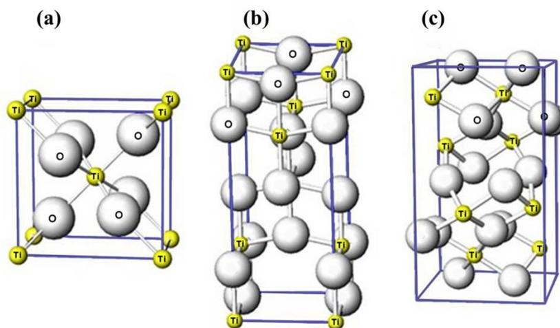
**Figure 2.4** The crystal structure of TiO<sub>2</sub> in phase: a) Rutile, b) anatase, c) brookite.
