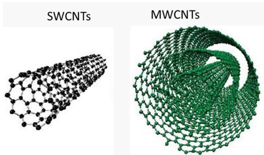
**Figure 3.3 Schematic diagrams of SWCNTs and MWCNTs [6].**
