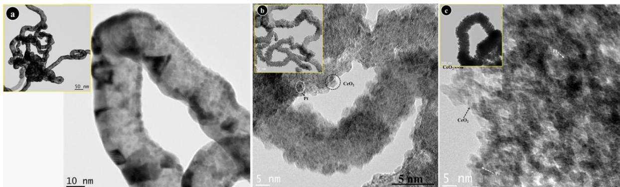
**Figure 3** Upper left panels are TEM and main panels are HR-TEM micrographs of CBPLD-synthesized  $(\text{Pt-CeO}_2)$  films onto CNTs catalyst support. (a)  $(\text{Pt-CeO}_2)_{\text{UV}}$  film; (b)  $(\text{Pt-CeO}_2)_{0.5\text{T}}$  film; and (c)  $(\text{Pt-CeO}_2)_{2\text{T}}$  film.
