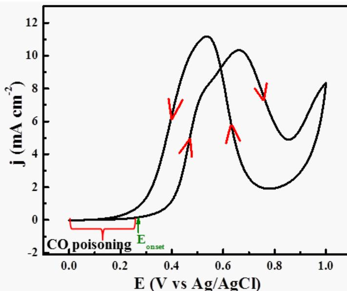
**Figure 3.19** Cyclic voltammogram of CNTs/Pt electrode in 0.5 M H<sub>2</sub>SO<sub>4</sub> + 1.0 M CH<sub>3</sub>CH<sub>2</sub>OH solution with a scan rate of 5 mV s<sup>-1</sup>.
