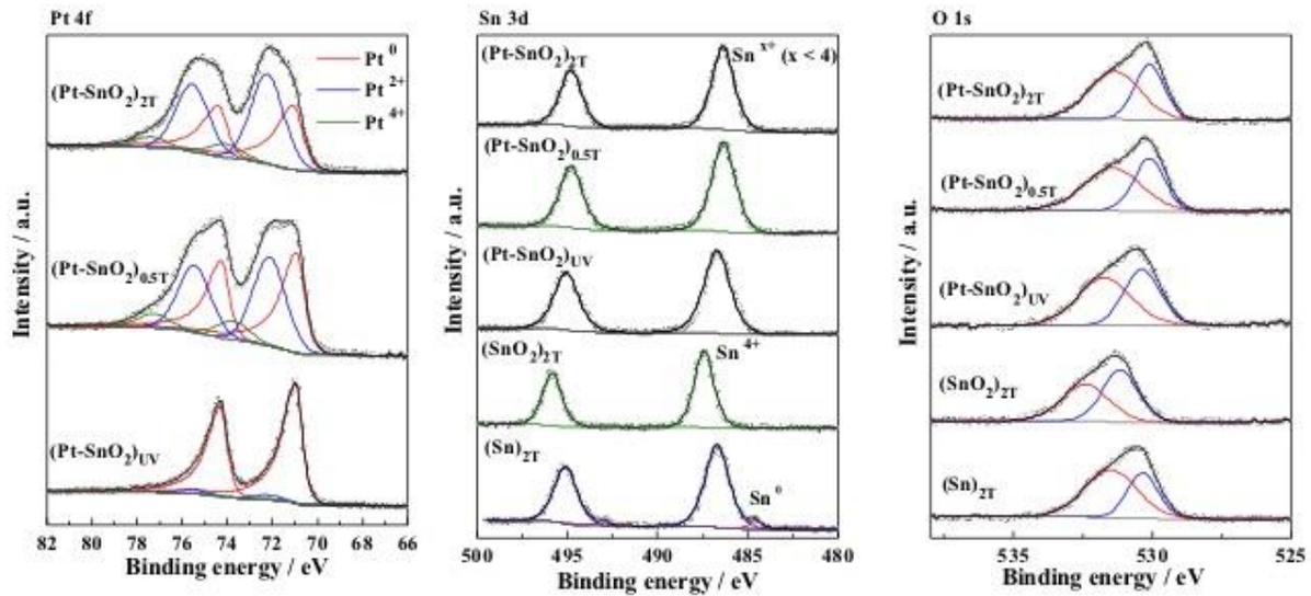
Figure 3. High-resolution XPS spectra (as indicated in the figures) of Pt 4f core level, Sn 3d core level and O 1s core-level.
