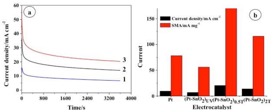
**Figure 6. (a) Durability results in  $0.5 \text{ M H}_2\text{SO}_4 + 1 \text{ M C}_2\text{H}_5\text{OH}$  argon purged solution. (b) Steady-state current density and SMA values extracted from Fig. 6a. (1) CNT/ $(\text{Pt-SnO}_2)_{\text{UV}}$ , (2) CNT/ $(\text{Pt-SnO}_2)_{2\text{T}}$ , and (3) CNT/ $(\text{Pt-SnO}_2)_{0.5\text{T}}$ .**
