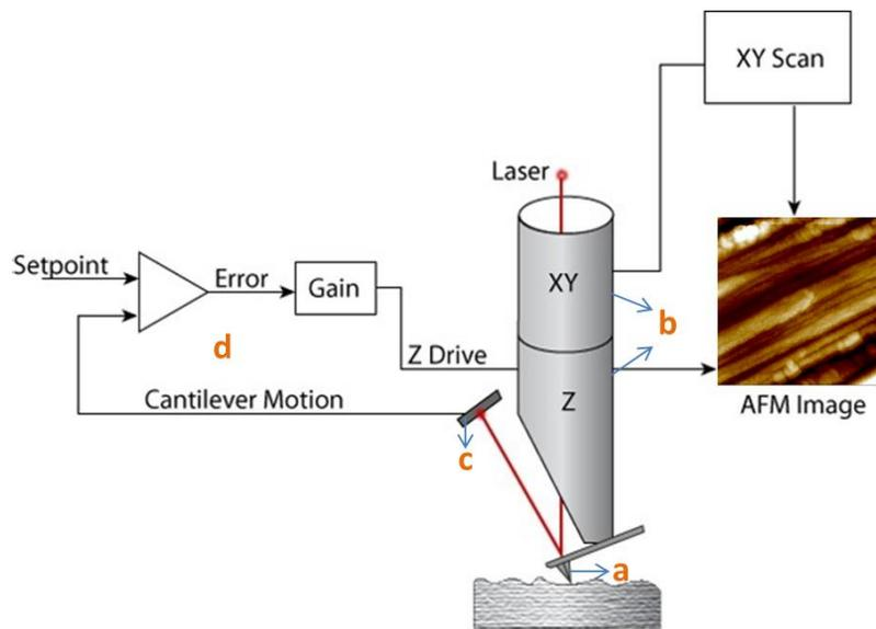
**Figure 3.13 Schematic diagram of AFM with (a) cantilever tip (b) scanner (c) laser beam deflection system and (d) feedback system.**
