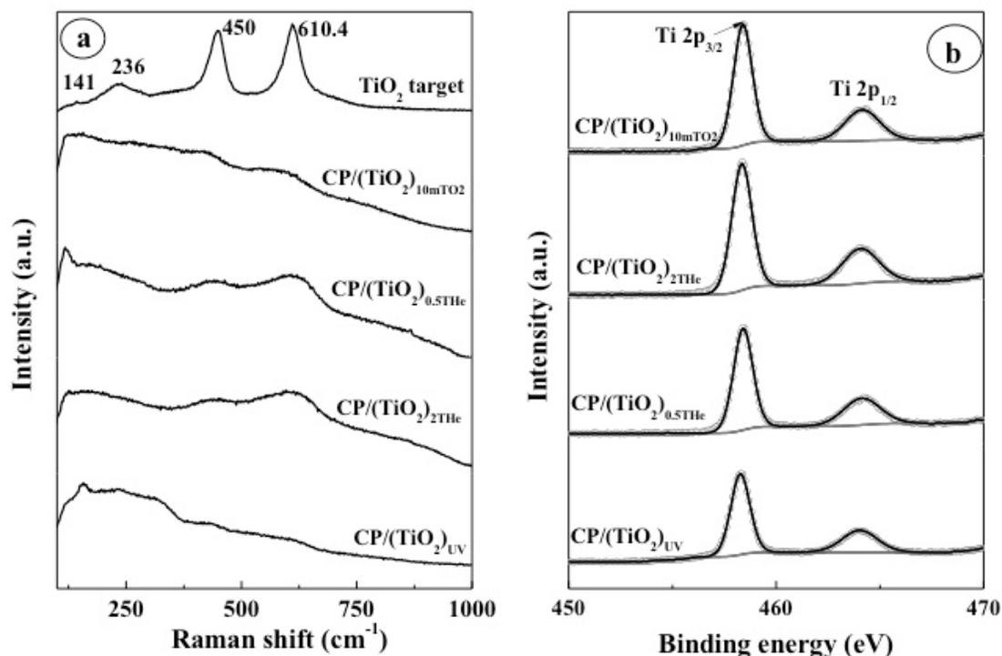
**Fig. 3** Spectroscopy analyses of PLD-synthesized TiO<sub>2</sub> films. (a) Raman spectra. The Raman spectrum of the TiO<sub>2</sub> target is shown for referencing. (b) High-resolution XPS spectra of Ti 2p core level in CP/TiO<sub>2</sub> samples.
