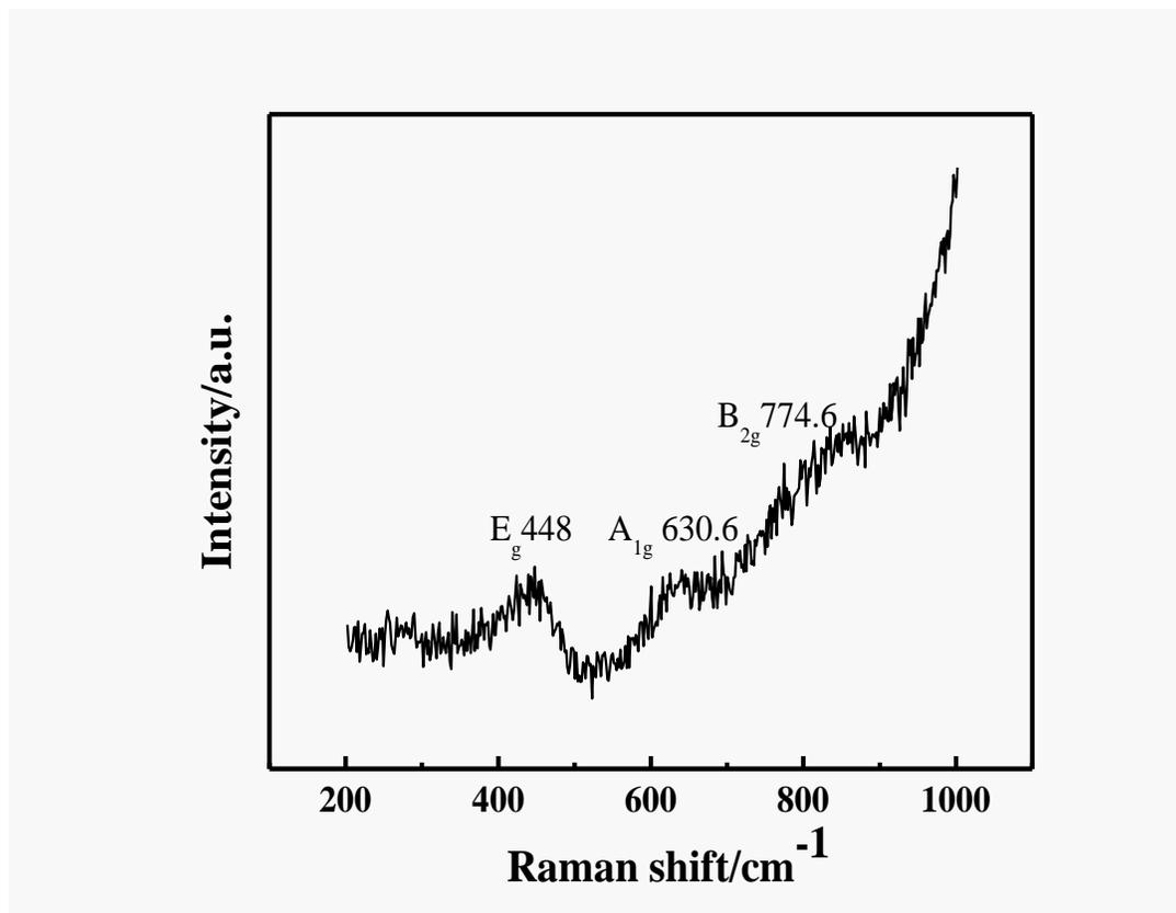
Figure S3 Raman spectrum of CNT/SnO<sub>2</sub> sample. SnO<sub>2</sub> was synthesized onto CNTs using pulsed laser deposition with 20000 laser pulses under 2 Torr of He.
