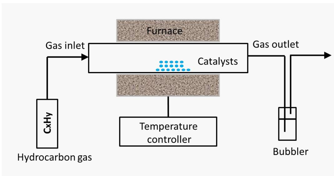
**Figure 3.4 Schematic diagram of the CVD reactor for CNTs growth [13].**
