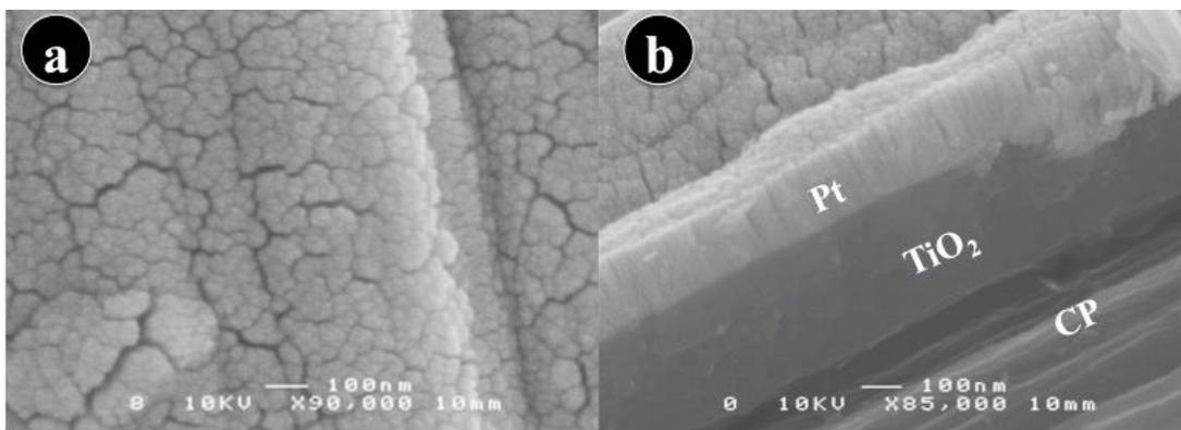
**Fig. 4 Representative top view (a) and corresponding cross-section (b) SEM micrographs of Pt thin film deposited by PLD onto TiO<sub>2</sub> film itself deposited onto CP substrate.**
