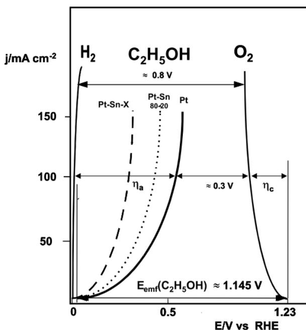
**Figure 2.1**  $j/E$  curves of DEFCs with Pt-based material as anode catalysts, compared to that of a  $\text{H}_2$  PEMFC with Pt catalysts as anode catalysts [19].
