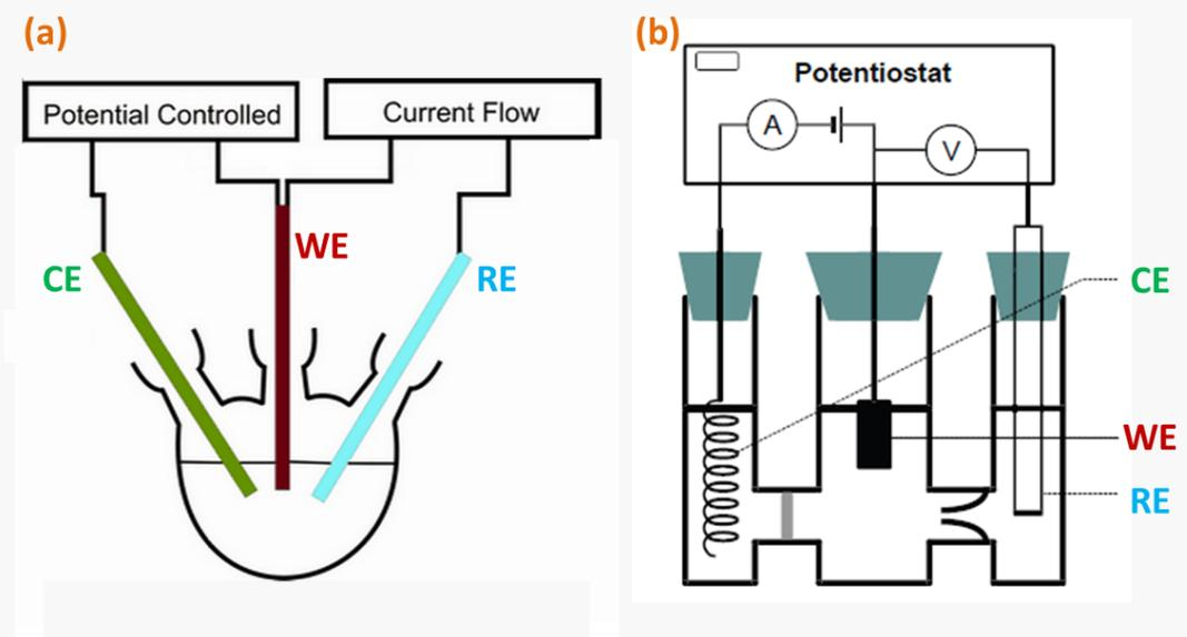
**Figure 3.15** Diagrams of (a) three-electrode setup and (b) three-compartment cell.
