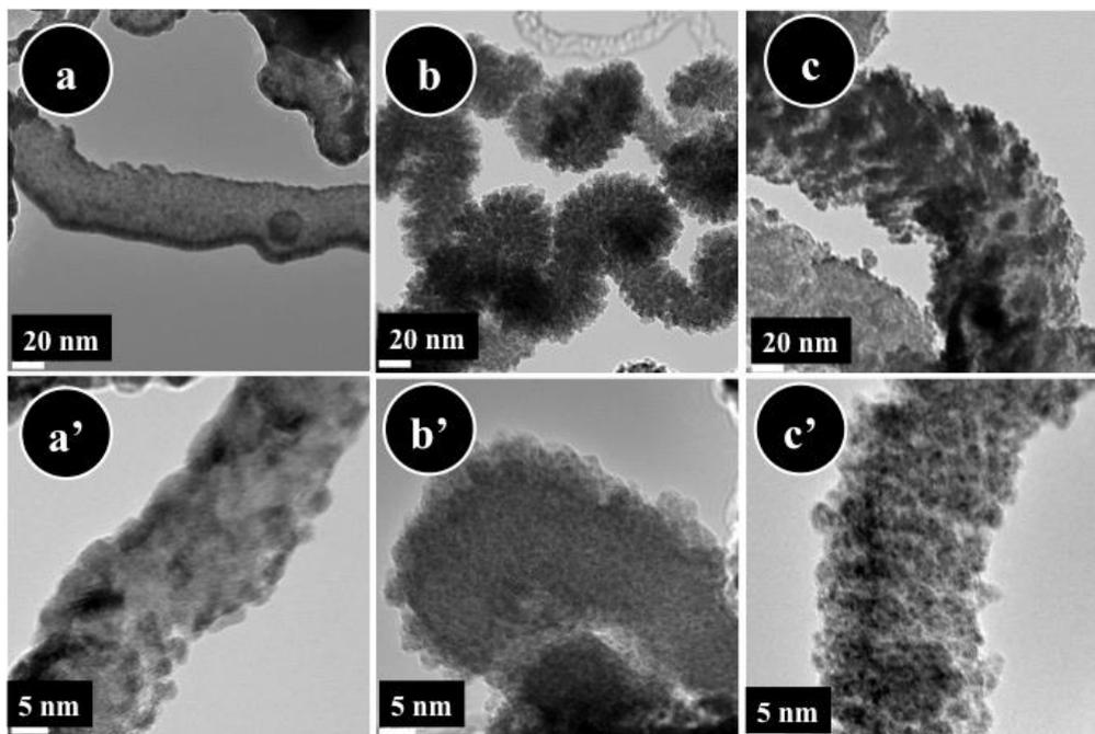
**Figure 4. TEM and HR-TEM micrographs of CBPLD-synthesized (Pt-SnO<sub>2</sub>) nanocomposites onto CNTs catalyst support: (a, a') CNT/(Pt-SnO<sub>2</sub>)<sub>UV</sub>, (b, b') CNT/(Pt-SnO<sub>2</sub>)<sub>0.5T</sub>, and (c, c') CNT/(Pt-SnO<sub>2</sub>)<sub>2T</sub>.**
