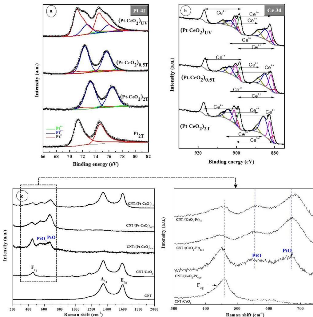
**Figure 2. Spectroscopy analyses of CBPLD-synthesized (Pt-CeO<sub>2</sub>) films. High-resolution XPS spectra of (a) Pt 4f core level (the spectrum of pure Pt is shown for referencing) and (b) Ce 3d core level. (c) Raman spectra. The Raman spectra of bare CNTs and CNT/CeO<sub>2</sub> materials are shown for referencing.**
