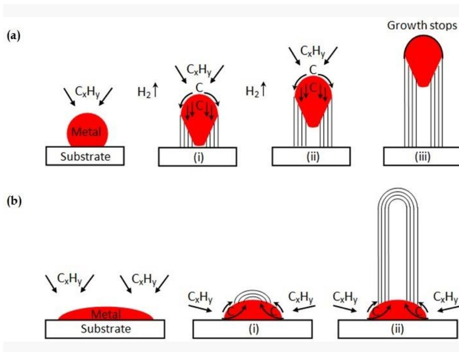
**Figure 3.5 CNTs growth mechanism: (a) tip-growth model (b) base-growth model [13].**
