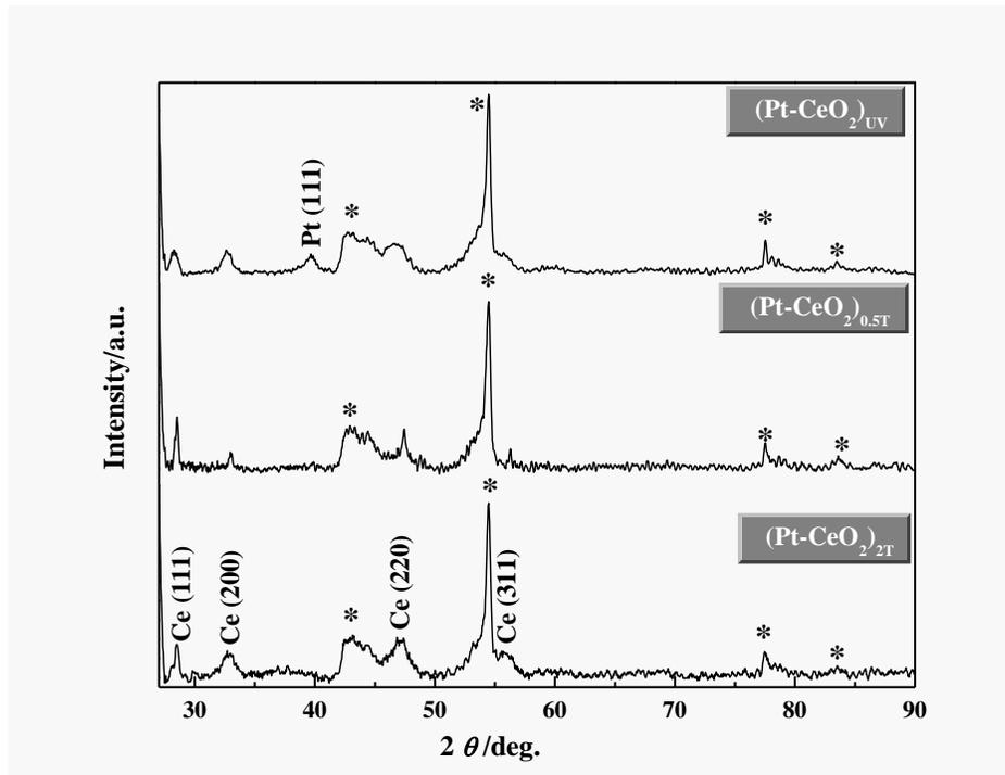
Figure S2: XRD patterns of  $(\text{Pt-CeO}_2)$  samples synthesized under different background gas atmospheres. (\*) are patterns related to carbon.
