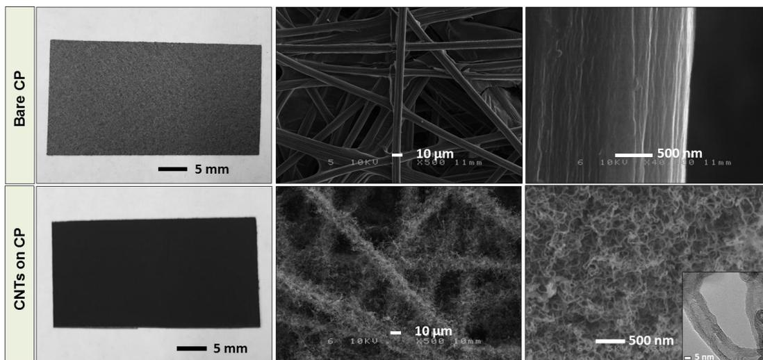
**Figure 3.1** The photos and SEM images with low and high magnifications of bare CP (upper row) and CNTs grown on CP (bottom row).
