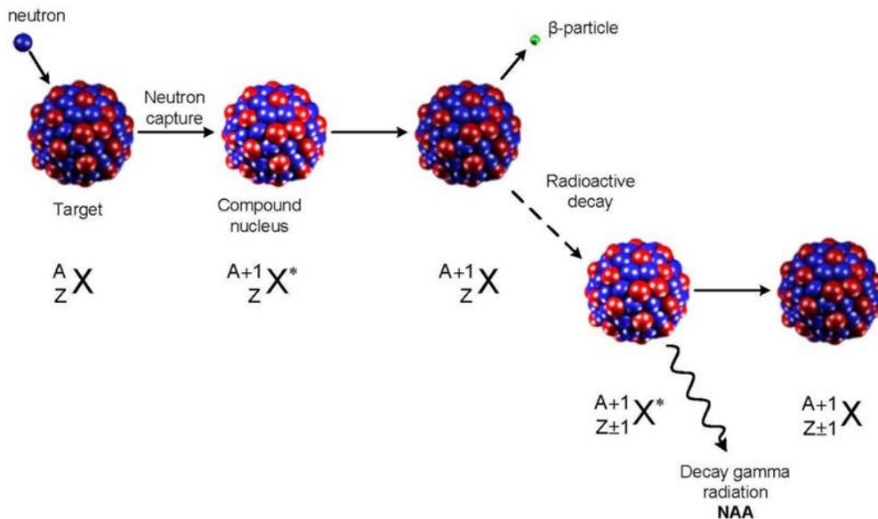
**Figure 3.14 Schematic diagram representing the process of neutron capture by a target nucleus followed by the emission of gamma-rays [54].**
