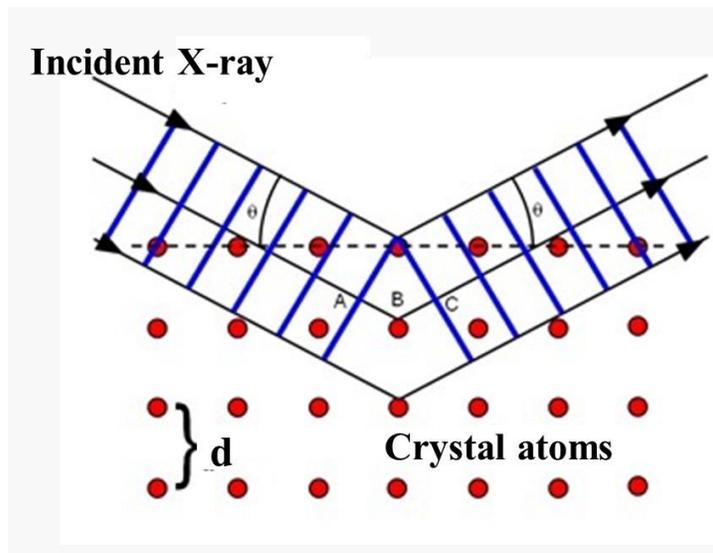
**Figure 3.10 Diffraction of X-ray by parallel planes of atoms in a crystalline material.**
