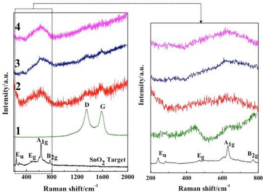
**Figure 2.** Raman spectra of (1) CNTs substrate, (2) CNT/(Pt-SnO<sub>2</sub>)<sub>UV</sub>, (3) CNT/(Pt-SnO<sub>2</sub>)<sub>0.5T</sub> film, and (4) CNT/(Pt-SnO<sub>2</sub>)<sub>2T</sub> nanocomposites. The Raman spectrum of the SnO<sub>2</sub> target is shown for referencing.
