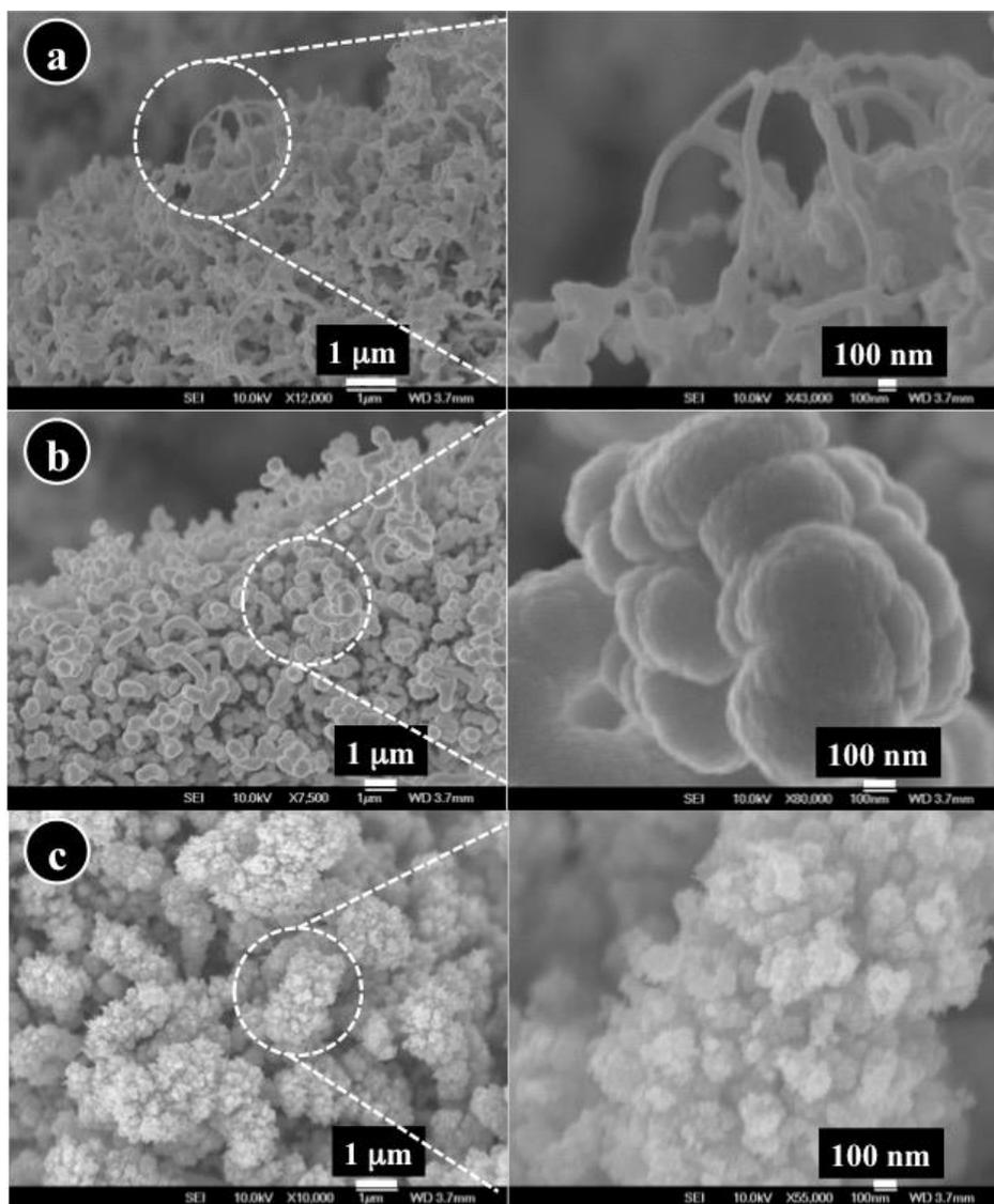
**Figure 1. SEM micrographs with increasing magnification of CBPLD-synthesized (Pt-SnO<sub>2</sub>) nanocomposites onto CNTs catalyst support. (a) CNT/(Pt-SnO<sub>2</sub>)<sub>UV</sub>, (b) CNT/(Pt-SnO<sub>2</sub>)<sub>0.5T</sub>, and (c) CNT/(Pt-SnO<sub>2</sub>)<sub>2T</sub>.**
