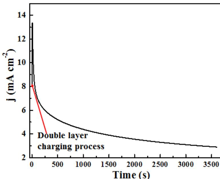
**Figure 3.20 Chronoamperometric curve of CNTs/Pt electrode in 0.5 M  $\text{H}_2\text{SO}_4$  + 1.0 M  $\text{CH}_3\text{CH}_2\text{OH}$  solution at an applied potential of 0.6 V.**
