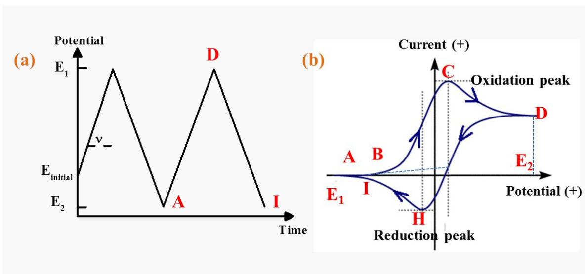
**Figure 3.16 (a) Potential-time wave applied for CV and (b) the resulting i-E curve.**
