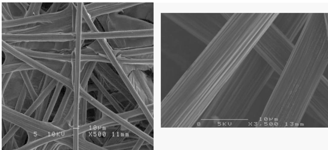
Figure S1: The carbon paper substrate used in this work is an untreated carbon paper (CP, Toray) made of 3D network of carbon fibers each having a diameter ranging between 7 and 10  $\mu\text{m}$ . This type of CP is well known in the area of fuel cells as the gas diffusion layer in Membrane Electrode Assembly (MEA) and it is highly porous with good electrical conductivity and thus can also act as the current collector in the structures developed in this work.
