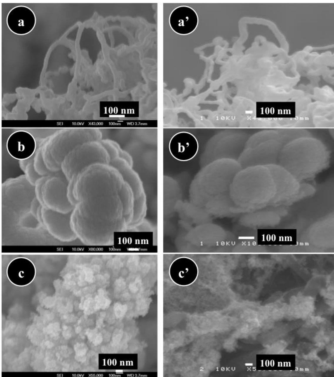
Figure S5 SEM analysis of: as-prepared nanocomposites: (a) CNT/(Pt-SnO<sub>2</sub>)<sub>UV</sub>, (b) CNT/(Pt-SnO<sub>2</sub>)<sub>0.5T</sub>, and (c) CNT/(Pt-SnO<sub>2</sub>)<sub>2T</sub> and their (a'), (b') and (c') are their respective morphologies after durability measurements.
