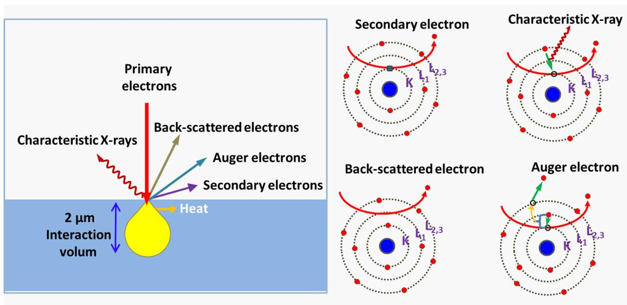
**Figure 3.8 Signals generated from the interaction between SEM electron beam and specimen under study.**
