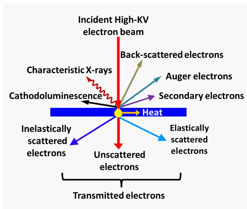
**Figure 3.9** Diagram illustration of the interaction of highly energetic electrons with matter
