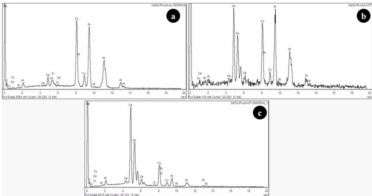
Figure S3: Energy dispersion spectroscopy (EDS) under transmission electron microscope of CNT/(Pt-CeO<sub>2</sub>) samples: (a) CNT/(Pt-CeO<sub>2</sub>)<sub>UV</sub>, (b) CNT/(Pt-CeO<sub>2</sub>)<sub>0.5T</sub>, and (c) CNT/(Pt-CeO<sub>2</sub>)<sub>2T</sub>.
