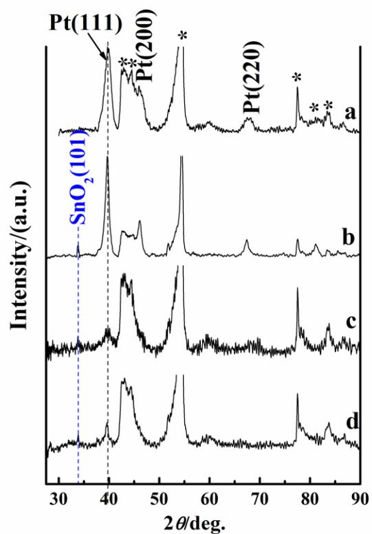
Figure S1 XRD profiles of PLD-deposited Pt and CBPLD-deposited (Pt-SnO<sub>2</sub>) nanocomposites onto carbon nanotubes substrate. (a) CNT/Pt, (b) CNT/(Pt-SnO<sub>2</sub>)<sub>UV</sub>, (c) CNT/(Pt-SnO<sub>2</sub>)<sub>0.5T</sub>, and (d) CNT/(Pt-SnO<sub>2</sub>)<sub>2T</sub> nanocomposites. (\*) patterns related to carbon.
