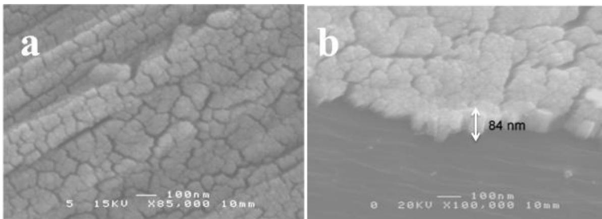
Figure S2: Top view (a) and corresponding cross-section (b) SEM micrographs PLD-synthesized Pt onto carbon paper substrate.
