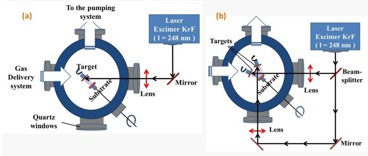
**Figure 3.7 Schematic illustration of (a) PLD and (b) CBPLD setup.**
