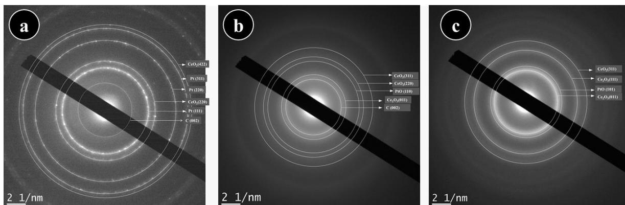
Figure S5: SAED patterns of CNT/(Pt-CeO<sub>2</sub>) samples: (a) CNT/(Pt-CeO<sub>2</sub>)<sub>UV</sub>, (b) CNT/(Pt-CeO<sub>2</sub>)<sub>0.5T</sub>, and (c) CNT/(Pt-CeO<sub>2</sub>)<sub>2T</sub>.
