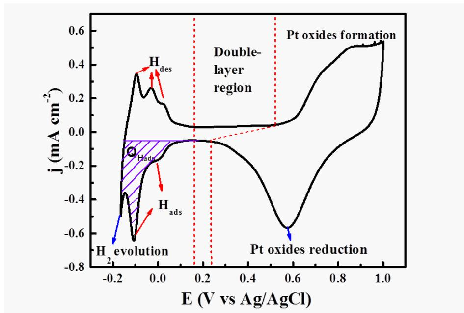
**Figure 3.18** Cyclic voltammogram of polycrystalline Pt electrode in 0.5 M  $H_2SO_4$ -Ar purged solution with a scan rate of  $50 \text{ mV s}^{-1}$ .
