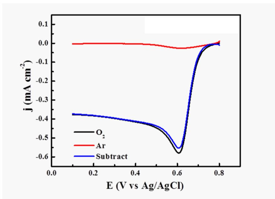
**Figure 3.21** Electroactivity towards oxygen reduction reaction in 0.5 M  $\text{H}_2\text{SO}_4$ -oxygen saturated solution with a potential scan rate of  $5 \text{ mV s}^{-1}$ .
