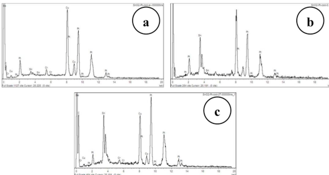
Figure S2 Energy dispersion spectroscopy (EDS) graphs under transmission electron microscope of CBPLD-synthesized (Pt-SnO<sub>2</sub>) films onto CNTs catalyst support. (a) CNT/(Pt-SnO<sub>2</sub>)<sub>UV</sub>, (b) CNT/(Pt-SnO<sub>2</sub>)<sub>0.5T</sub>, and (c) CNT/(Pt-SnO<sub>2</sub>)<sub>2T</sub> nanocomposites.
