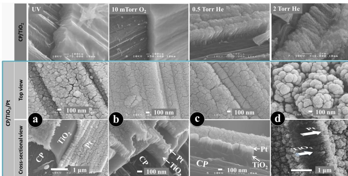
**Figure R2. Micrographies SEM des échantillons CP/(TiO<sub>2</sub>); et des échantillons CP/(TiO<sub>2</sub>)/Pt (a) CP/(TiO<sub>2</sub>)<sub>UV</sub>/Pt; (b) CP/(TiO<sub>2</sub>)<sub>10mTorrO<sub>2</sub></sub>/Pt; (c) CP/(TiO<sub>2</sub>)<sub>0.5THe</sub>/Pt and (d) CP/(TiO<sub>2</sub>)<sub>2THe</sub>/Pt.**
