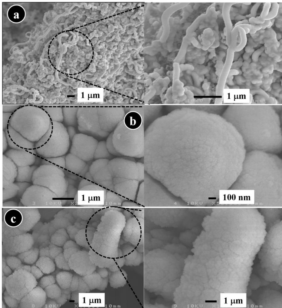
**Figure 1. SEM micrographs with increasing magnification of CBPLD-synthesized (Pt-CeO<sub>2</sub>) films onto CNTs catalyst support. (a) (Pt-CeO<sub>2</sub>)<sub>UV</sub> film; (b) (Pt-CeO<sub>2</sub>)<sub>0.5T</sub> film; and (c) (Pt-CeO<sub>2</sub>)<sub>2T</sub> film.**
