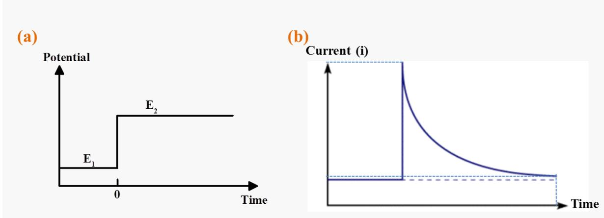
Figure 3.17 (a) Typical waveform of CA and (b) current–time response.
