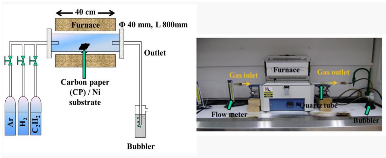
Figure 3.6 Schematic diagram (left) and photo (right) of CVD setup for CNTs growth.
