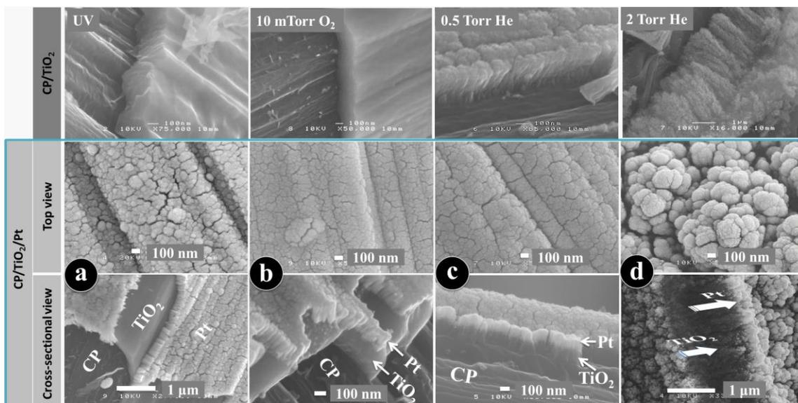
**Figure 5.1 SEM micrographs of PLD-synthesized CP/(TiO<sub>2</sub>) and CP/(TiO<sub>2</sub>)/Pt samples. (a) CP/(TiO<sub>2</sub>)<sub>UV</sub>/Pt; (b) CP/(TiO<sub>2</sub>)<sub>10mTorrO<sub>2</sub></sub>/Pt; (c) CP/(TiO<sub>2</sub>)<sub>0.5TorrHe</sub>/Pt and (d) CP/(TiO<sub>2</sub>)<sub>2TorrHe</sub>/Pt.**
