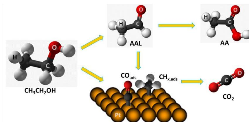
**Figure 2.6 Schematic of the global reaction mechanism for the electro-oxidation of ethanol on Pt electrodes in acidic medium [131, 139, 144].**
