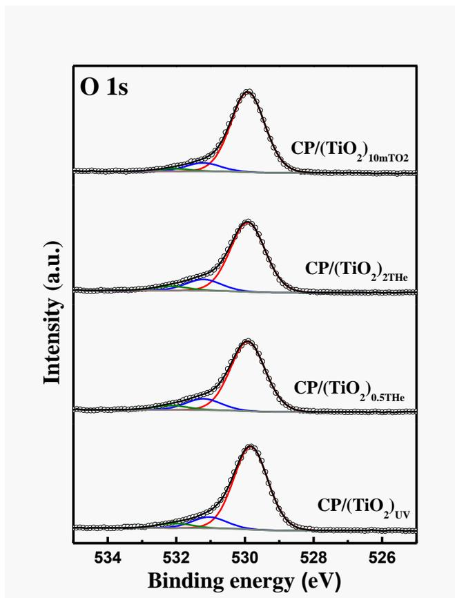
Figure S1: High-resolution XPS spectra of O 1s core level in the TiO<sub>2</sub> films synthesized with PLD.
