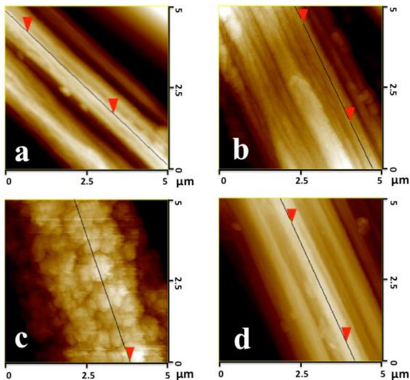
**Fig. 2 AFM images of PLD-synthesized  $\text{TiO}_2$  films onto carbon paper substrate. (a)  $(\text{TiO}_2)_{\text{UV}}$ ; (b)  $(\text{TiO}_2)_{0.5\text{THe}}$ ; (c)  $(\text{TiO}_2)_{2\text{THe}}$  and (d)  $(\text{TiO}_2)_{10\text{mTO}_2}$ .**
