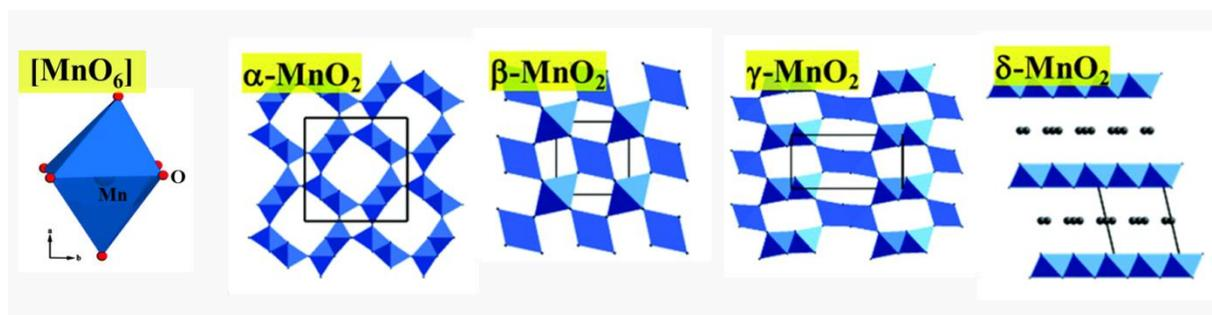
**Figure 2.5 Polyhedral representations of the crystal structures of different  $\text{MnO}_2$  and  $[\text{MnO}_6]$  octahedron.**
