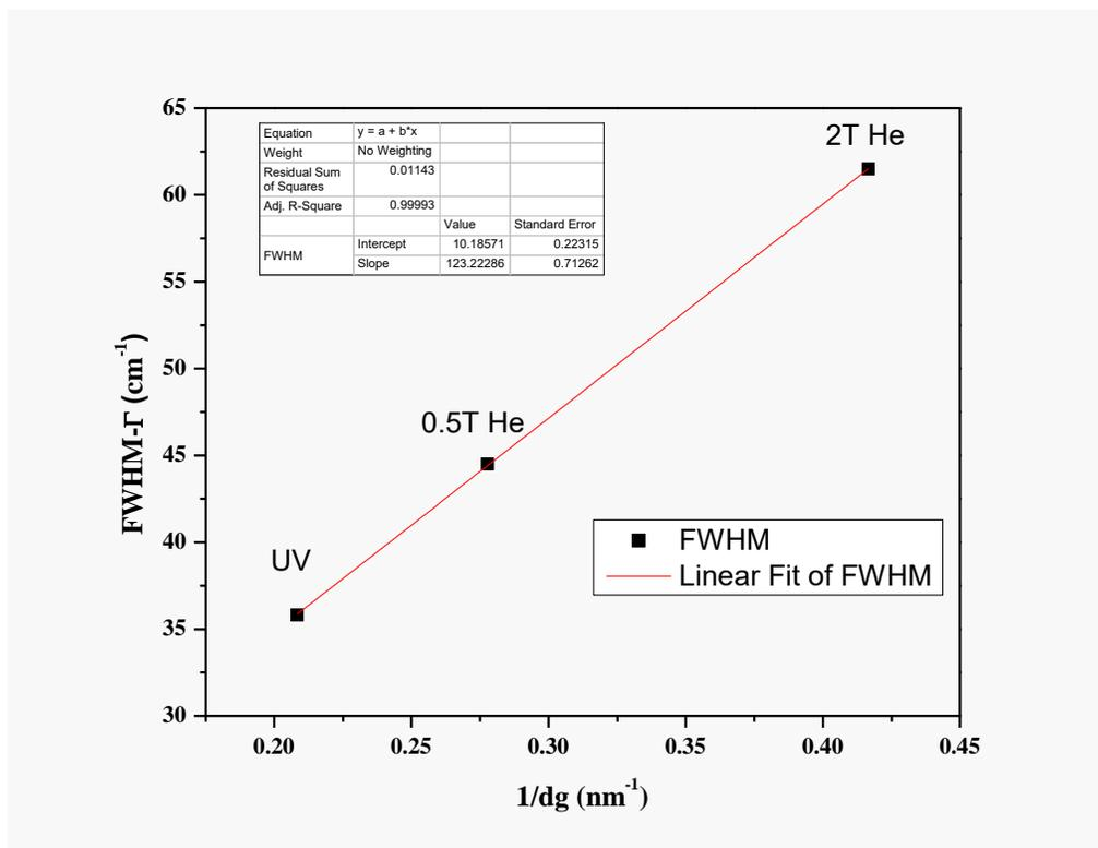
Figure S4: Variation of the half-width,  $\Gamma$ , corresponding to the Raman line of CeO<sub>2</sub> on the inverse of grain size,  $dg$ .
