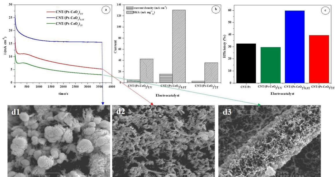
**Figure 5 (a) Durability in 0.5 M H<sub>2</sub>SO<sub>4</sub>+ 1 M C<sub>2</sub>H<sub>5</sub>OH argon purged solution of CBPLD-synthesized (Pt-CeO<sub>2</sub>) films onto CNTs catalyst support. (b) Steady-state density and SMA values extracted from Figure 5a. (c) Efficiency (the efficiency of CNT/Pt catalyst is shown for referencing). Bottom are SEM images taken after durability measurements shown in Figure 5a.**
