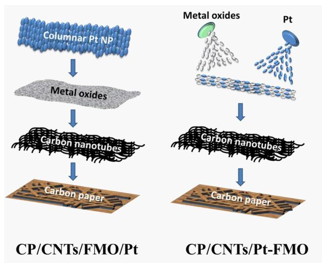
**Figure 3.2** The representation of two catalyst layer architectures containing Pt and FMO: (left) Layer onto layer structure, (right) Co-deposition structure.
