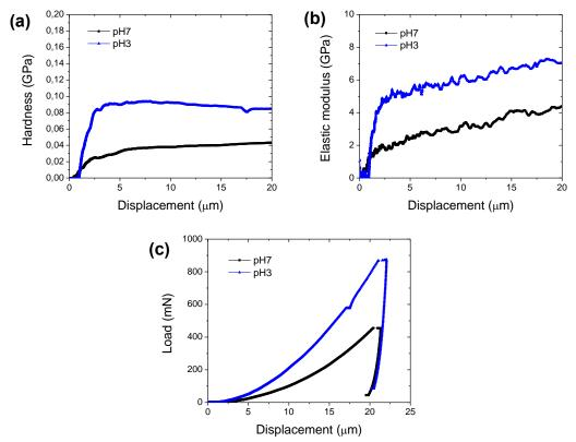
Fig. 6 (a) load/unload, (b) hardness, and (c) elastic modulus curves versus the indentation depth for the pH3 and pH7 coatings.
