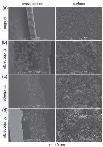
Fig. 4 Cross-sectional and surface SEM images of pH7 electrodes (a) before cycling, (b) after the 1st discharge, (c) after the 1st charge, and (d) after 5 cycles.
