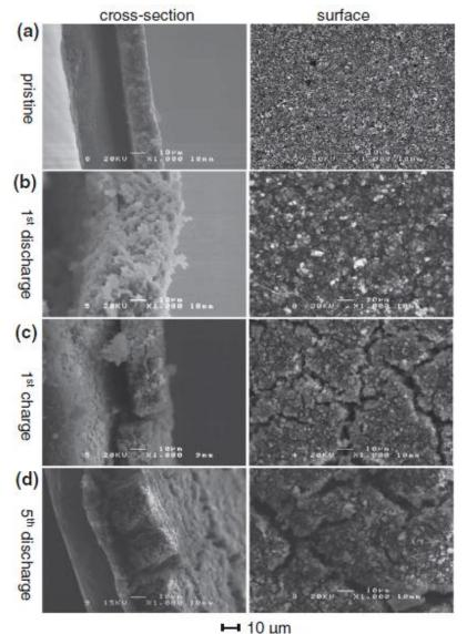
Fig. 3 Cross-sectional and surface SEM images of pH3 electrodes (a) before cycling, (b) after the 1st discharge, (c) after the 1st charge, and (d) after 5 cycles.
