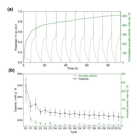
Fig. 4 (a) Typical evolution of the cumulated acoustic activity and electrode potential during the first 10 cycles. (b) Evolution of the electrode capacity and acoustic activity with cycling (mean values based on 8 experiments).
