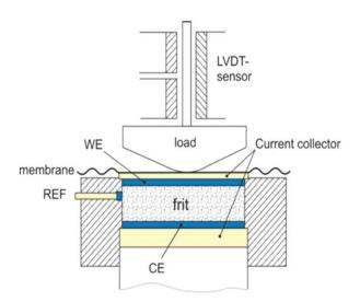
$\textbf{\it Fig. 1} \ Schematic \ diagram \ of \ the \ electrochemical \ dilatometer \ (EL-CELL^{\circledR}).$
