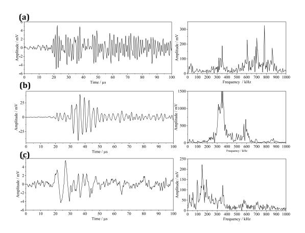
Fig. 7 Typical waveforms and FTT spectra of the AE signals of (A) type 1, (B) type 2 and (C) type 3.
