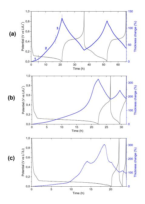
Fig. 5 Evolution of the electrode potential and thickness change during the first two cycles for (a) pH3 electrode and (b, c) pH7 electrodes. The current density is 180 mA g-1 Si.
