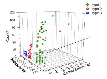
Fig. 8 Distribution as a function of their frequency, number of counts and energy of the three types of signals identified from manual clustering of the AE events detected during the first two cycles.
