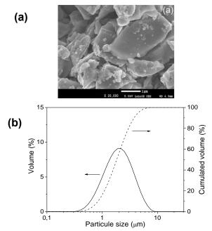
Fig. 2. (a) SEM micrographs and (b) particles size distribution of the asreceived Si powder.
