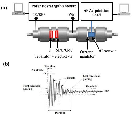
Fig. 1. (a) Schematic diagram of the experimental set-up coupling AE and electrochemical measurements. (b) Main acoustic characteristics recorded on a typical waveform AE signal.
