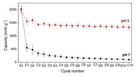
Fig. 2 Evolution with cycling (10 cycles) of the discharge and charge capacities for the pH3 and pH7 electrodes (means values based on 7-8 experiments using Swagelok half-cells).
