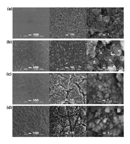
Fig. 3. SEM micrographs at different magnifications of the electrode surface (a) before cycling, (b) after the 1st discharge (lithiation), (c) after the 1st charge and (d) after the 10th cycle.
