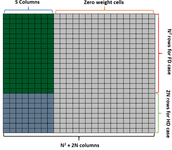
Figure 3.3: Structure of the matching weight matrix.
