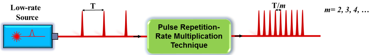
Figure 1.15 – Pulse repetition-rate multiplication technique to increase the repetition-rate of a low-rate laser source.
