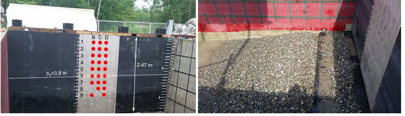
Figure 2. The central instrumented wall is mainly composed of an aluminium plate with 25 pressure sensors (in red) installed. A flat steel plate (right picture) is welded at the bottom to prevent scouring.
