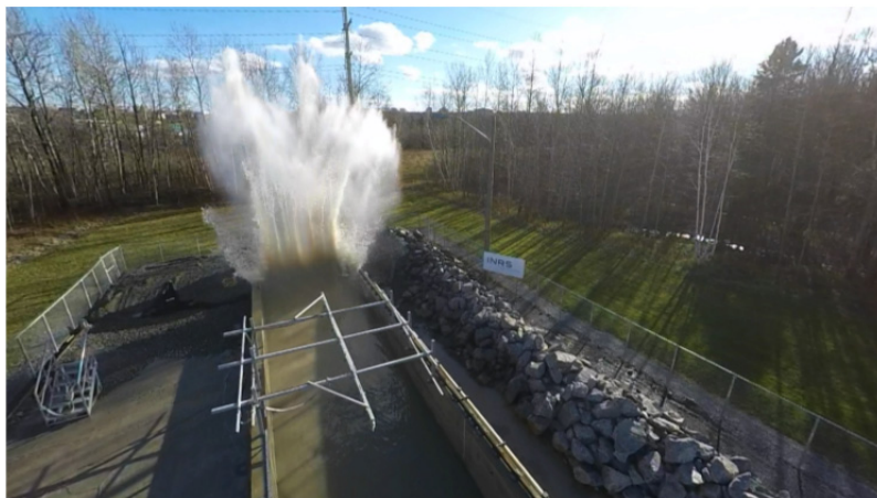
Figure 1. Impact on a seawall in the Quebec Coastal Physics Laboratory facilities.
