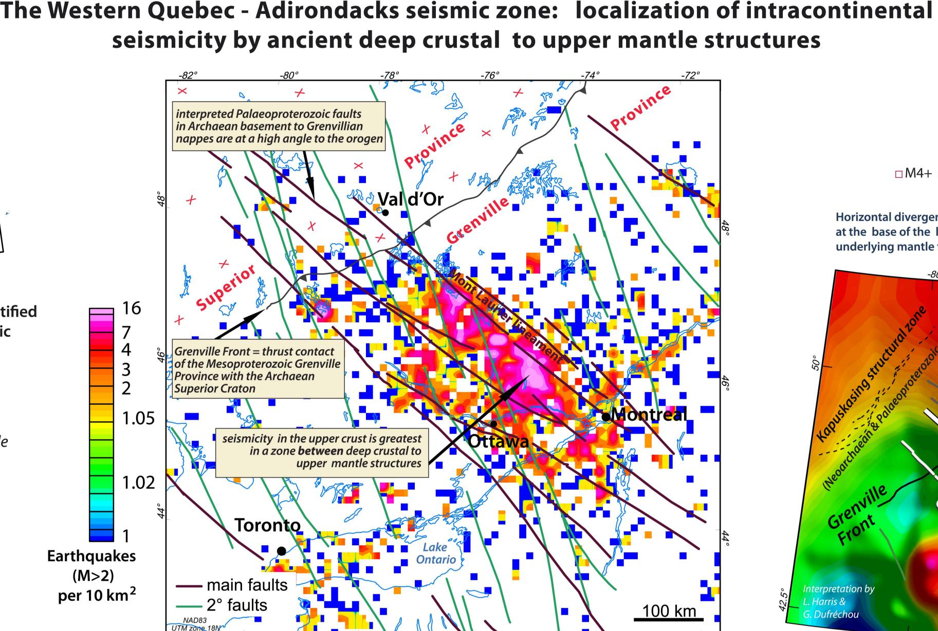
Gravity lineaments (= deep crustal to mantle structures) define boundaries to areas of greatest seismicity: structures act as stress guides
