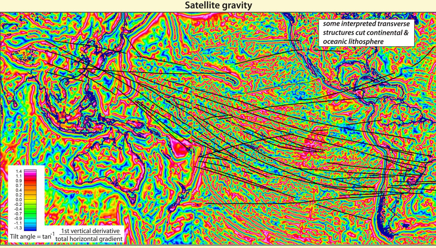
Tilt angle of long wavelength component highlights linear features = deep crustal to mantle structures
