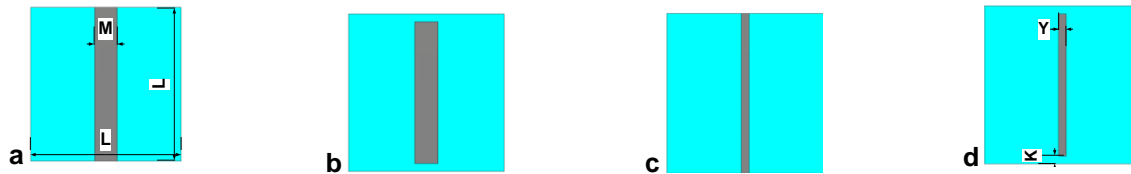
Figure 3-3 Conventional strip line FSS unit cell-Dimensions (mm): M=1.5 , L=10 , Y=.5 , K=0.5 , Y=0.5 .
