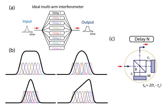
Figure 1.13 – (a) Conceptual diagram of the pulse shaping technique based on the concept of temporal coherence synthesization; (b) Examples of synthesized temporal waveforms: flat-top, parabolic, triangular and trapezoidal pulse; (c) Schematic of a single stage of the multi-stage interferometric setup for pulse shaping based on this concept. B: 50:50 beam splitter; M: Mirror. Figure reproduced from Ref. [52]
