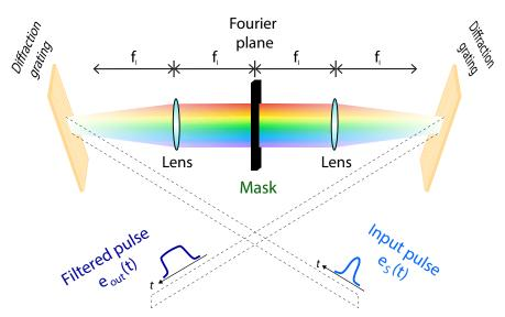
Figure 1.11 – Schematic of a spatial-domain filter for time-domain optical pulse shaping. The optical pulses are pre- and post- converted to the spatial-domain by means of diffraction gratings.
