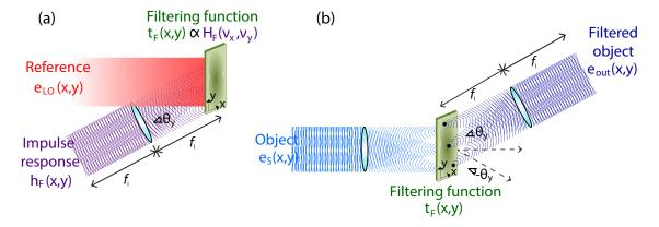
Figure 3.5 – Vander-Lugt filter: (a) Recording of the hologram, which contains information on the amplitude and phase of the complex-valued filter transfer function and (b) signal filtering process based on the concatenation of two Fourier-transforming systems and placing the hologram in the Fourier plane.
