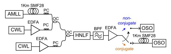
Figure 4.14 – Experimental setup of the XPM-based wavelength converted scheme for complexenvelope optical signals. AMLL: Active mode-locked laser; PC: Polarization controller; CWL: Continuous-wave laser; EDFA: Erbium-doped fiber amplifier. OSO: Optical sampling oscilloscope.
