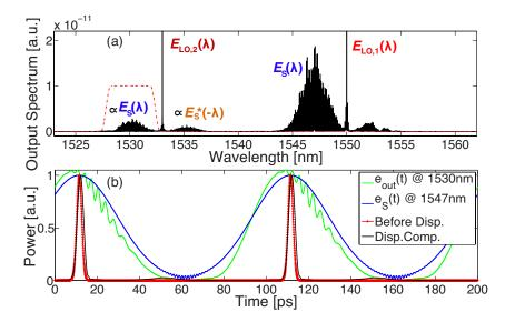
Figure 4.12 – Results from the numerical simulation of the proposed scheme (no phase-matching) (a) Spectrum at the output of the HNLF; dashed red line represents the applied numerical BPF (b) Resulting temporal waveform after the BPF (green line); transform-limited input before propagation through the SMF (red line); input chirped signal to be conjugated (blue line); wavelength-converted output after compensating the dispersion from the SMF (black line).
