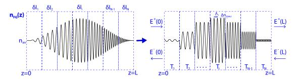
Figure B.2 – Schematic of the division into layers of a non-uniform FBG for its analysis using CMT. The complete grating structure is divided into layers containing few periods, and each layer is treated as a uniform FBG. The analysis of the complete structure is done based on TMM. The propagating waves' dependence with the angular frequency has been omitted in the figure for simplicity.
