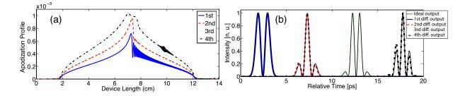
Figure 5.10 –  $N^{th}$ -order optical differentiators (up to N = 4) based on FBGs in transmission: (a) Apodization profiles considering realistic spatial resolution (limited to 0.5 mm); (b) Time-domain intensity outputs from practical FBG-based differentiators.
