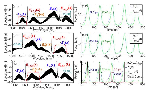
Figure 4.15 – (a) Down-conversion of  $e_S(t)$ ; (b) Up-conversion of  $e_S(t)$ ; (c) Down-conversion of  $e_S^*(t)$ ; a-c (1) Spectrum after HNLF; a,b (2) Temporal signal after BPF (green line) vs input signal (dashed blue line); c (2) includes output from AMLL (red line) and signal after dispersion compensation (black line).
