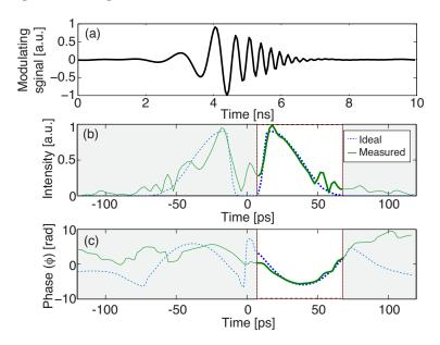
Figure 5.5 – Asymmetric triangular pulse with parabolic phase: (a) spectral hologram  $H_{hc}(t)$ ; (b) temporal intensity of the output signal; and (c) temporal phase of the output signal: target (dotted blue line) and measured (solid green line) output. The spectral hologram was designed so that the right-hand side of the temporal output (highlighted and marked with a dashed red line) matches the target profile.
