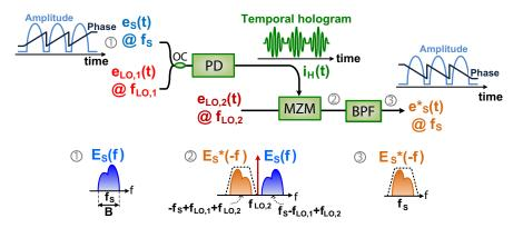
Figure 4.7 – Scheme to perform TPC based on time-domain holography. The scheme comprises the concatenation of the detection and reconstruction steps of holography, in this case using two different reference signals in each step.
