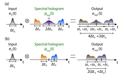
Figure 5.1 - (a) Temporal width of the output signal resulting from convolving the input signal to be processed with the impulse response of the spectral hologram; (b) Temporal width of the output signal if the terms proportional to the intensity of the target impulse response and reference signal are not considered in the generation of the spectral hologram.
