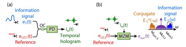
Figure 4.1 – Implementation of the concept of time-domain holography as the temporal counterpart of spatial-domain holography. (a) Generation of the temporal hologram; (b) Retrieval of the complex information signal. For the sake of simplicity, the optical temporal signals are represented by their amplitude envelope. OC, optical coupler; PD, photodetector; MZM, Mach-Zehnder modulator.
