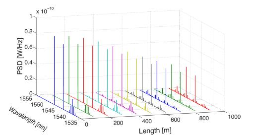
Figure 1.3 – Example of the evolution of the spectrum of three input optical signals (centered at different carrier wavelengths) in their propagation along a HNLF (1 km-long). New frequency components are generated due to the effect of  $\chi^{(3)}$ . The simulation has been carried out solving the nonlinear Schrödinger equation by using the split-step Fourier method [19].
