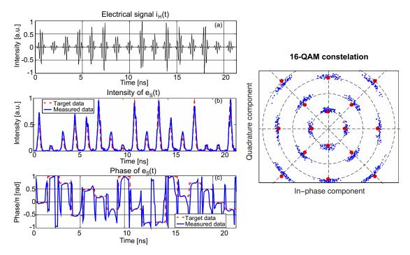
Figure 4.6 – 1024-symbol 16-QAM optical data stream. (a) A portion of the numerically designed temporal hologram, shown over 16 consecutive symbols, as generated by the electrical AWG; (b) Intensity and (c) phase profiles of the generated complex-envelope optical signal (solid blue line) and target data stream (dashed red line) over the signal portion (16 symbols) shown in (a); (d) Constellation of the generated data stream (blue points) and ideal constellation of a 16-QAM signal.
