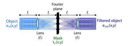
Figure 3.4 – Spatial filtering process. The first lens generates the Fourier transform of the object wave; in the Fourier plane (at twice the focal length  $f_l$  of the lens), an amplitude or phase mask modulates the traveling wave; finally a second lens in the same configuration at the previous one generates the Fourier transform of the modulated wave. The total system performs the operation of convolution. For simplicity, the coordinates in all the planes have been labeled as (x, y).
