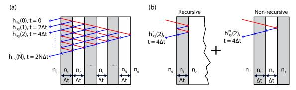
Figure B.5 - (a) Layout of the division of the FBG in layers and the contribution to the total sampled impulse response; (b) The calculation of the refractive index of each layer is obtained from the non-recursive component of the impulse response in this layer. To this purpose, the total sampled impulse response is decomposed into the recursive component and the non-recursive component, where the total impulse response and its non-recursive component are known.
