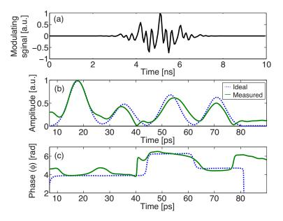
Figure 5.6 – 4-symbol 16-QAM code: (a) spectral hologram  $H_{hc}(t)$ ; (b) temporal amplitude of the output signal, just right-hand side is shown; (c) temporal phase of the output signal: target (dotted blue line) and measured (solid green line) output.
