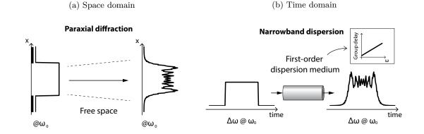
Figure 1.6 – Schematic diagram of the duality between spatial paraxial diffraction and first-order temporal dispersion: (a) Propagation of a plane wave through a rectangular aperture in free space. For simplicity, the problem has been reduced to the x-axis in the illustration. The same behavior would be observed in the y-axis. (b) Propagation of a temporal rectangular pulse through a first-order dispersion medium.
