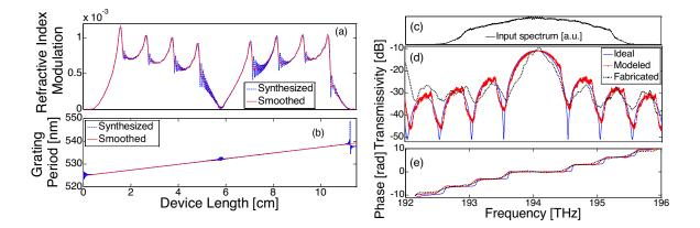
Figure 5.11 – Flat-top pulse shaper based on an FBG in transmission: Obtained grating apodization profile (a) and period (b) from synthesis (blue line) and smooth profiles adapted to fabrication constraints, i.e., spatial resolution  $\geq 1 \text{ mm}$  (red line); (c) Input signal spectrum; (d) transmissivity and (e) transmission phase response: ideal (blue line), simulated considering fabrication constraints (red line) and measured from fabricated device (dotted black line).
