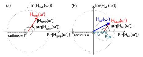
Figure 5.13 – (a) Phasor diagram of  $H_{NMP}(\omega')$ ; (b) Phasor diagram of  $H_{MP}(\omega')$ , illustrating how its phase varies only between  $-\pi/2$  and  $\pi/2$ .
