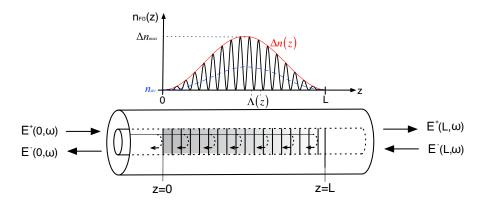
Figure B.1 – Nomenclature for the optical waveforms at the two extremes of an FBG of length L.
