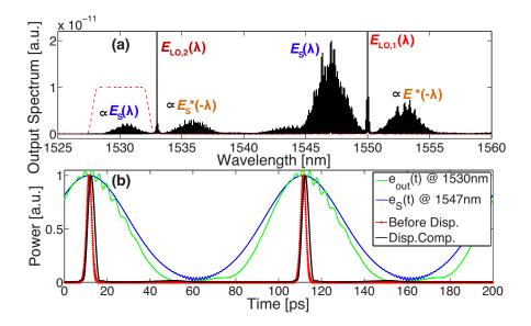
Figure 4.13 – Results from the numerical simulation of the proposed scheme (a) Spectrum at the output of the HNLF; dashed red line represents the applied numerical BPF. (b) Resulting temporal waveform after the BPF (green line); transform-limited input before propagation through the SMF (red line); input chirped signal to be conjugated (blue line); wavelength-converted output after compensating the dispersion from the SMF (black line).
