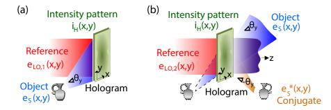
Figure 3.1 - (a) Signal recording step and (b) signal retrieval step in classical holography. The figure represents the geometry proposed by Leith and Upatnieks, from which the information signal and its conjugate appear angularly separated from the reference and ambiguity components.
