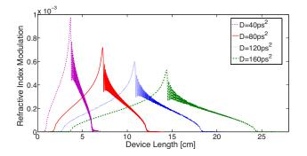
Figure 5.8 – First-order optical differentiator based on an FBG in transmission: Grating apodization profiles and device lengths obtained for different values of the dispersion parameter.
