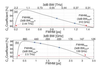
Figure 5.17 – PHT based on an FBG in transmission: Cross-correlation coefficient between the output of the measured PHT and an ideal PHT vs. the temporal FWHM (or 3dB bandwidth) of an input Gaussian pulse; (a) integer PHT; and (b) fractional PHT. The position of the input pulses in the temporal characterization is marked by a blue cross.
