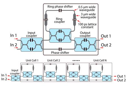
Figure 1.12 – Schematic design of a single unit-cell lattice filter, at the top of the figure, and example of an *N*-unit cell filter, at the bottom. Figure reproduced from Ref. [134].
