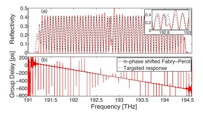
Figure 5.14 – PHT based on an FBG in transmission: (a) Reflectivity and (b) Group delay. The dashed black line represents the specified spectral response and the red line represents the spectral response of an FBG-based  $\pi$ -phase shifted Fabry-Perot structure.
