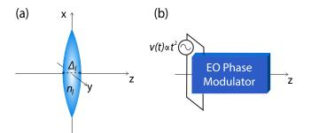
Figure 1.7 – (a) Conventional space lens; (b) Time lens implemented with a phase modulator driven by a quadratic voltage.
