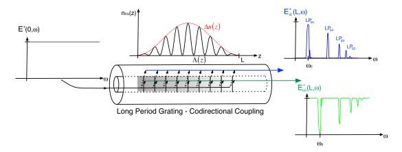
Figure 1.10 – Schematic diagram of a long-period fiber grating (LPG), indicating two operation possibilities, the core-to-core mode and the core-to-cladding mode. In the figure, coupling to a higher-order cladding mode (LP<sub>05</sub>) is assumed.
