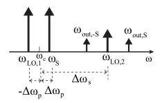
Figure 4.11 – Scheme of the central frequency of the signals involved in the wavelength conversion process and nomenclature given to the spectral separation between signals to develop the equations of phase-matching condition (Eqs. 4.12 and 4.13).
