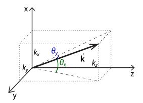
Figure 1.5 – Schematic illustrating the angles of propagation of a traveling plane wave with wavevector  $\vec{k}$ .
