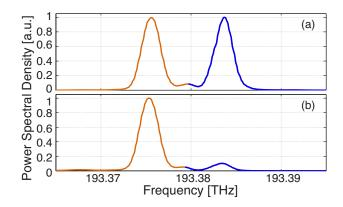
Figure 4.8 – Power spectral density of (a) the real optical signal after the modulation process; (b) the complex-envelope optical signal after the BPF. The spectrum of the input signal  $e_S(t)$  is nearly coincident with (b).
