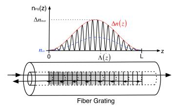
Figure 1.8 – Schematic of the sinusoidal perturbation at the core of an optical fiber, creating a fiber grating. The lower figure depicts light coupling to a counter-propagating mode.
