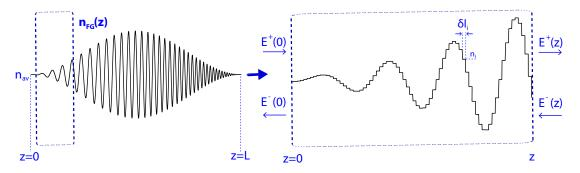
Figure B.3 – Schematic for division into layers of a non-uniform FBG for its analysis using ML-TMM. The complete grating structure is divided into layers with a length at least one order of magnitude shorter than the minimum value of the period, and each layer is treated as medium of constant refractive index. The analysis of the complete structure is done based on TMM. The optical waves' dependence with the angular frequency has been omitted in the figure for simplicity.
