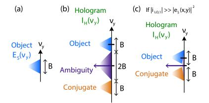
Figure 3.2 – Spectral content of (a) information signal  $e_S(x,y)$ , (b) hologram, and (c) hologram considering that  $i_{LO} \gg |e_S(x,y)|^2$ .
