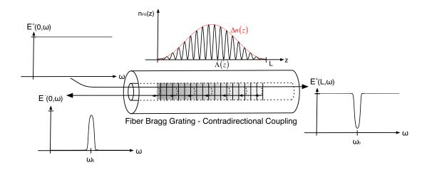
Figure 1.9 – Schematic diagram of a fiber Bragg grating (FBG), indicating two operation possibilities: the reflection mode and the transmission mode.  $\omega_0$  is the Bragg angular frequency,  $\omega_0 = 2\pi c_0/\lambda_0$ .
