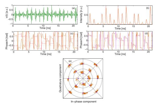
Figure 4.10 - TPC of a 1024-symbol 16-QAM optical data stream. (a) Temporal hologram of the input signal; (b) Detected intensity of the conjugated signal; (c) Detected phase of the conjugated signal (orange line); (d) Comparison between the detected phase (orange line) and phase of the ideally conjugated input (dashed purple line), and (e) Output constellation (purple circles represent the symbol's ideal positions).
