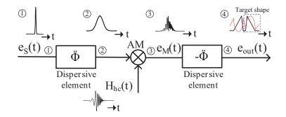
Figure 5.3 – Schematic of operation of the TDSS system. Vander-Lugt filters are based on this configuration, but using a spectral hologram as the modulating signal. AM: amplitude modulation.
