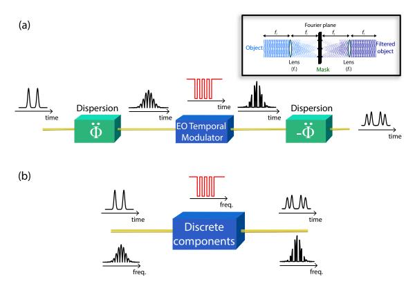
Figure 1.4 – Procedures for implementing time-domain optical linear filters: (a) inspired in spatialdomain filters, such as the one in the inset, and implemented for time-domain processing following the space-time duality, and (b) based on discrete components, e.g., ring resonators or fiber gratings. The system in (a) is time-variant, but when assuming synchronization between the modulating electrical signal and the modulated optical input, it can be considered as an optical filter.
