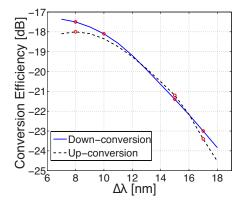
Figure 4.16 – Conversion efficiency of the XPM-based wavelength converter scheme as a function of the wavelength shift  $\Delta \lambda$ , for the cases of down-conversion (solid blue line) and up-conversion (dashed black line).
