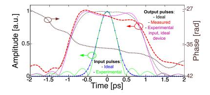
Figure 5.12 – Flat-top pulse shaper based on an FBG in transmission: Temporal signals from FTSI; ideal input pulse (crossed blue line); experimental input pulse (dotted green line); ideal output pulse (dotted-dashed black line); measured flat-top output pulse (dashed red line); output pulse obtained numerically from the experimental input pulse and the ideal grating response (solid purple line); phase of the measured output pulse (dotted line).
