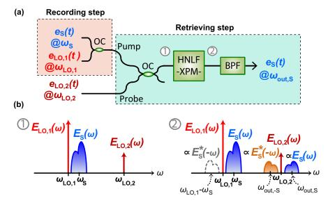
Figure 4.3 – (a) Scheme for performing time-domain holography based on XPM. In this case, both the recording and the retrieving processes are concatenated; (b) Spectra before and after the highly nonlinear fiber (HNLF): Blue components represent the information signal, the yellow component represents the conjugated signal and the dashed grey component represents the conjugated signal resulting from four wave mixing (FWM) between the pump's components.
