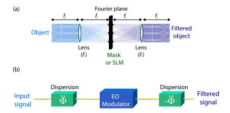
Figure 5.2 – (a) Spatial domain spectral shaping setup, and (b) time-domain spectral shaping (TDSS) setup.  $f_l$  is the focal length of the lenses.
