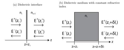
Figure B.4 – Schematic of the two elements that compose the whole grating structure for its analysis following ML-TMM.
