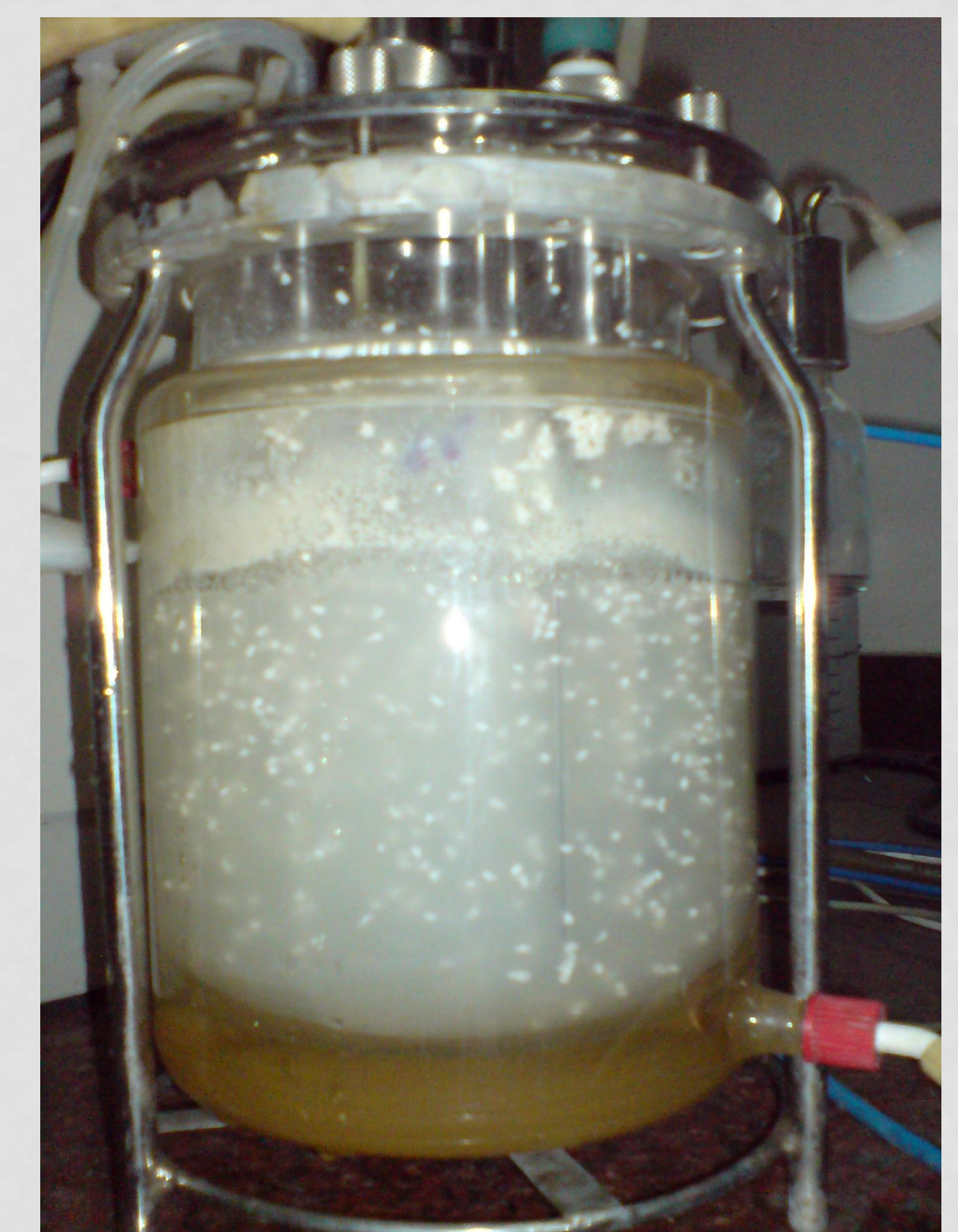
Fig. 4: Photograph of bioreactor vessel showing oil encapsulated bead suspended in aqueous media.
