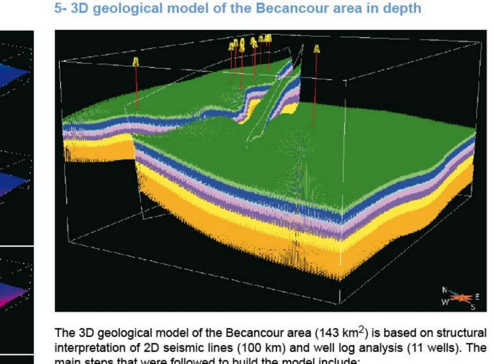
interpretation of 2D seismic lines (100 km) and well log analysis (11 wells). The main steps that were followed to build the model include: ) identification of formation tops in depth (m) after well log analysis
