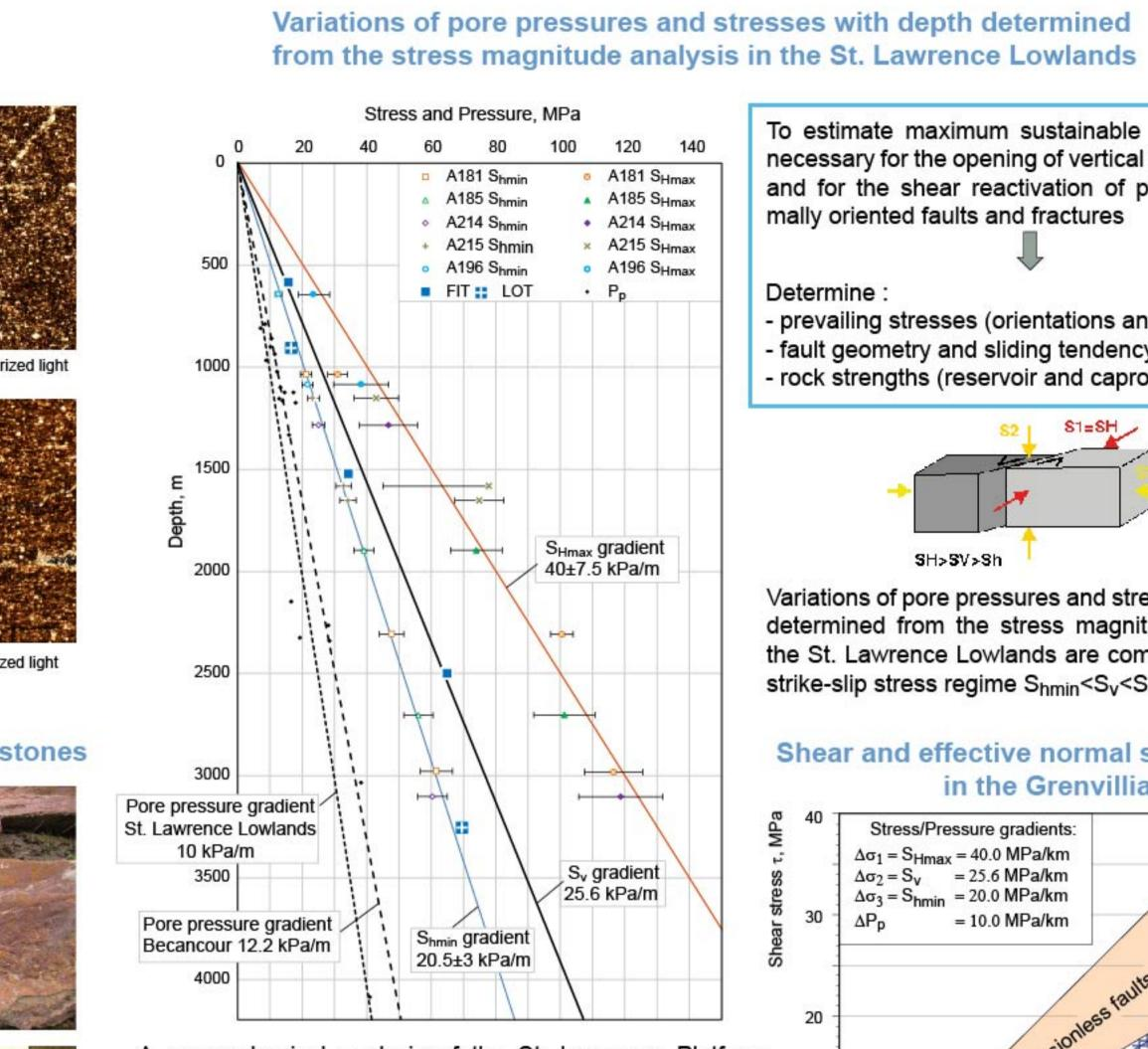
geomechanical analysis of the St. Lawrence Platform sedimentary basin provides the maximum sustainable fluid pressures for CO2 injection that will not induce tensile fracturing and shear reactivation along pre-existing fractures and faults in the caprock.
