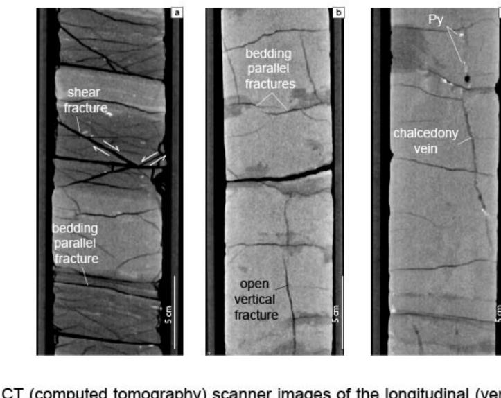
CT (computed tomography) scanner images of the longitudinal (vertical) sections of cores. Stratification is subhorizontal. Shale beds are dark gray, limestones are light gray, shaly limestones are medium gray, open fractures (filled with air) are black, the chalcedony vein is dark gray to black and sulfide mineralization (Py) is bright white spots in the vein. The bedding-parallel and inclined shear fractures are observed in Utica shales.
