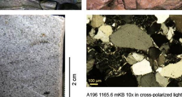
The Covey Hill is found to be the only unit with significant CO sequestration potential, since these coarse-grained poorly-sorted fluvial-deltaic quartz-feldspar sandstones are characterized by the highest porosity of 6%, matrix permeability (0.3 mD) and net pay thickness (188 m) relative to other Becancour saline aquifer units.
