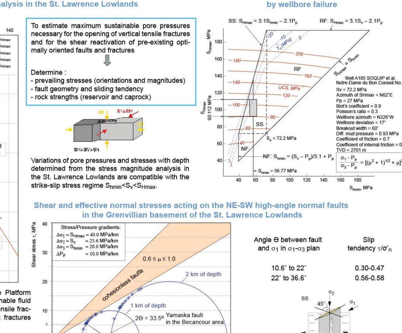
Polygon of S<sub>Hmax</sub> estimation constrained
