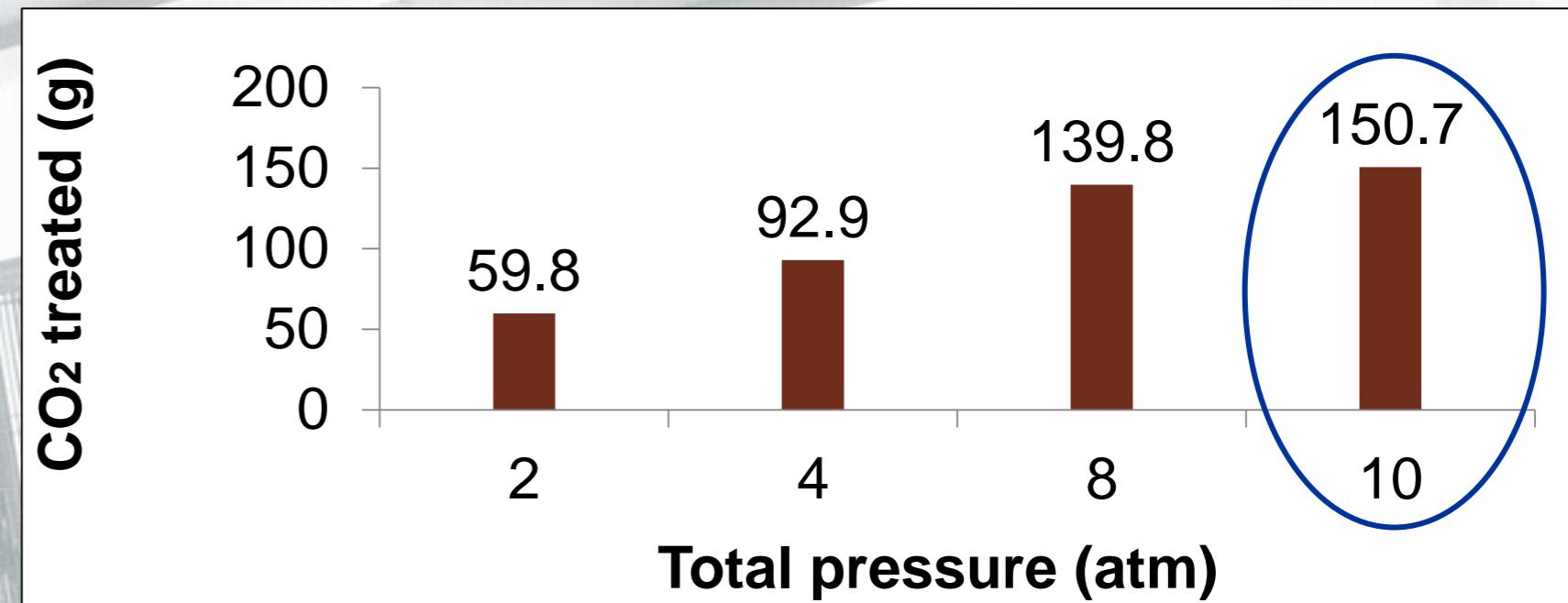
Cumulative mass of CO<sub>2</sub> treated using Sample (A)
