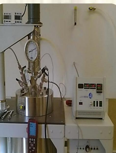
Pulp & Gas in a stirred reactor
