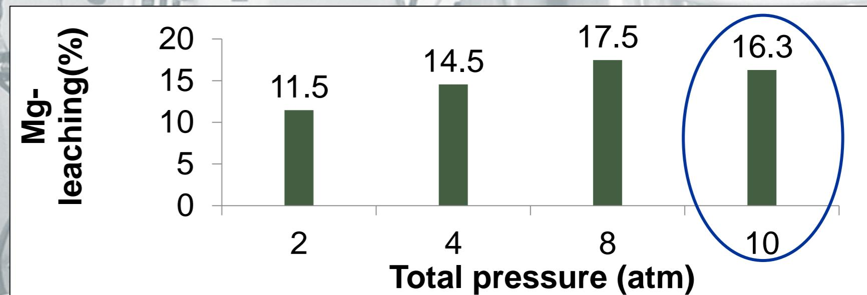
Cumulative rate of leached magnesium using Sample (A)
