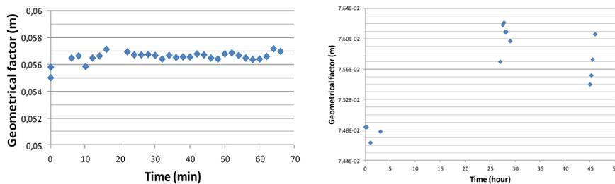
Fig.2 : (a) The geometrical factor measured with a KCl solution of a known conductivity as a function of time. The value seems stable over a one hour period with an error of about 1%. (b) The geometrical factor measured over a 3 days period. After a day, we notice and increase of 2% associated with a slight corrosion on the electrodes that then remain stable.
