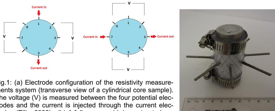
Fig.1: (a) Electrode configuration of the resistivity measurements system (transverse view of a cylindrical core sample). The voltage (V) is measured between the four potential electrodes and the current is injected through the current electrodes (Ellis, 2008). (b) A fully prepared brine saturated porous ceramic sample.
