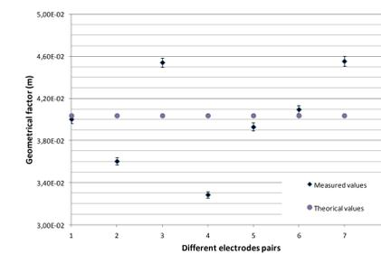
Fig.5 : The geometrical factor for the eight possible electrodes pairs. We observe an important difference with the theoretical values. By averaging the different pairs, a mean value of :  $(3,99 \pm 0,04) \cdot 10^{-2} \text{ m}$  is obtained. A difference of about 1% with the theoretical value.
