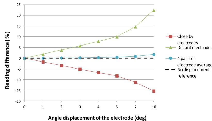
Fig.4 : Modeled difference on the voltage between the pairs of electrodes affected by the angular displacement of one of the four potential electrodes.
