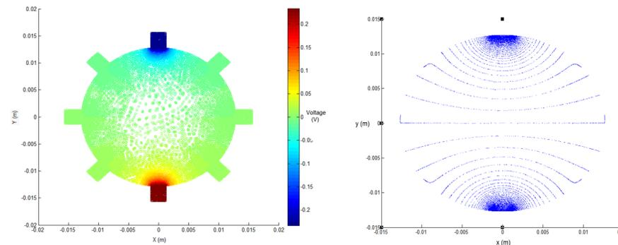
Fig.3 : (a) Electric potential modeled within the sample and the electrodes. (b) Equipotential lines within the sample. Each level correspond to 1% of the total voltage.
