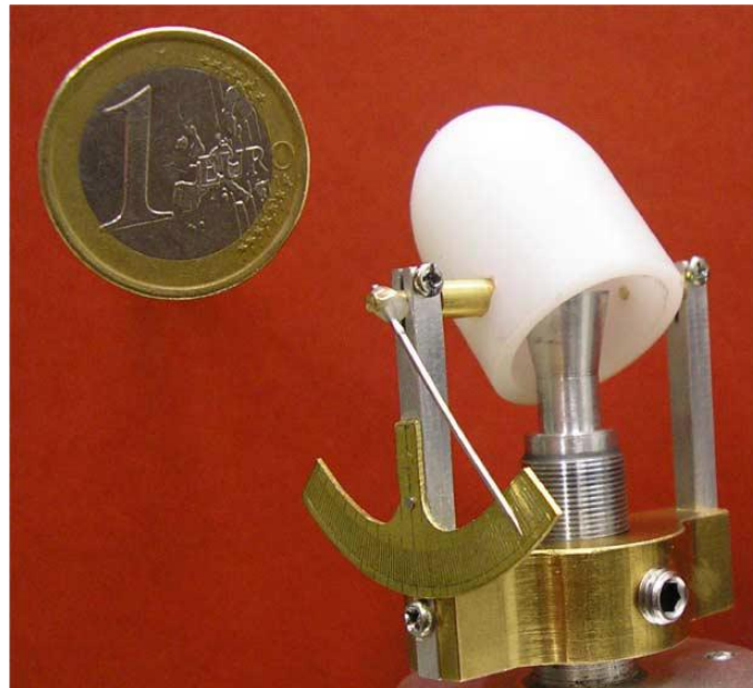
Figure 1-5: Dielectric lens antenna integrated by horn antenna for mechanically beam tilting at 60 GHz [5].
