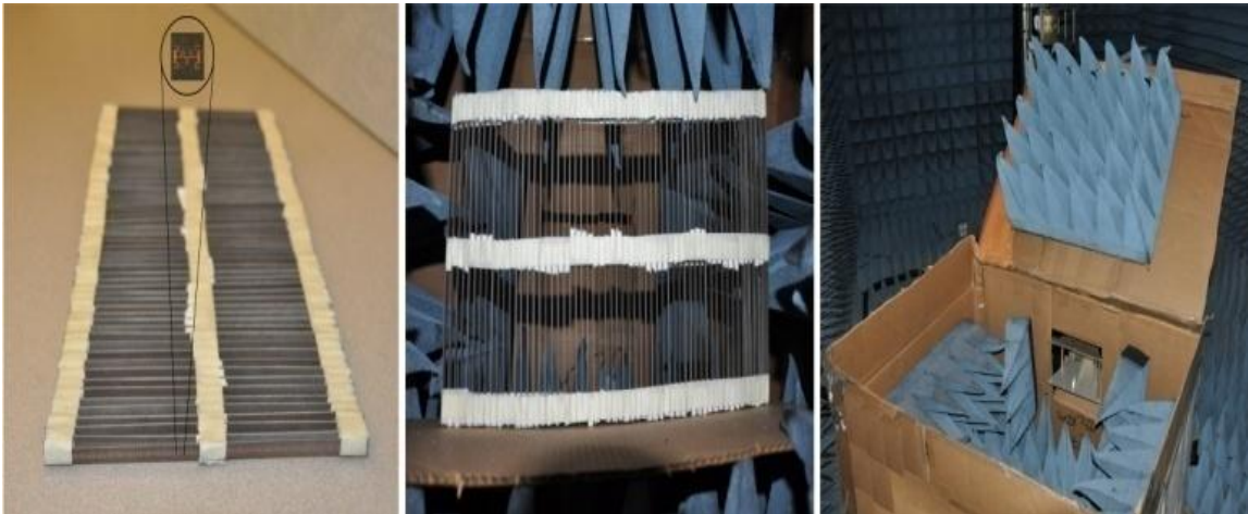
Figure 2-3: Measurement setup for acquiring the S -parameters of the unit-cell array.
