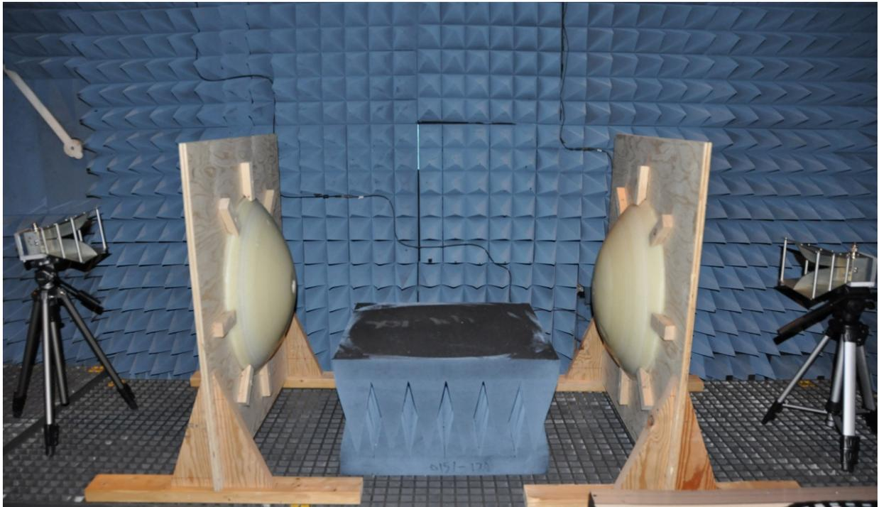
Fig. 8.6. Paraffin dielectric lenses used in the measurement setup.
