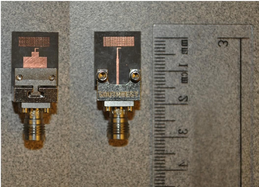
Fig. 7.22 The fabricated prototype at millimeter waves.
