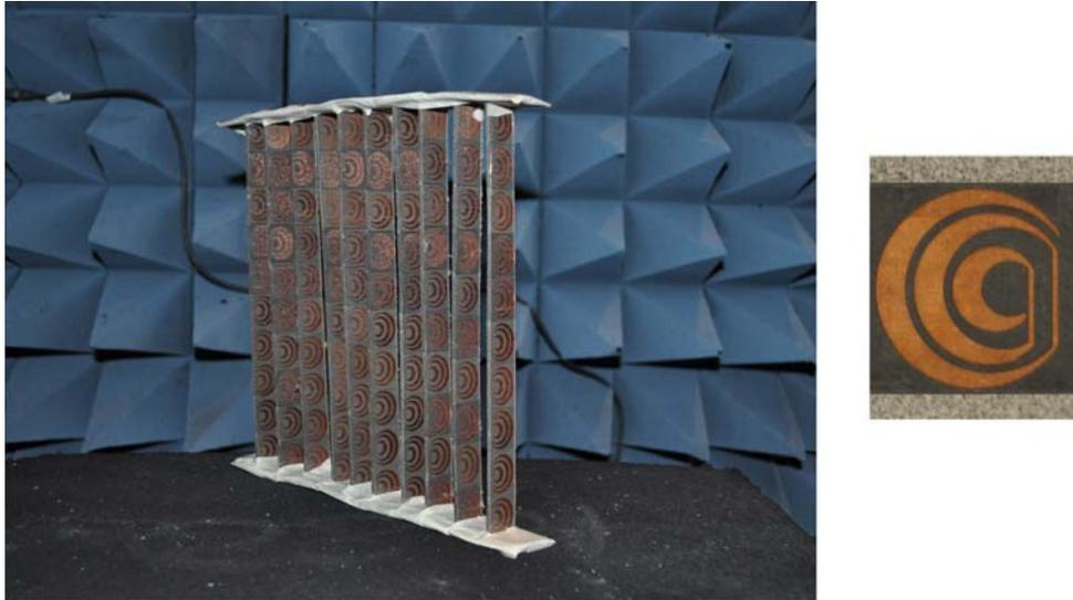
Fig. 5.17. The fabricated crescent-shaped prototype.
