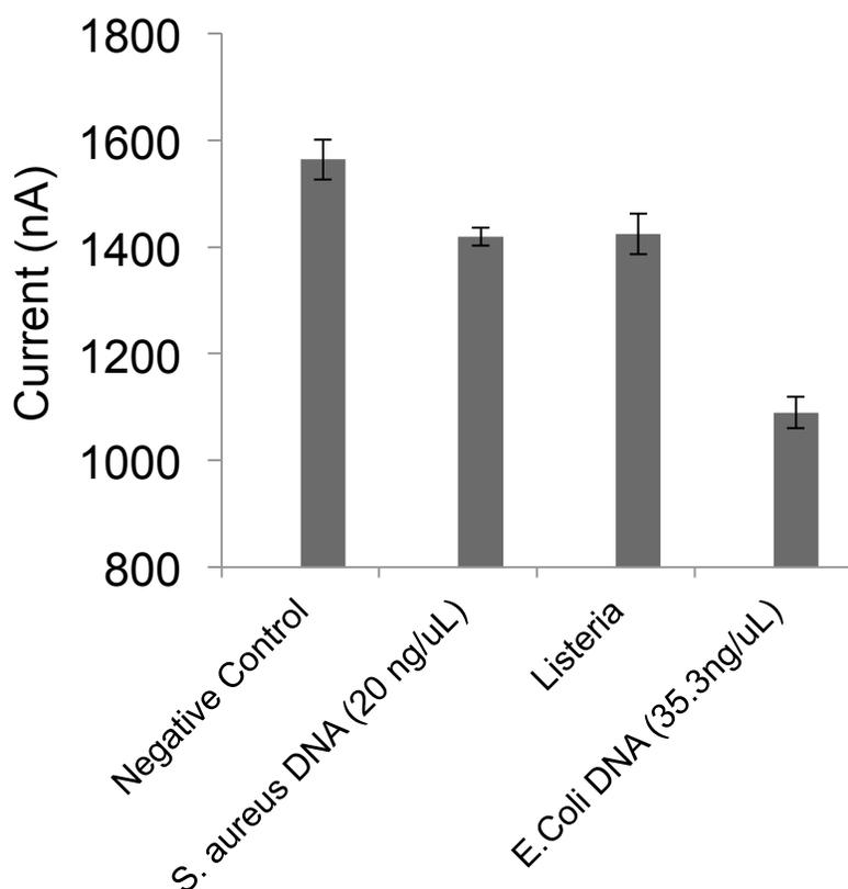
**Fig. 3.6.** Cross reactivity test for the E.coli primes in the chip. Negative control contained of water with no E.coli DNA template. Due to existence of DNA and binding to redox molecule with its minor groove there is a small drop in the anodic oxidation peak current. The major drop is distinguishable between the E.coli DNA sample and other bacteria.
