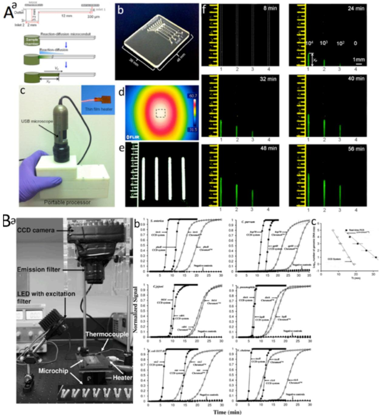
Figure A1.6 LAMP Microfluidic chips integrated with CCD Camera. (A) The Nucleometer. (a) Schematic of nucleometer, which consists of reaction chamber and a microconduit where reaction-diffusion takes place. NA template is amplified and diffused
