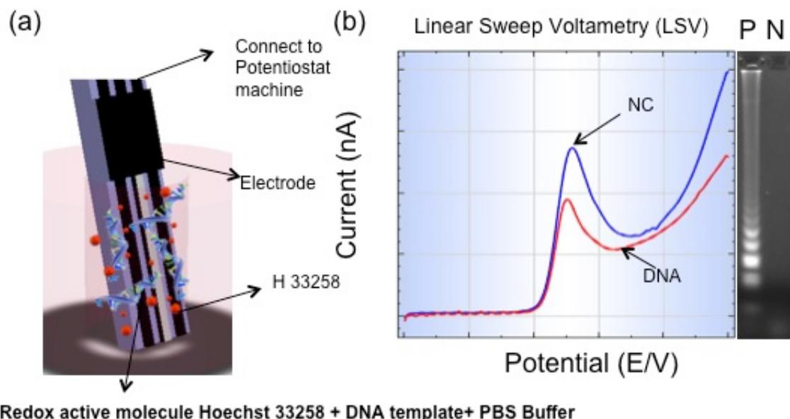
**Fig. 3.2** Schematic of the electrochemical detection in the electrode chamber on microfluidic chip. (a) The redox active molecule Hoechst 33258 binds to the DNA minor groove, which causes the major reduction of electron on the surface of the electrode. (b) LSV is used as an electrochemical method demonstrating major drop in DNA detection in comparison with negative control sample. Gel electrophoresis image of negative sample, N, and positive sample, P, approves the DNA amplification.
