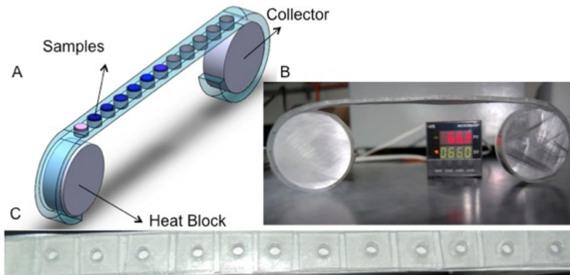
**Fig 4.1** Overview of Cassette device and its components. (A) Schematic of the Cassette. Cassette consists of two aluminum reels to provide and collect samples, a heat controller and heater to provide precise temperature for amplification and the flexible substrate where the chambers are fabricated. (B) Image of the flexible substrate. (C) Image of the flexible substrate.
