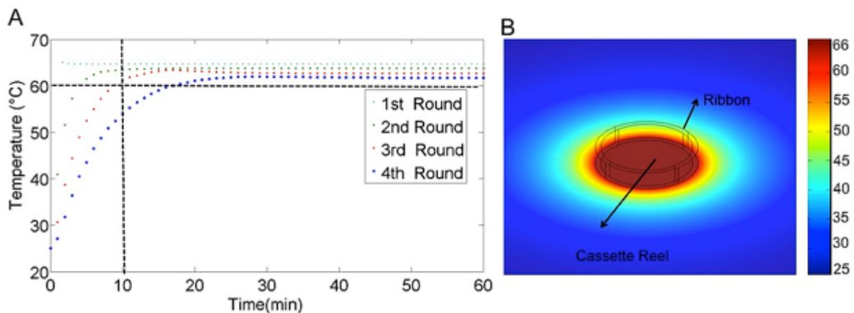
**Fig 4.5** Numerical heat-transfer simulation around the Cassette reel and ribbon. (A) 3D time-dependent heat transfer simulation has been implemented for different rounds of ribbons around the heater reel. The heater can provide minimum  $60^\circ\text{C}$  for at least 50 min, which requires for amplification and colorimetric detection. (B) Temperature profile around the heater and ribbon.
