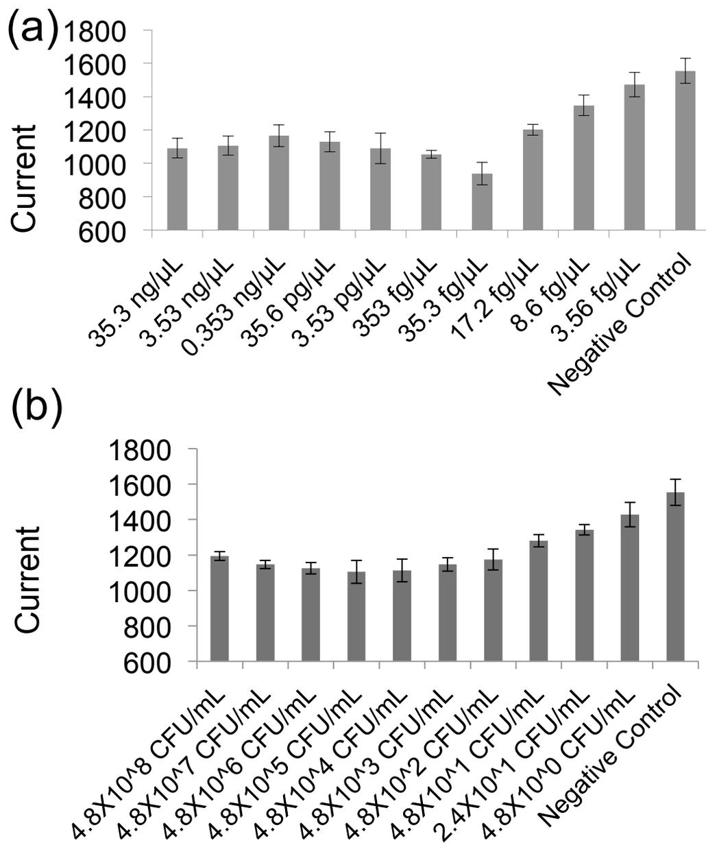
**Fig. 3.3** Electrochemical detection of *E.coli* in the microfluidic chip (a) Maximum peak current in LSV for different extracted *E.coli* DNA concentration. The detection limit on the chip is 8.6 fg/μL. (b) Maximum peak current in LSV for different bacteria concentration. The detection limit for the bacteria detection on chip is 24 CFU/ml.
