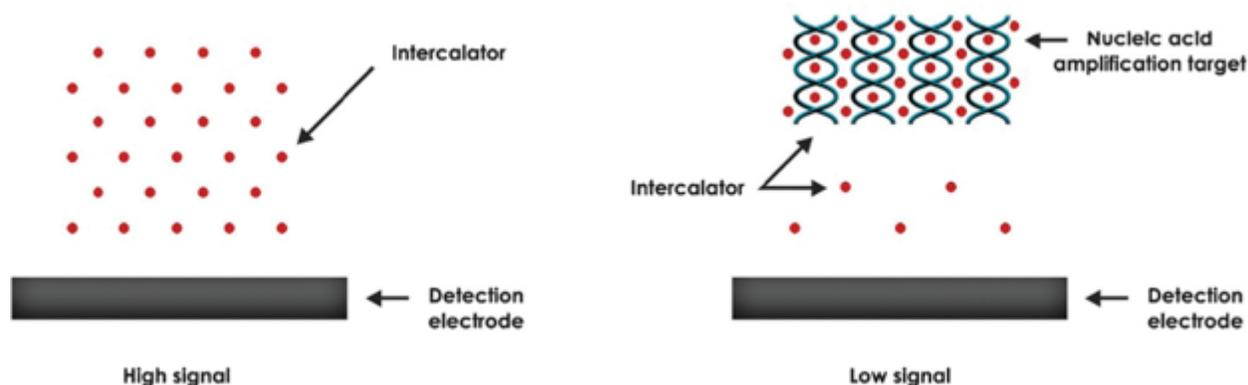
**Figure 2.9.** Schematic of electrochemical detection of NA. When NA is not present, the signal is high due to all redox intercalator molecule are free to react on surface of electrode. When NA is present, the signal is low as significant amount of redox binds with NA[116].
