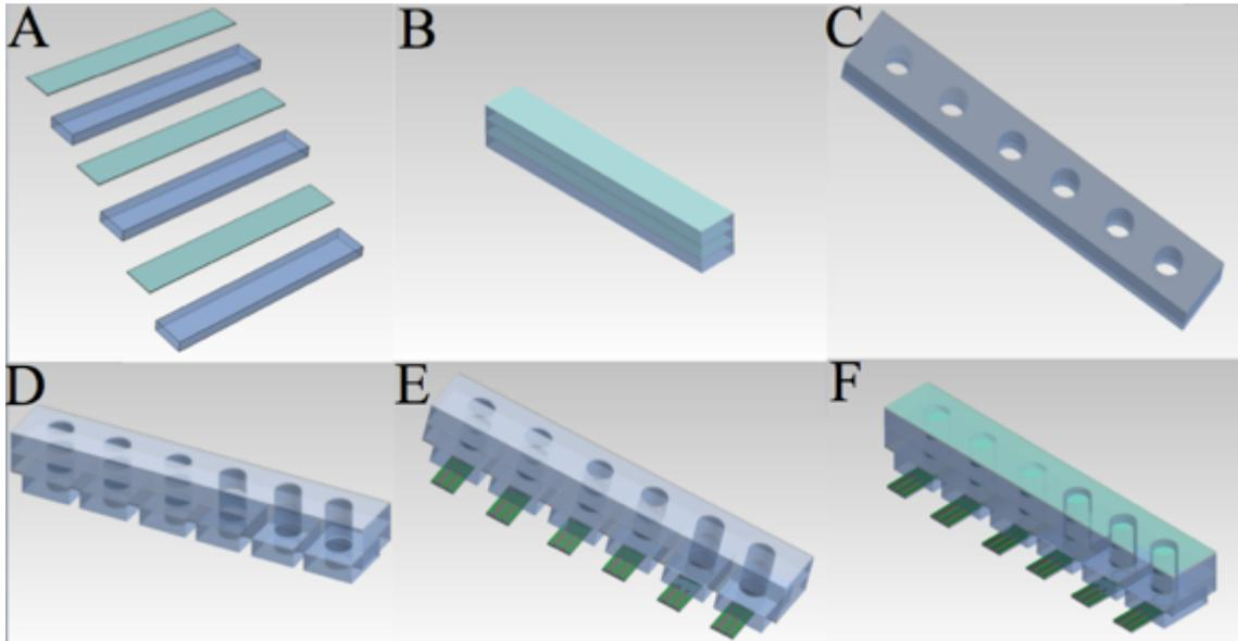
**Fig A3.1:** Schematic of the fabrication process. (A) Flexible substrate consists of three layers of polyethylene ribbons, which was attached using double-sided tape. (B) The layers were attached on top of each other. (C) Punching the substrate to form reservoirs. (D) Removing the redundant to enhance bending and flexibility. (E) Attaching the flexible carbon electrode at the bottom of each reservoir. (F) Apply the samples and cover the reservoirs using the tape.
