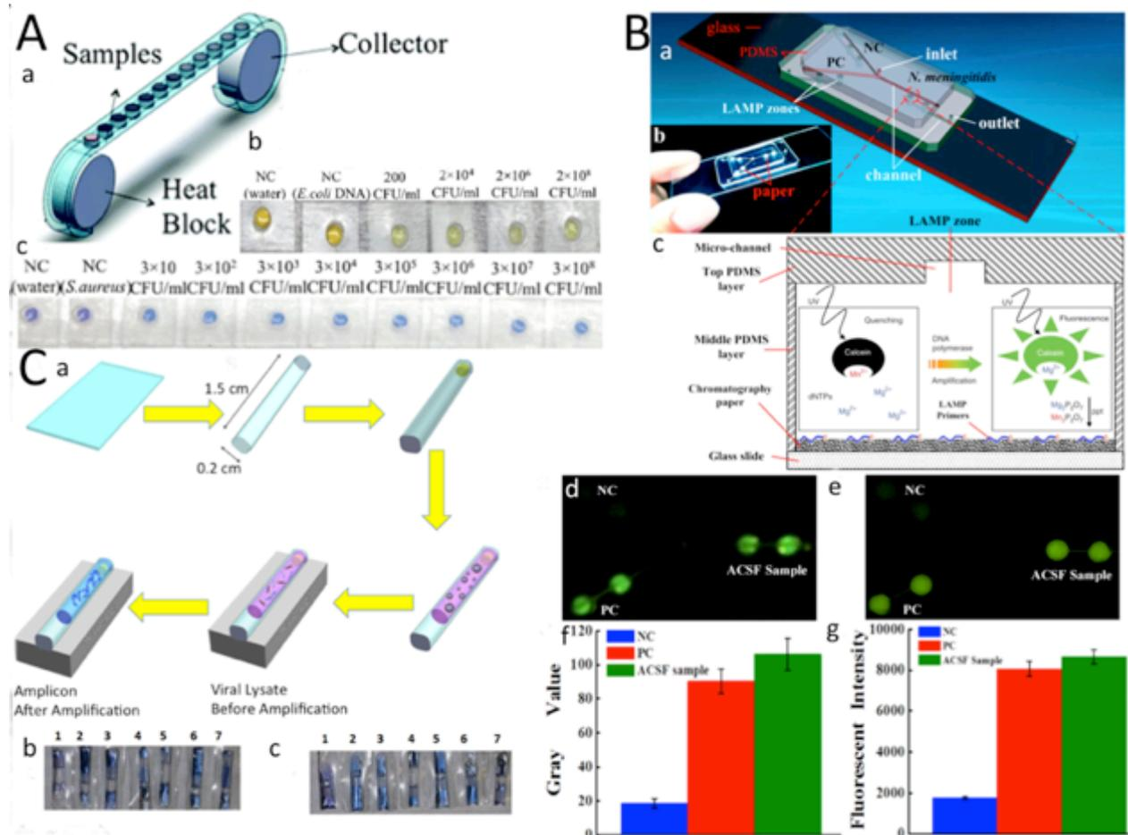
Figure A1.1 LOC devices based on LAMP amplification and colorimetric detection (A) (a) Cassette device for high throughput bacteria detection, which has the array of chamber on flexible ribbon. (b) *S.aureus* pathogen was detected using Calcein with the LOD of 200 CFU/ml. (c) *E.coli* bacteria was detected using HNB dye with LOD of 100 CFU/ml.
