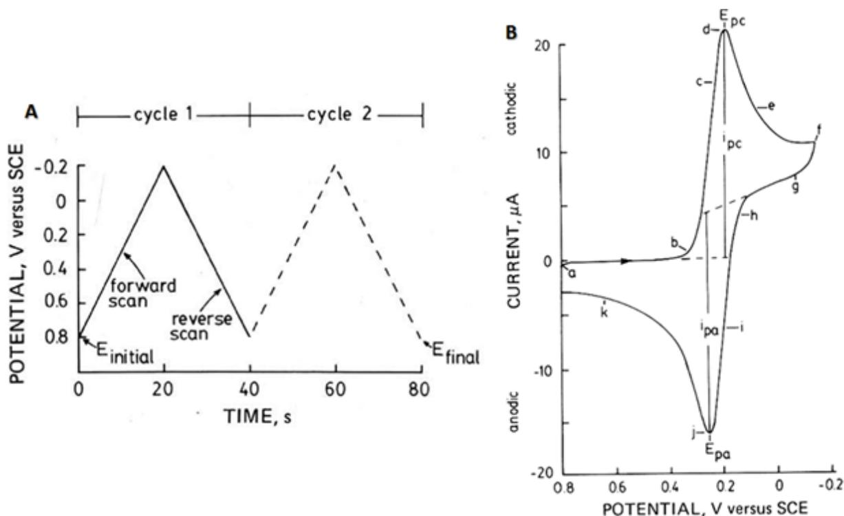
Figure 2.5 Schematic diagram of CV. (A) applied voltage. (B) CV diagram[98].
