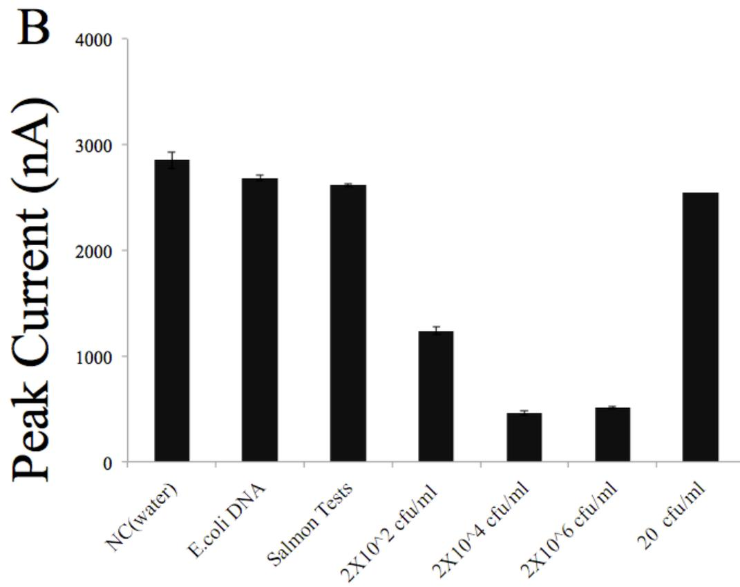
**Fig 5.5** End-point detection of bacteria at different concentration and cross-reactivity tests. (A) 30 CFU/mL of *E.coli* bacteria (B) 200 CFU/mL of *S.aureus* bacteria were detected after 50 min amplification time. The cross-reactivity test were performed for *E.coli* detection (A) using *S.aureus* DNA and *Salmon testes* DNA and (B) using *E.coli* DNA, *Salmon testes* DNA which reflect the fact that the assays are highly specific to the amplified targets.
