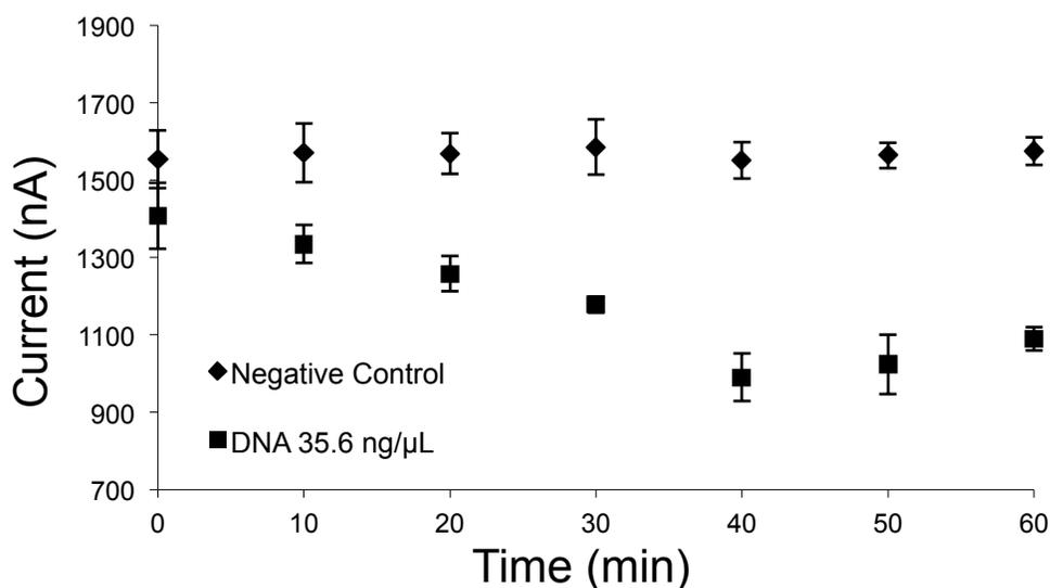
**Fig. 3.4** Time optimization of DNA sample on the chip. The (◆) illustrates the negative control and the (■) data represents the DNA sample. The chip detects the target DNA in 20 minutes. The DNA concentration is 35.6 ng/μL. Each measurement is carried out in separate chip, which reflects the reproducibility and stability of data.
