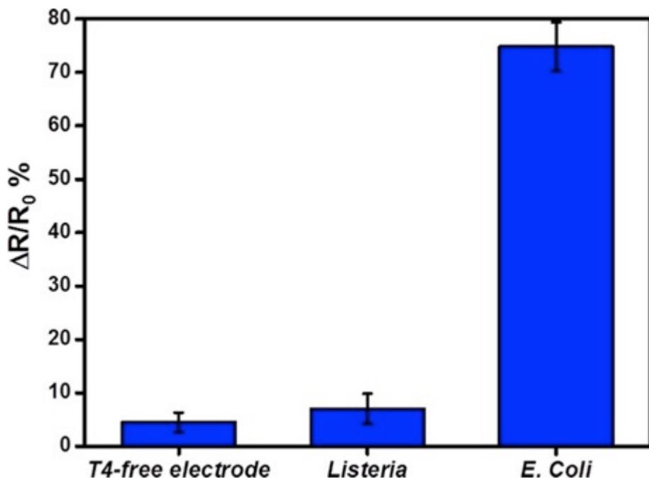
Fig 6.4 Figure 4. T4-bacteriophage biosensors selectivity against *Listeria* cells.
