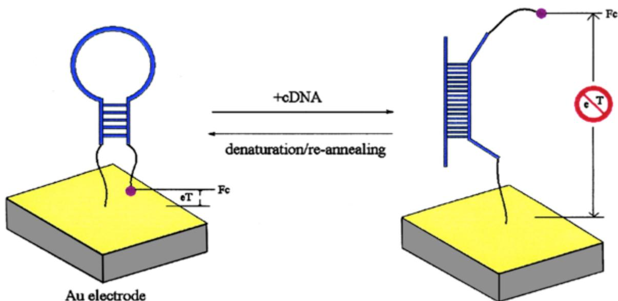
**Figure 2.7** Schematic of electrochemical DNA hybridization detection based on molecular beacon. The hybridization changes the distance of the label from the surface of electrode (Reproduced with the permission from [113]).
