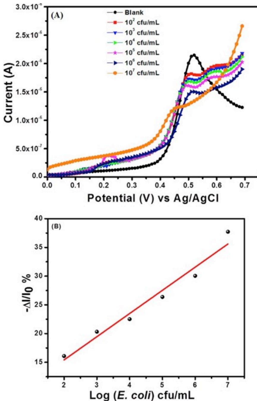
Fig 6.6 (A) Linear Sweep voltammetry (LSV) monitoring the LAMP amplification of the *Tuf* gene target. (B) Calibration curve of the LAMP assay.
