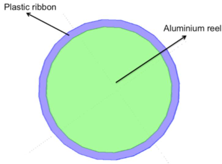
Figure A2.1 Schematic of the geometry of reel for heat transfersimulation.
