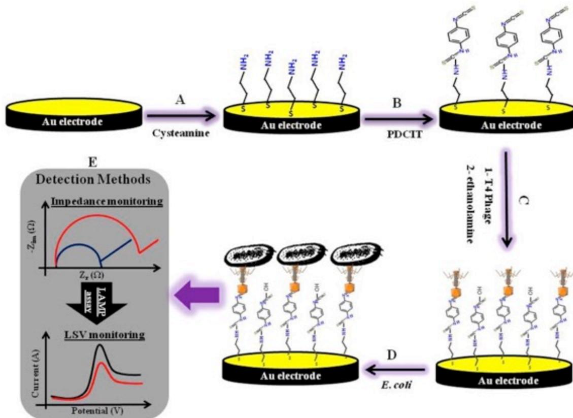
**Fig 6.1** Schematic representation of the T4-bacteriophage biosensors. (A) Cysteamine-assembly on gold electrode. (B) Activation with 1,4-dithiocyanate (PDICT) cross-linker. (C) Immobilization of the T4 phage and blocking with ethanolamine. (D) Capturing of the *E. coli* cells. (E) Detection method for *E. coli* based on the impedimetric/LAMP dual-response.
