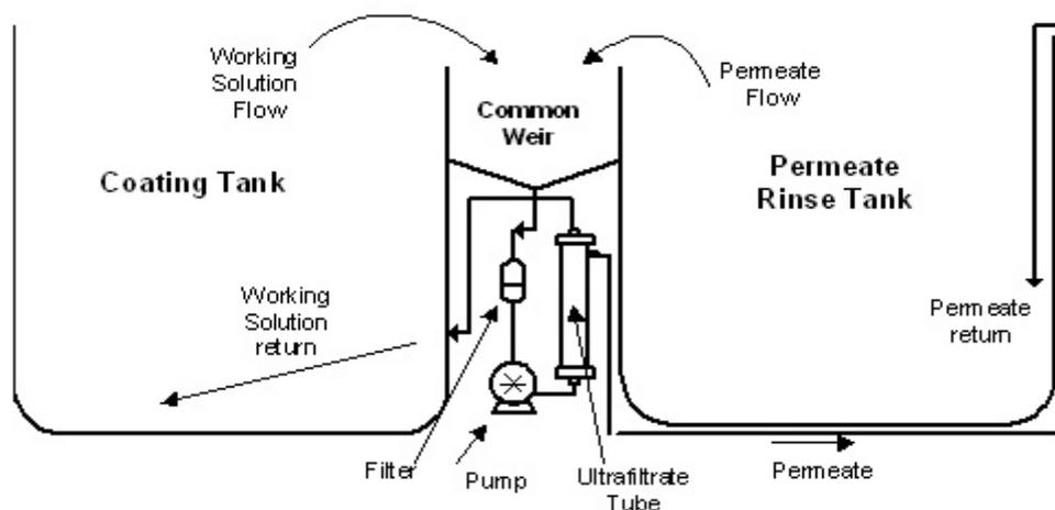
Figure 2.9. Schematic of the ultrafiltration system.
