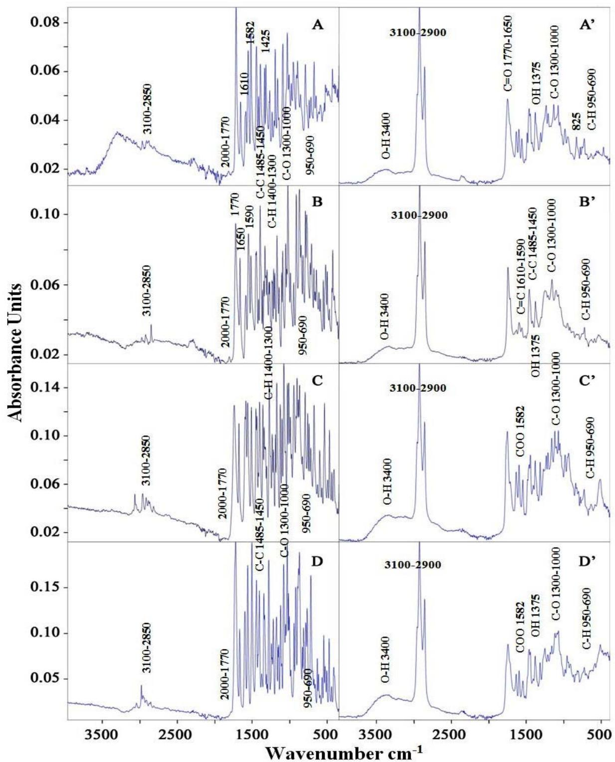
Figure 6.4. Fourier transform infrared spectroscopy (FTIR) spectra of the aflatoxins AFB1 (A), AFB2 (B), AFG1 (C), AFG2 (D) and the purified laccase-catalyzed end products of aflatoxins AFB1 (A'), AFB2 (B'), AFG1 (C'), AFG2 (D').
