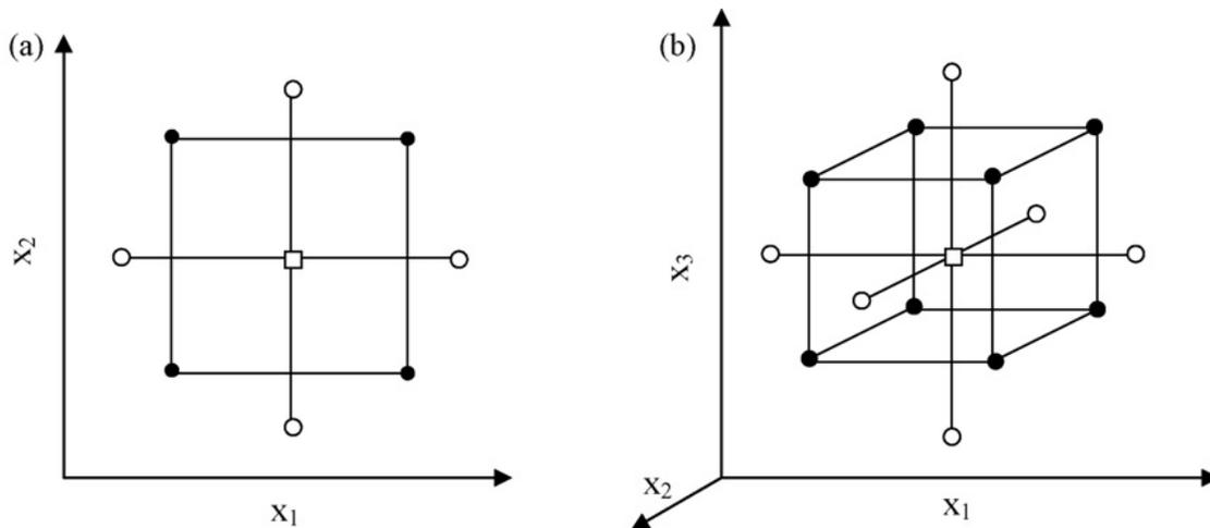
Figure 2.4. The representations of the central composite designs for (a) two- and (b) three-variables optimization (Bezerra *et al.*, 2008).
