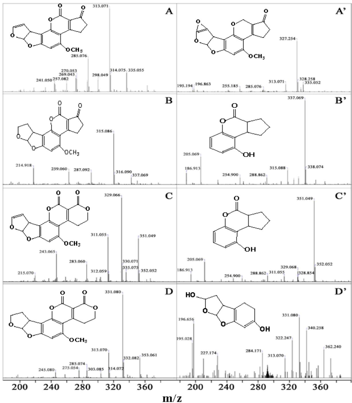
Figure 6.5. Liquid chromatography/mass spectrometry (LC/MS) chromatograms of the aflatoxins, AFB<sub>1</sub> (A), AFB<sub>2</sub> (B), AFG<sub>1</sub> (C), AFG<sub>2</sub> (D) and the purified laccase-catalyzed end product of aflatoxins AFB<sub>1</sub> (A'), AFB<sub>2</sub> (B'), AFG<sub>1</sub> (C'), AFG<sub>2</sub> (D').
