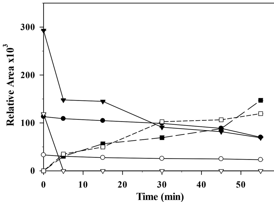
Figure 6.1. Degradation of aflatoxins, AFB1 (●), AFB2 (○), AFG1 (▼) and AFG2 (▽), from *Aspergillus parasiticus*, with the partial purified laccase from *Coriolus hirsutus* over 55 min. The symbols ■ & □ correspond to the formation of the enzymatic degradation products during laccase treatment.
