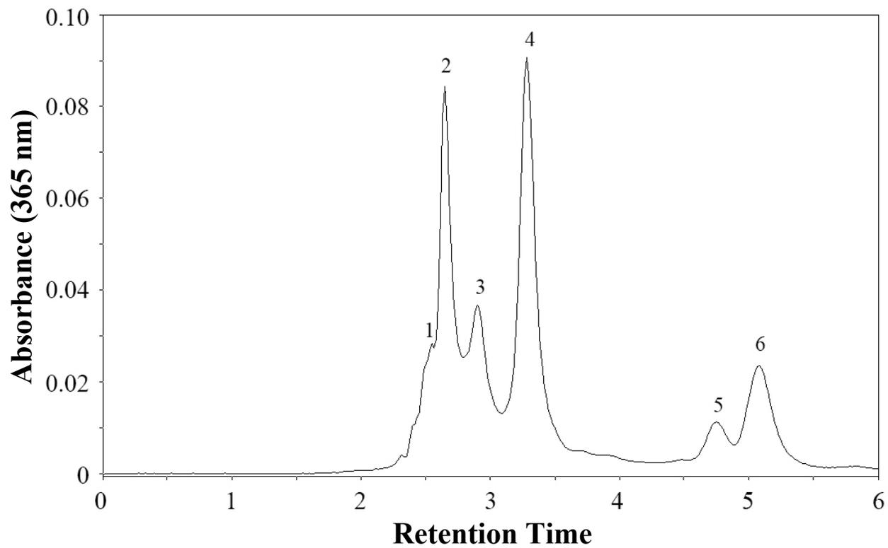
Figure 3.3. HPLC chromatogram of the aflatoxins from *Aspergillus parasiticus* at 365 nm, using an allsphere column C18 thermostated at 50°C, with a mix of methanol/water (60/40; v/v) as mobile phase, and a flow rate of 1 mL/min.
