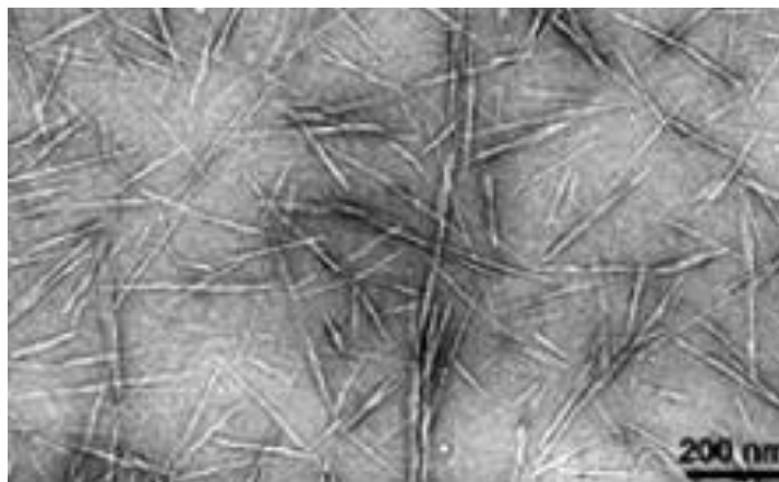
Figure -1.4: TEM image of highly anionic cellulose nanocrystals adapted from Habibi et al.
