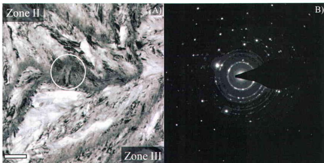
Figure 18. A) Bright field image of the end of the dendritic region (Zone II) and the beginning of the layered structure (Zone III). Scale bar: 500 nm. B) SAED pattern from the area surrounded by the white circle in A).
