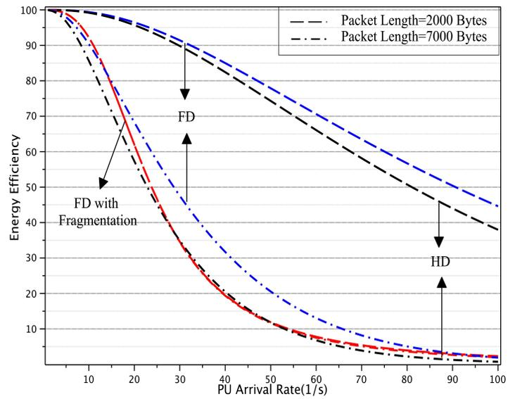
Figure 4.6: Energy efficiency  $\rho$  for data lengths of 2000 and 7000 bytes: HD vs. FD with or without fragmentation.
