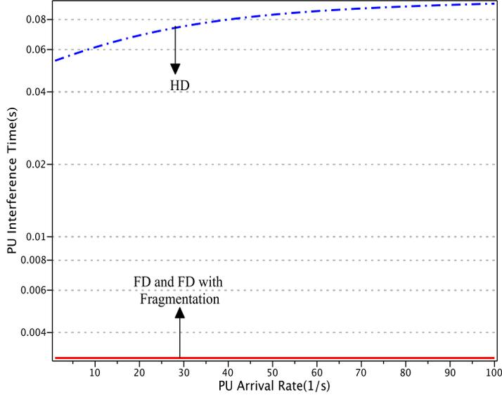
Figure 4.3: PU interference time,  $T_{int}$ , in HD and FD systems.
