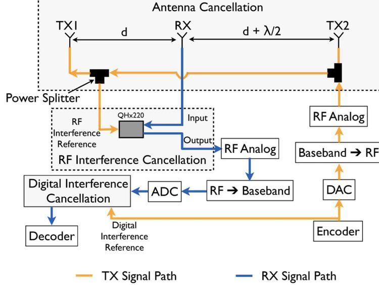
Figure 3.3: Detailed diagram of FD transceiver equipped with three methods of cancellation [2].
