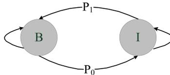
Figure 2.2: Two-state transition diagram for modeling the dynamic behavior of primary users over a channel.
