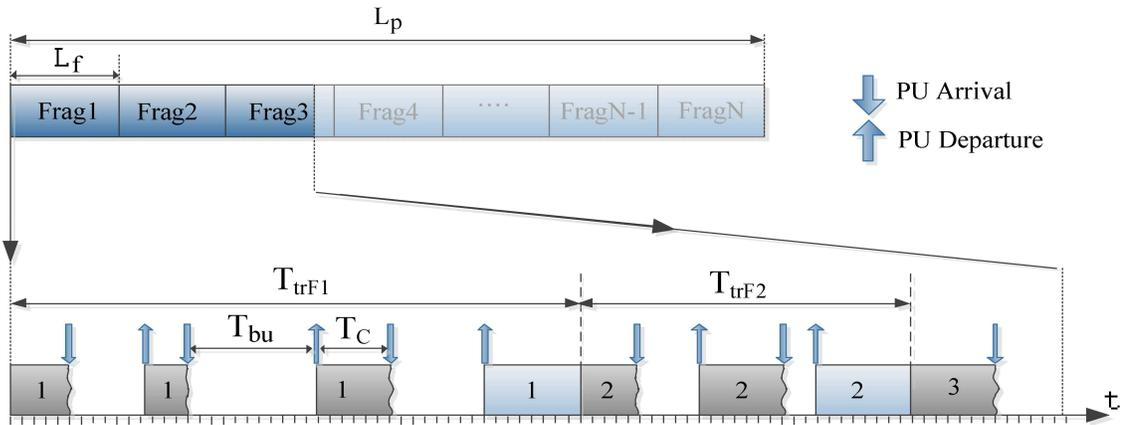
Figure 4.1: Packet fragmentation and its transmission on the channel.
