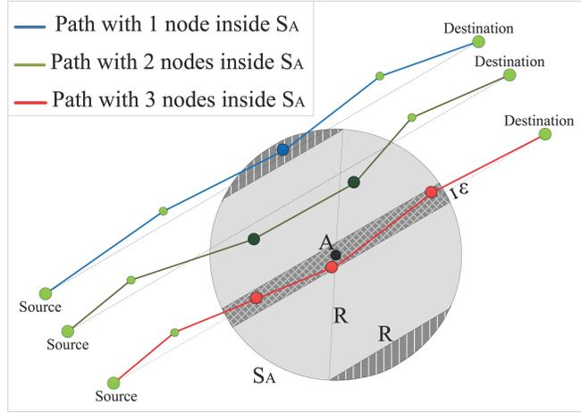
Figure 5.5: Node A different placement to a path and hearing one, two or three nodes of that path.
