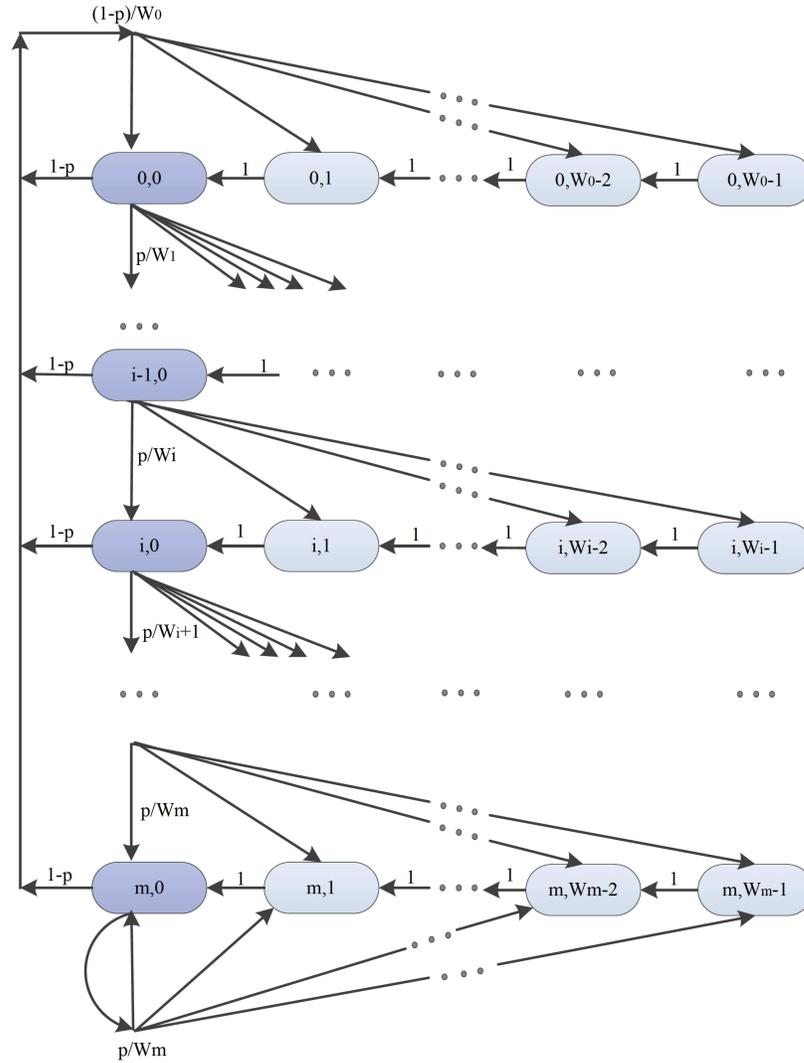
Figure 2.4: Proposed 2-D DTMC in [7] for the modeling of the DCF mechanism.
