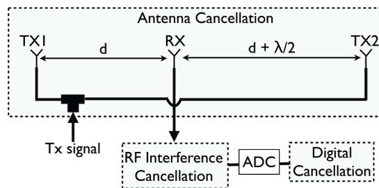
Figure 3.1: Three methods of self-interference cancellation in the FD transceiver [1].
