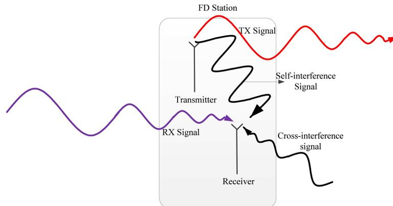
Figure 1.1: Self-interference in a full-duplex transmitter.
