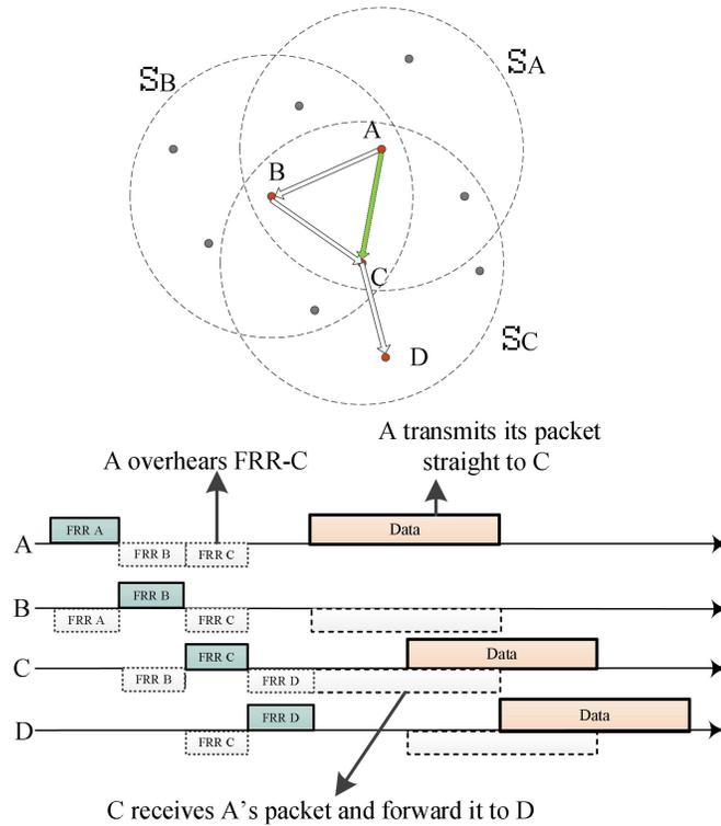
Figure 5.2: The ability of the proposed protocol to refine the route assigned by the network layer.
