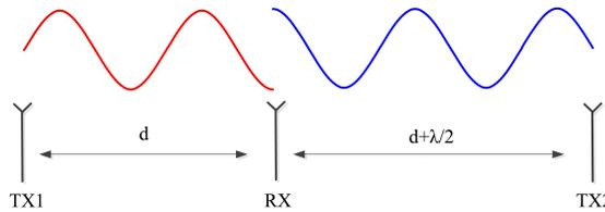
Figure 3.2: Transmitter and receiver antennas arrangement producing null point [2].
