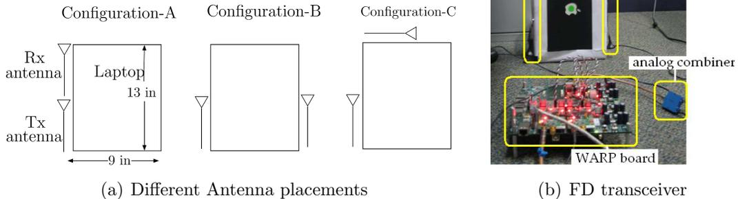
Figure 3.4: OFDM FD transceiver and different antenna placements for this system [3].
