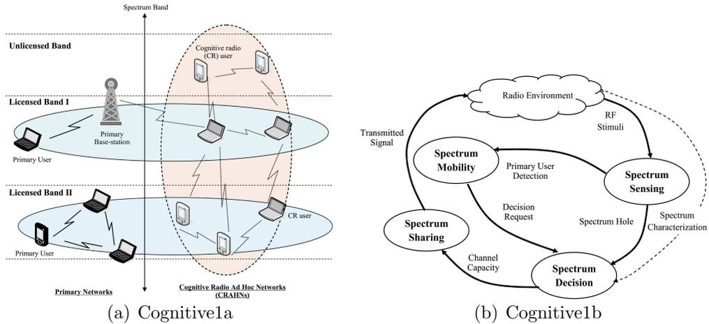
Figure 2.1: The CRAHN architecture and the cognitive radio cycle are shown in (a) and (b), respectively [5].
