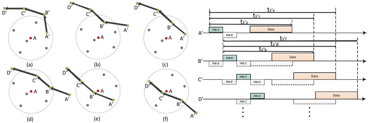
Figure 5.4: Different placement possibilities of a hearer node ( $A$ ) w.r.t. a forwarding path.
