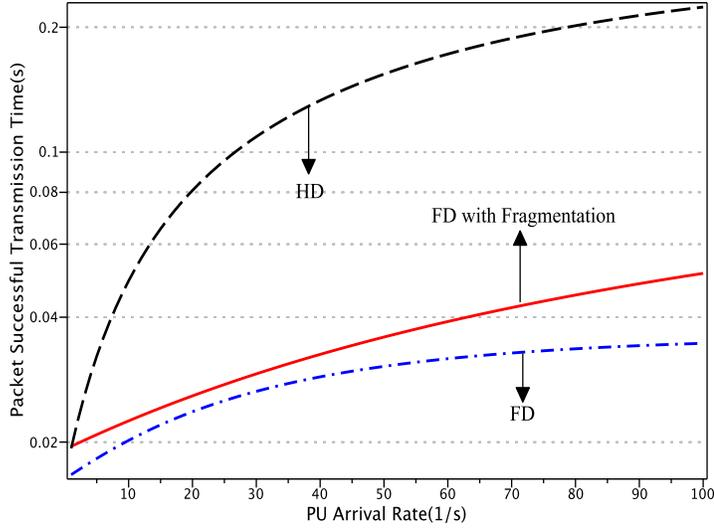
Figure 4.5: Packet successful transmission time  $\bar{T}_{tr}$ : HD vs. FD with or without fragmentation.
