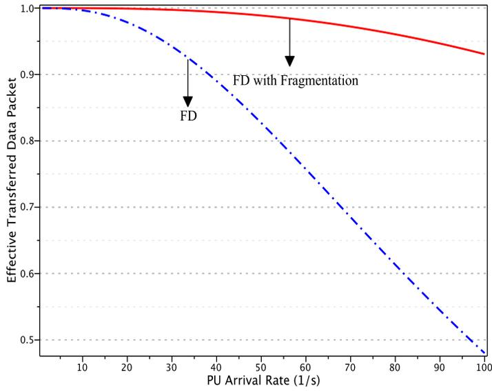
Figure 4.4: Average data fraction that is successfully transmitted over the channel before the first PU arrival,  $\bar{F}_T$ .
