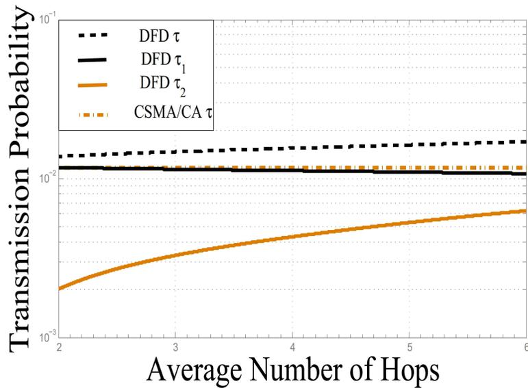
Figure 5.8: Comparison of DFD-MAC transmission probabilities ( $\tau_1$ ,  $\tau_2$ ,  $\tau$ ) with the transmission probability of CSMA/CA.
