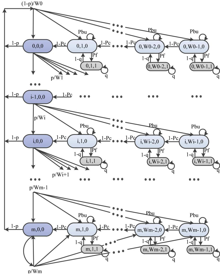
Figure 5.3: The proposed DTMC characterizing the dynamics of the DFD-MAC protocol at each node.
