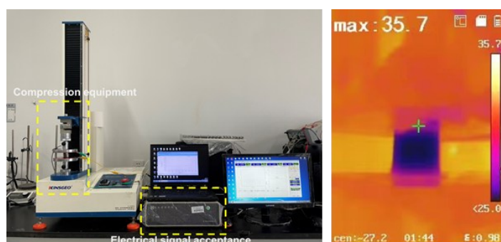
Figure 2.1 Real and thermographic images of the hydrogel's mechanics-electric conversion testing process.
