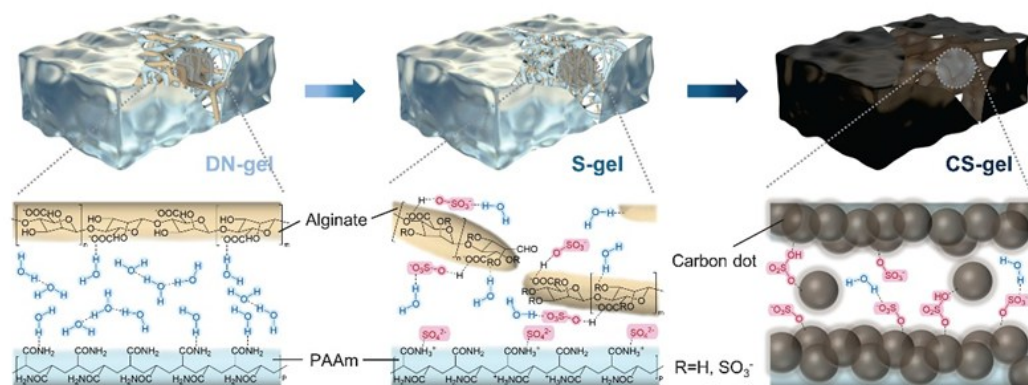
Figure 6.2 Schematic illustration of in situ formation of a carbon dot barrier on the surface of PAM hydrogel.[234]
