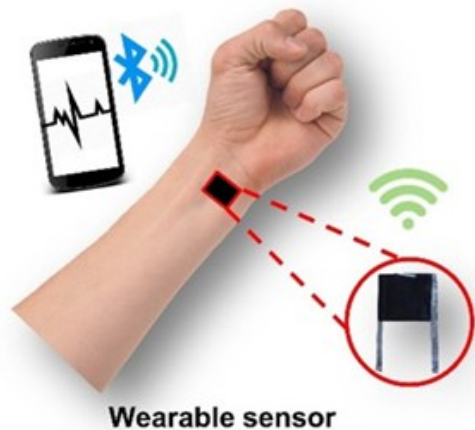
Figure 1.2 Real-time acquisition and wireless transmission of subtle pulse signals by a wearable pressure sensor. [13]
