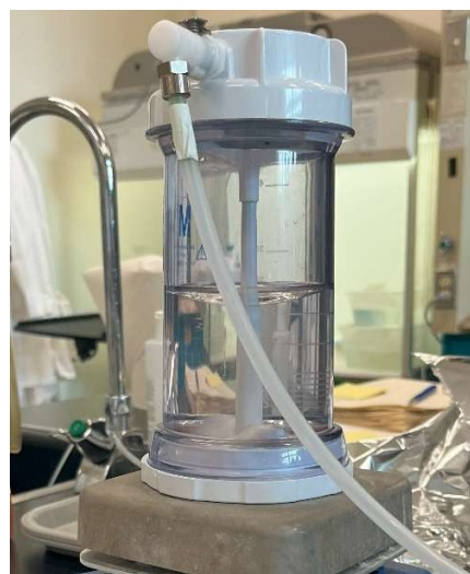
Figure 6 Cellule de filtration
