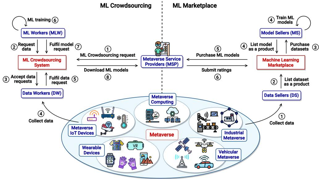
Figure 4.1: Overview of the metaverse and the architecture of MetaAICM with two operation modes, namely crowdsourcing system and decentralized marketplace.
