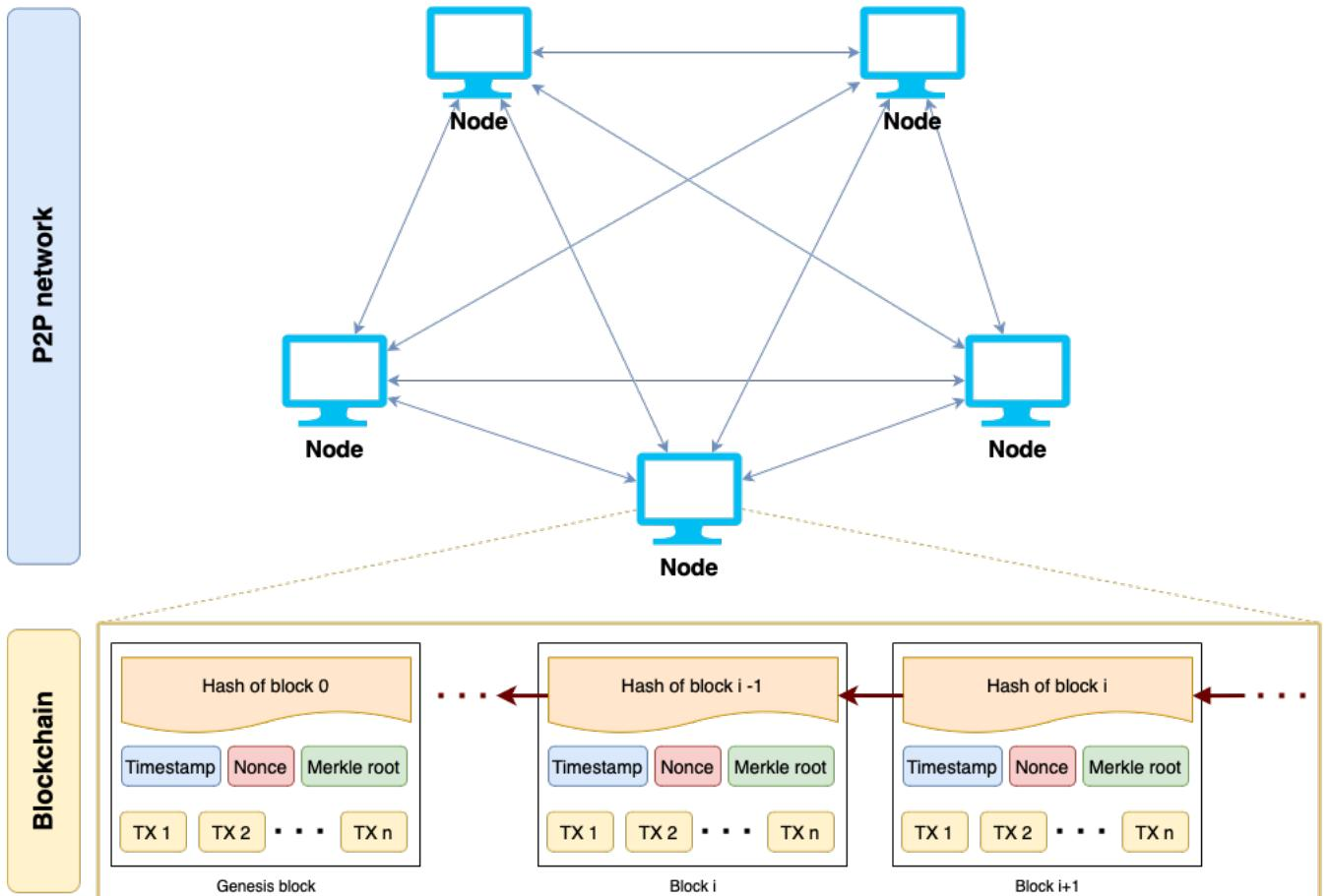
Figure 3.1: Architecture of a blockchain, consisting of a continuous sequence of blocks.
