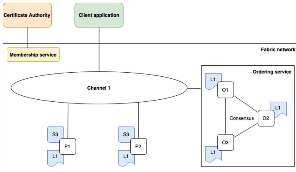
Figure 3.5: Hyperledger Fabric architecture featuring a channel (Channel 1) that includes smart contract (S3) and ledger (L1). The architecture shows five participants: peer nodes (P1, P2) and orderer nodes (O1, O2, O3).
