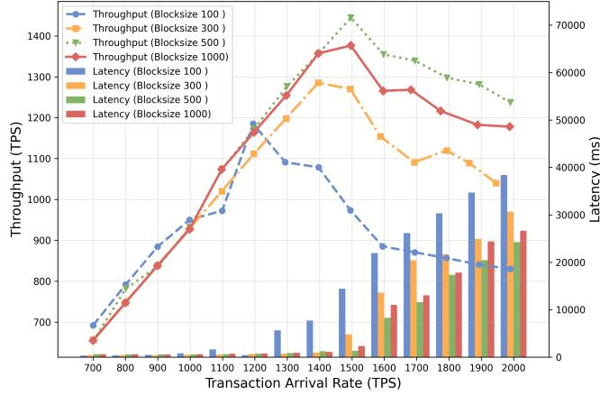
Figure 4.6: Blockchain performance as the block size varies from 100 to 1000 transactions per block.
