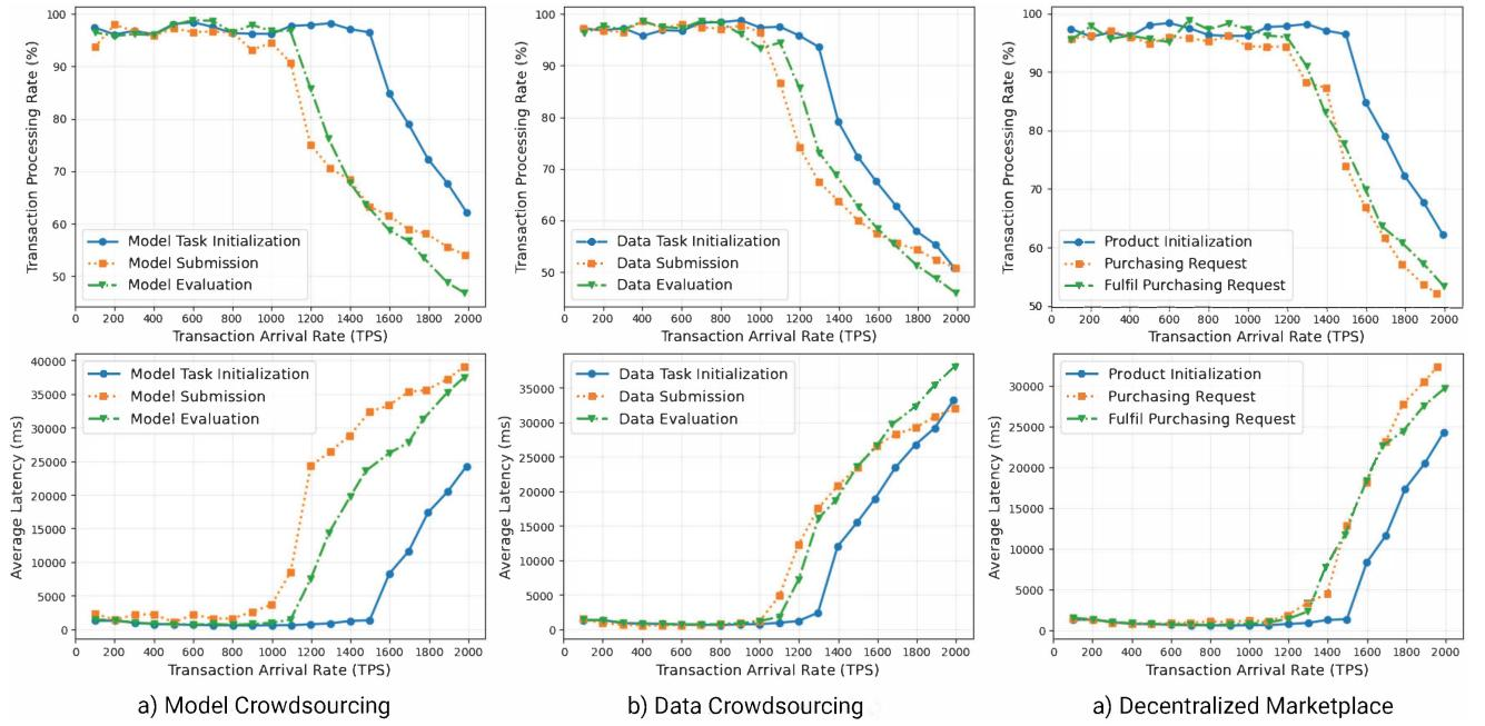
**Figure 4.5: Performance of smart contract’s functions under different workloads, ranging from 100 to 2000 TPS.**
