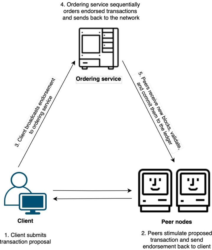
**Figure 3.6: Hyperledger Fabric Transaction Flow**
