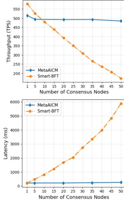
Figure 4.7: Performance of MetaAICM’s consensus compared to BFT-Smart when the committee size varies from 1 to 50.
