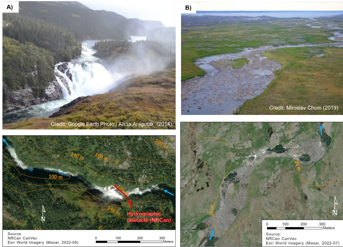
Figure 7 Examples of the obstacles identification with pictures, topographic data and satellite basemap imagery: A) Impassable waterfalls on the Clearwater River (southern Hudson Bay); B) Potential impassable low water level section on the Curot River (southern Ungava Bay)
