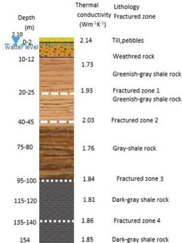
Figure 3.6 Hydrothermostratigraphic log of the 1UBHE at the INRS experimental site.
