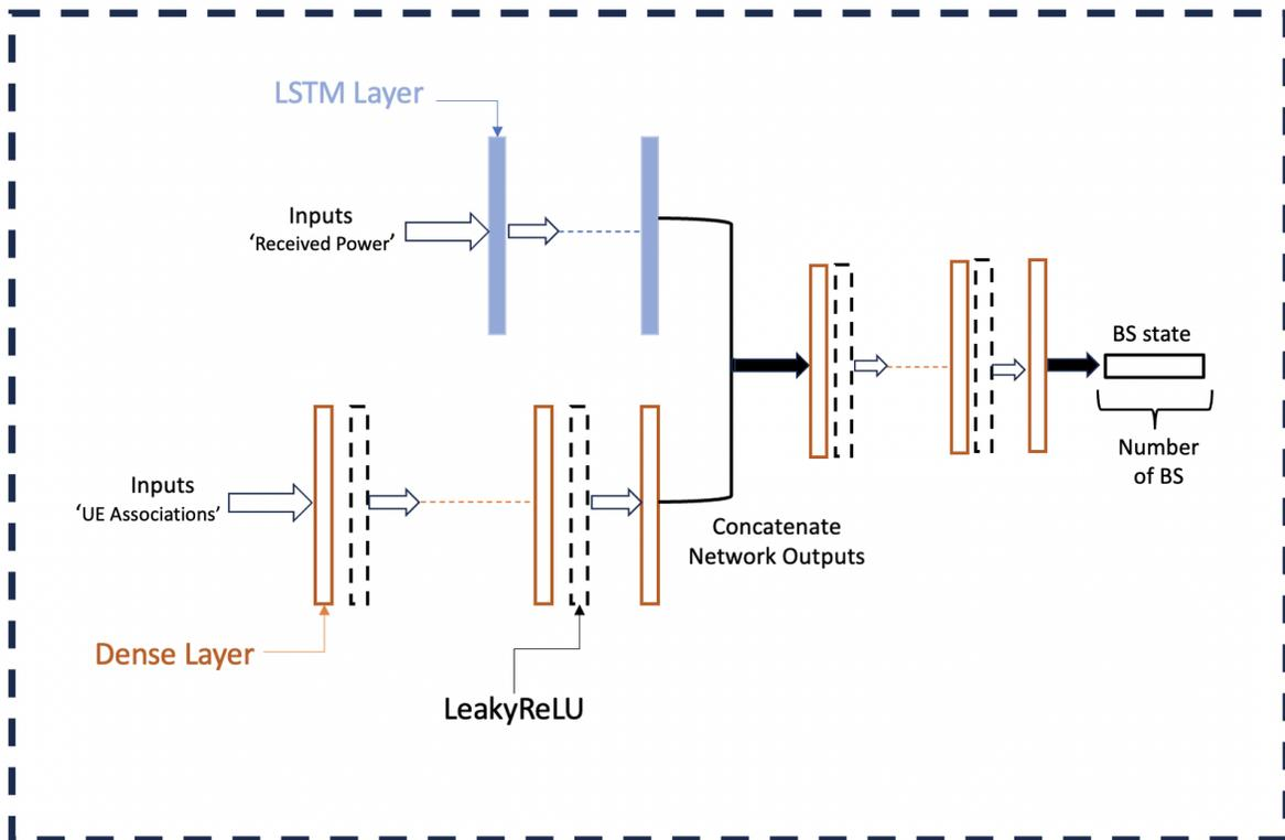
FIGURE 5.3 : Fused Model Structure.
