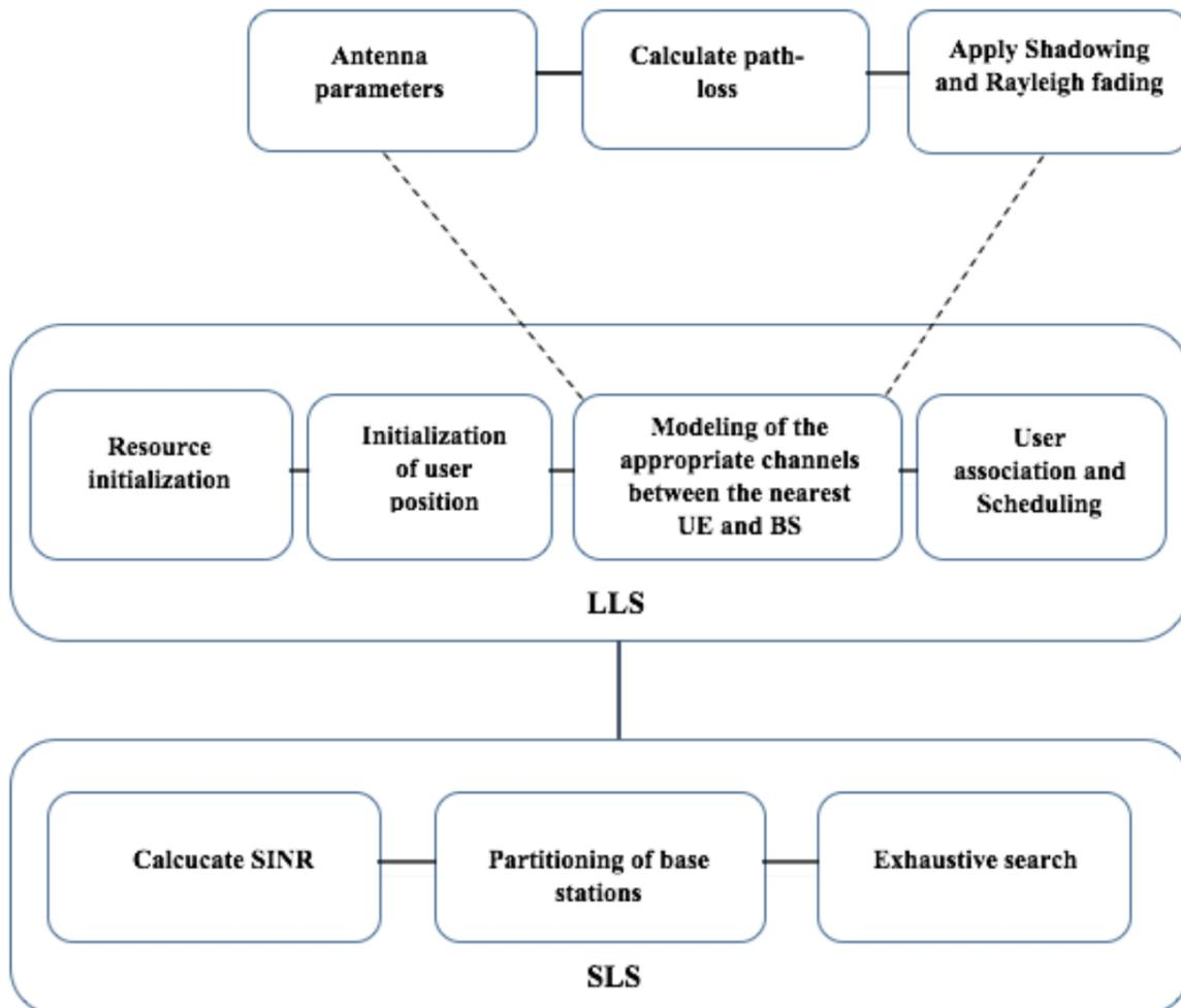
FIGURE 6.1 : Simulator Structure.
