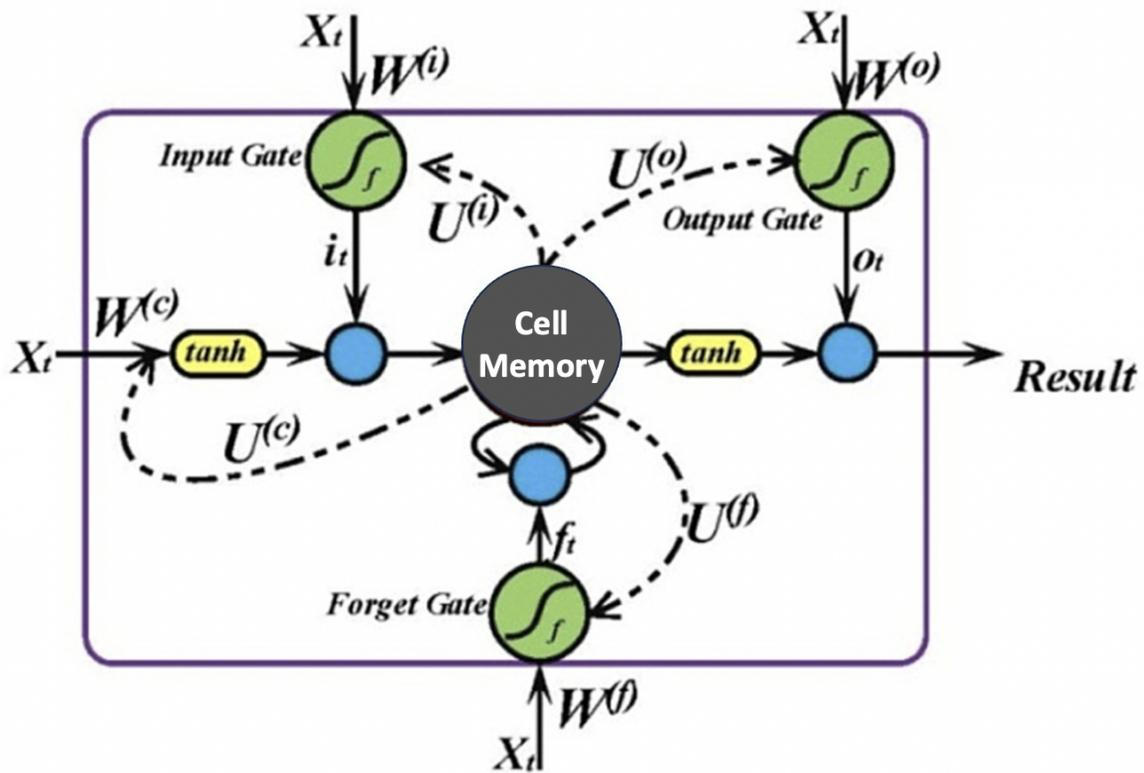
FIGURE 3.3 : The structure of LSTM's memory unit.
