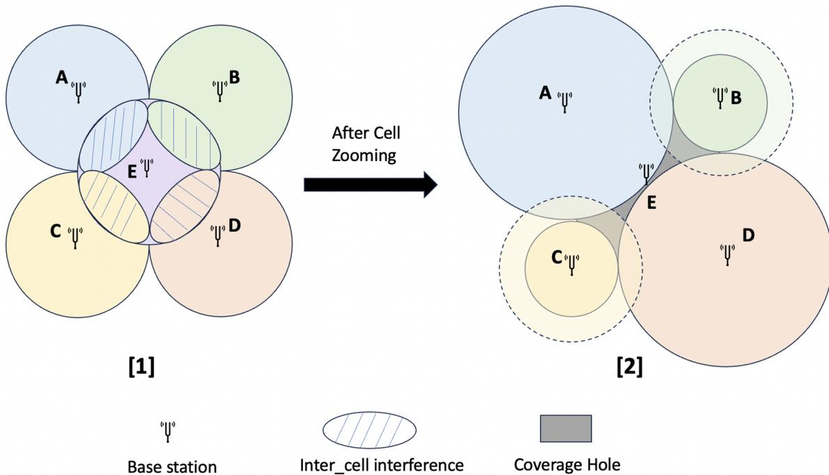
**FIGURE 2.5 : Cell zooming [1] : Normal cells deployed A-E. [2] : Cell E in sleep mode, cells A and C increasing their coverage to compensate, and B and D reducing their coverage.**
