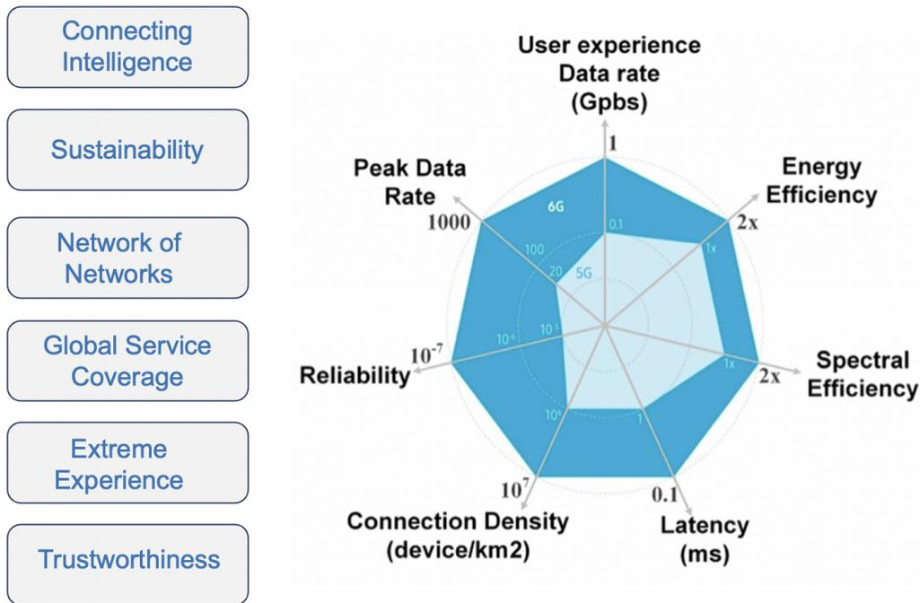
FIGURE 1.3 : Key enhancements of 6G versus 5G.
