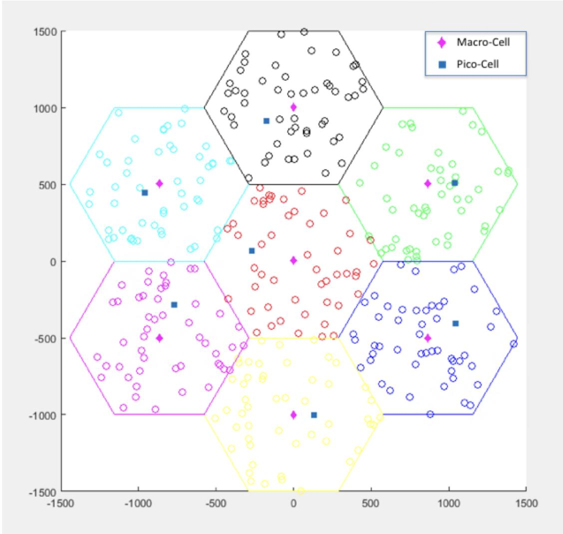
**FIGURE 6.6 : Distribution of users in the cellular network with hexagonal architecture**
