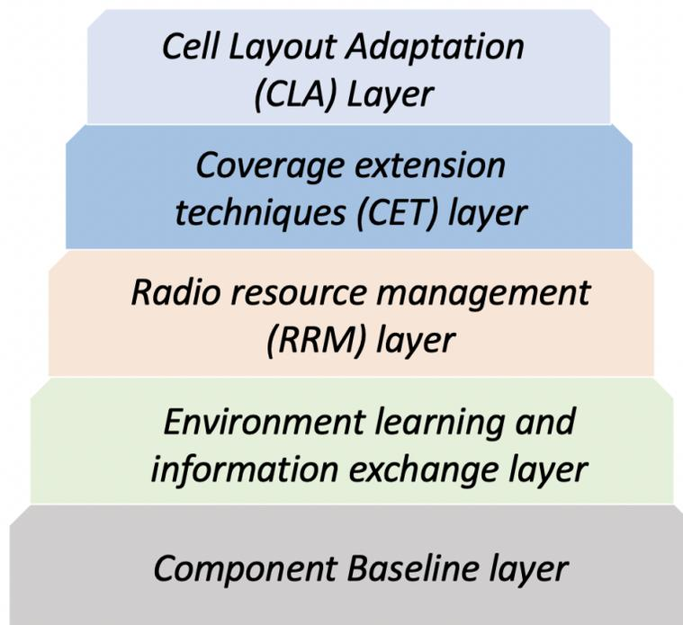
**FIGURE 2.2 : Framework with Stacked Layers for Energy-Efficient Strategies in Cellular Networks**
