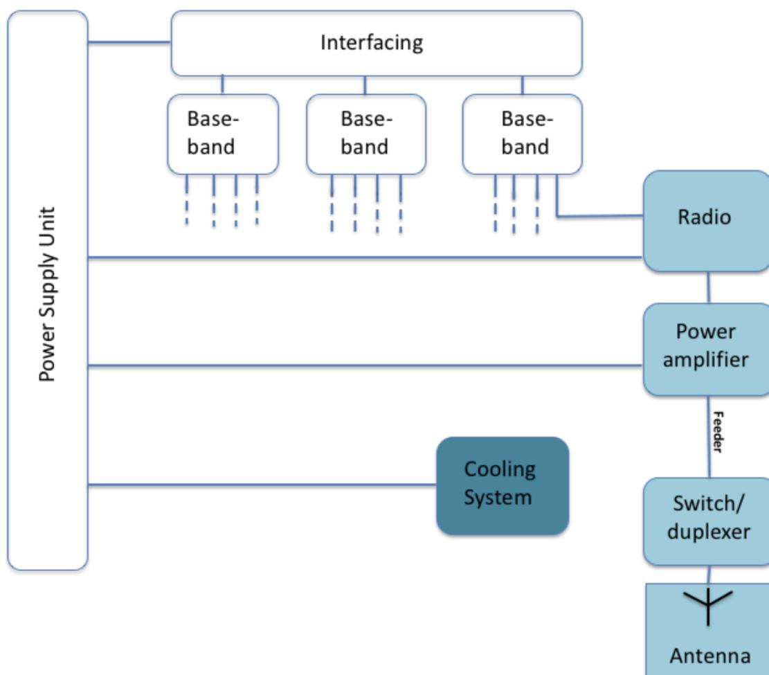
**FIGURE 4.2 : Base station architecture configured for a three-sector system with four transmit antennas per sector, enabling MIMO functionality.**
