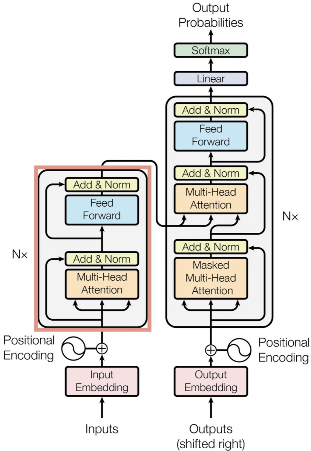
FIGURE 3.5 : The Transformer architecture's encoder-decoder structure, as presented in the paper "Attention Is All You Need".
