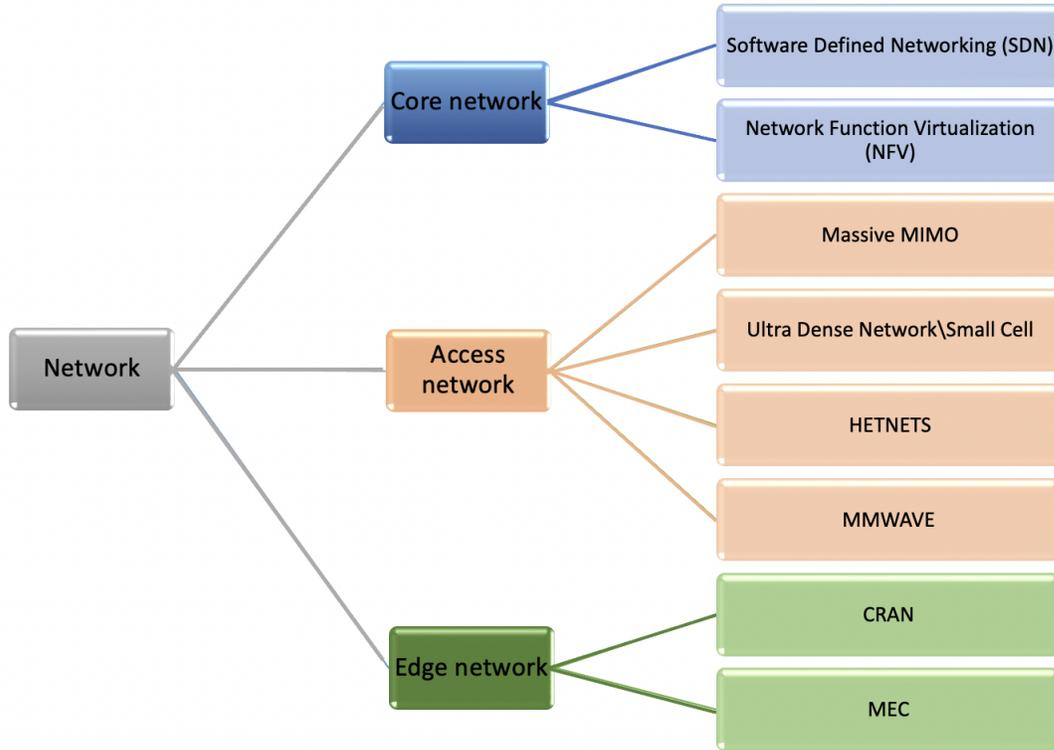
**FIGURE 2.1 : 5G technologies designed to boost energy efficiency.**
