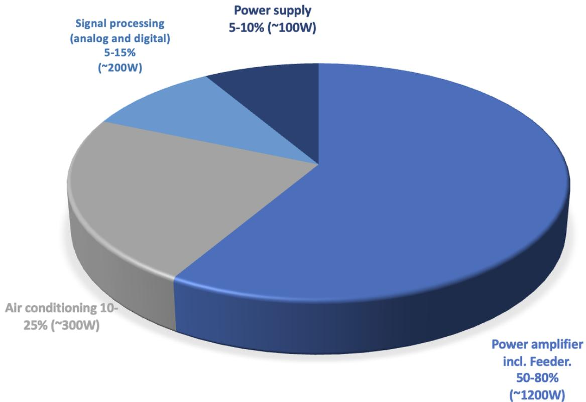
**FIGURE 4.1 : Power Consumption Across Different Base Station Components.**
