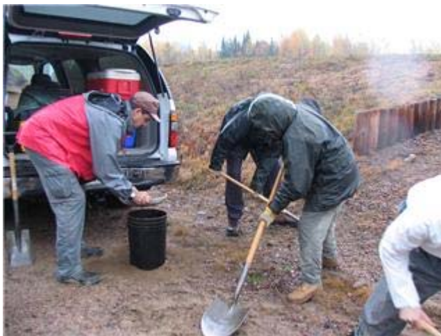
Figure 17. Sampling of propellant residues at the firing positions on antitank training range A, at CFB Petawawa.
