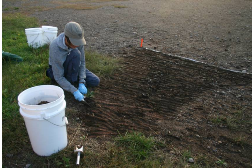
Figure 15. Sampling of propellant residues at firing position 2 of the Wellington antitank range, CFB Gagetown.
