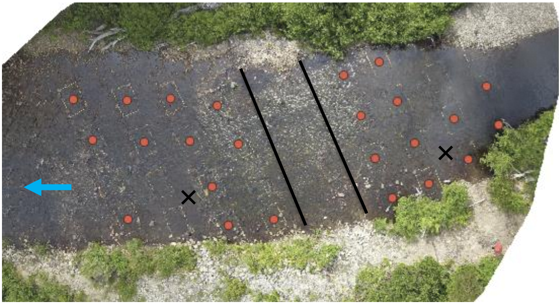
Figure 12. Aerial photo of the study site. The red dots represent the 24 functioning antennas on the study site. The black lines represent the ford. The blue arrow indicates the direction of the current. Fish were released at the two x. © Charles Gignac (2019)
