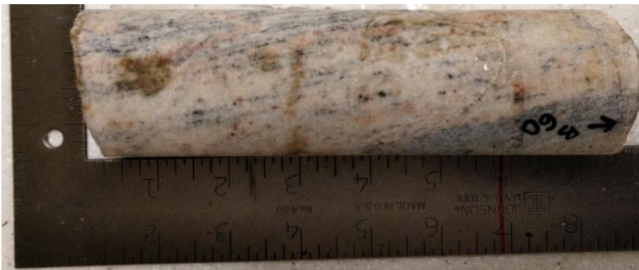
Figure A3.11. Sample F60 – Paragneiss sample from 60 m depth – Core box #16.
