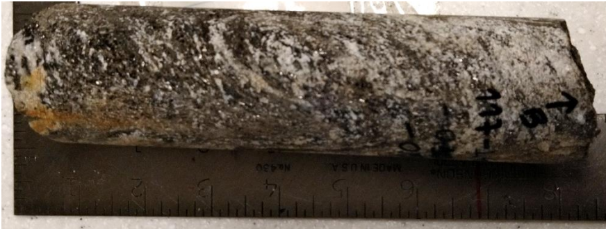
Figure A4.15. Sample F117 - Diorite sample from 114.88 m depth – Core box #29.
