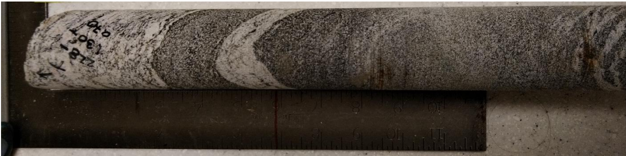
Figure A4.29. Sample F228 - Diorite sample from 226 m depth – Core box #55.
