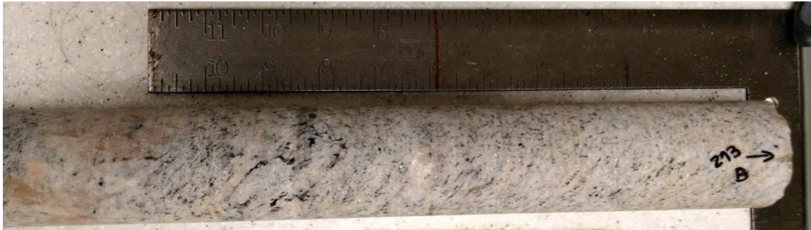
Figure A3.57. Sample F213 – Paragneiss sample from 213 m depth – Core box #52.
