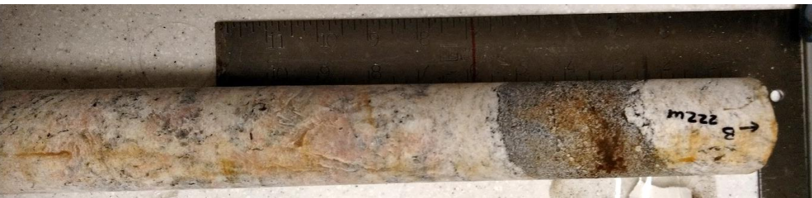
Figure A5.10. Sample F222 - Granitoid sample from 222 m depth – Core box #54.
