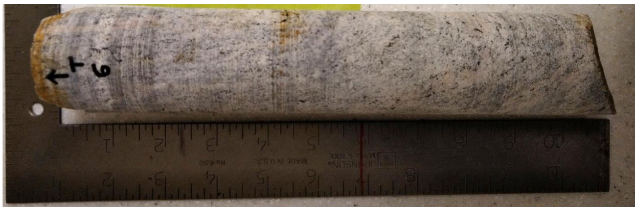
Figure A3.1. Sample F6 - Paragneiss sample from 6 m depth – Core box #1.
