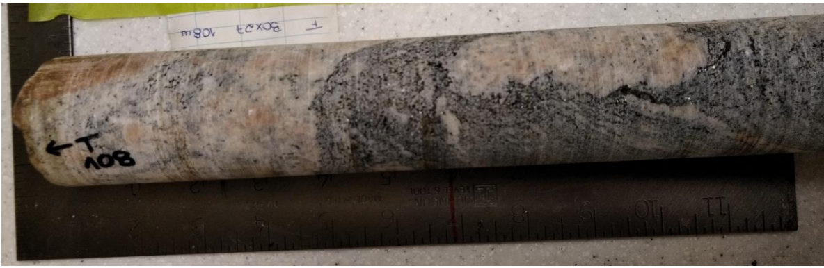
Figure A3.28. Sample F108 – Paragneiss sample from 108 m depth – Core box #27.
