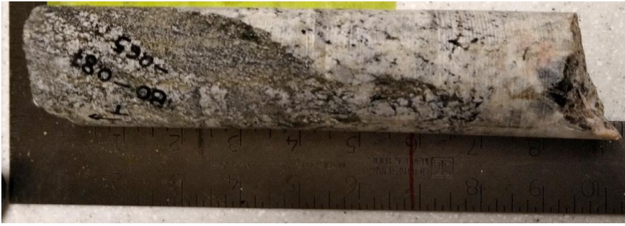
Figure A3.48. Sample F180 – Paragneiss sample from 178.48 m depth in contact with diorite (probably Kaslac Complex or Ralleau Suite) – Core box #44.
