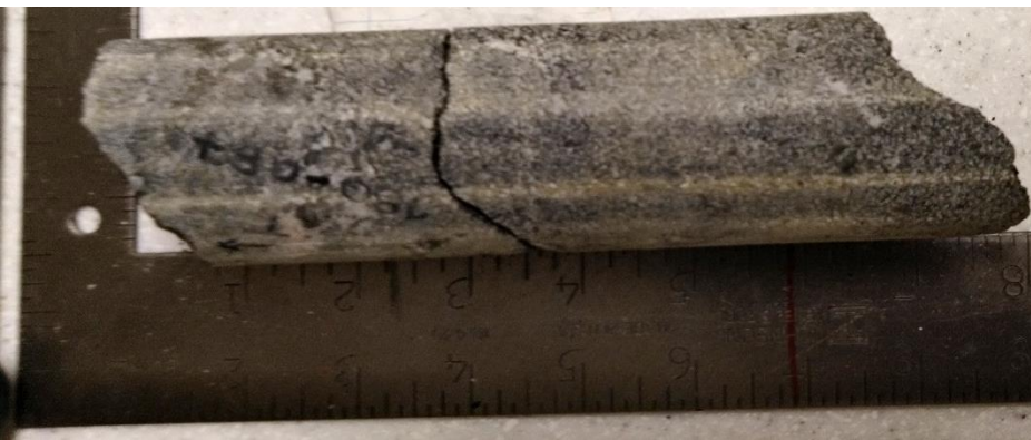
Figure A4.22. Sample F180 – Gabbro sample from 179.13 m depth – Core box #44.
