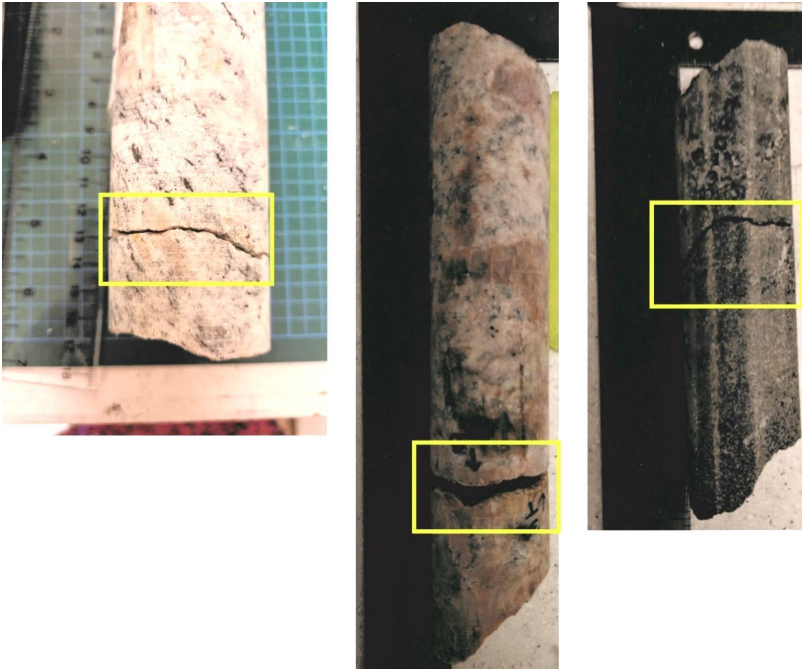
Figure 4.10. Example of horizontal induced fractures (highlighted by the green square) observed along the core.
