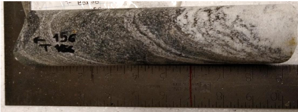
Figure A4.16. Sample F156 - Diorite sample from 156 m depth – Core box #38.
