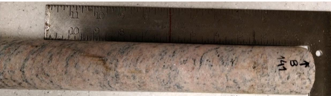
Figure A3.39. Sample F141 – Paragneiss sample from 141 m depth – Core box #35.
