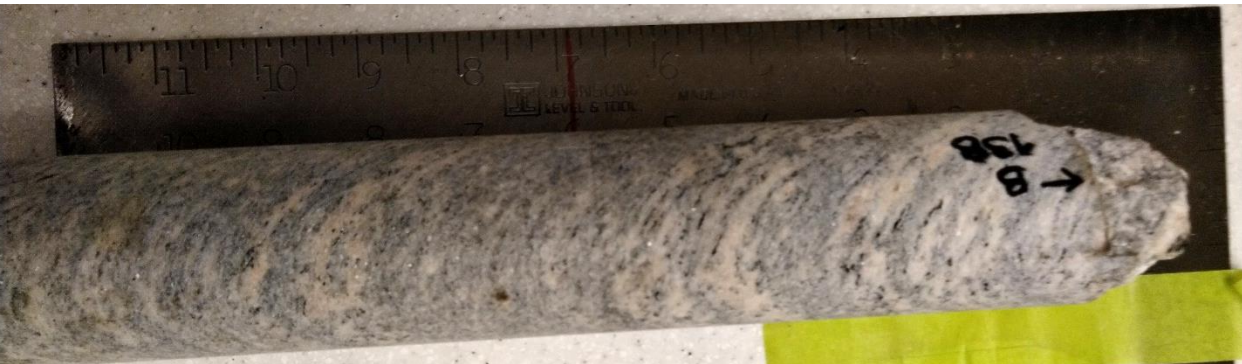
Figure A3.38. Sample F138 – Paragneiss sample from 138 m depth – Core box #34.
