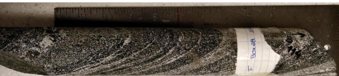
Figure A4.14. Sample F114 - Diorite sample from 114 m depth – Core box #28.
