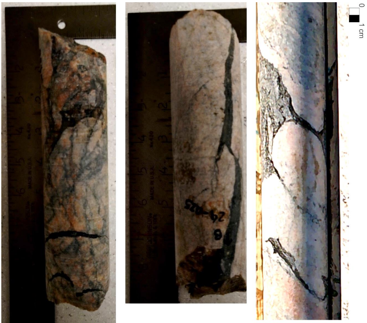
Figure 4.11. Example of fissures (right), veins (center) and expulsion structures (left) observed along the core.
