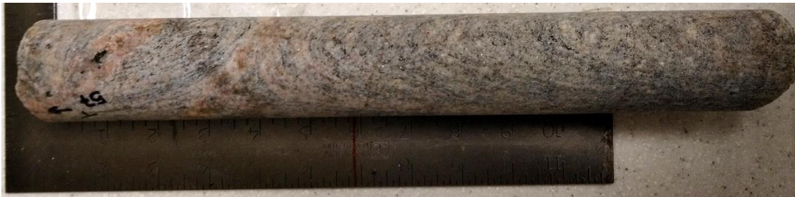
Figure A3.10. Sample F57 - Paragneiss sample from 57 m depth – Core box #15.
