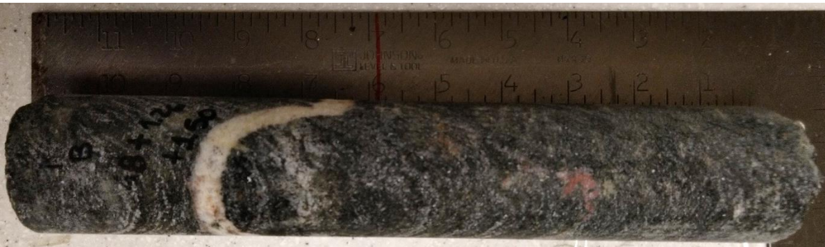
Figure A4.10. Sample F48 – Gabbro sample from 50.76 m depth with garnet clusters – Core box #14.
