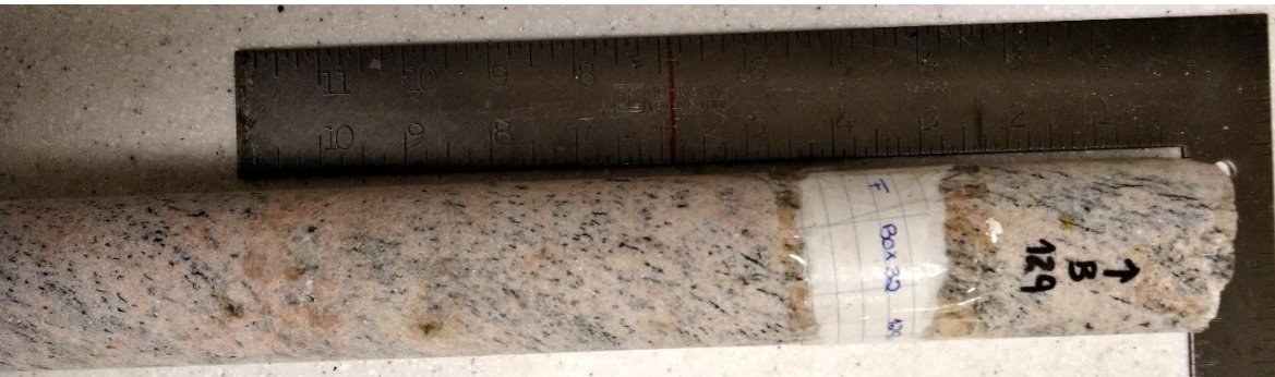
Figure A3.34. Sample F129 – Paragneiss sample from 129 m depth – Core box #32.
