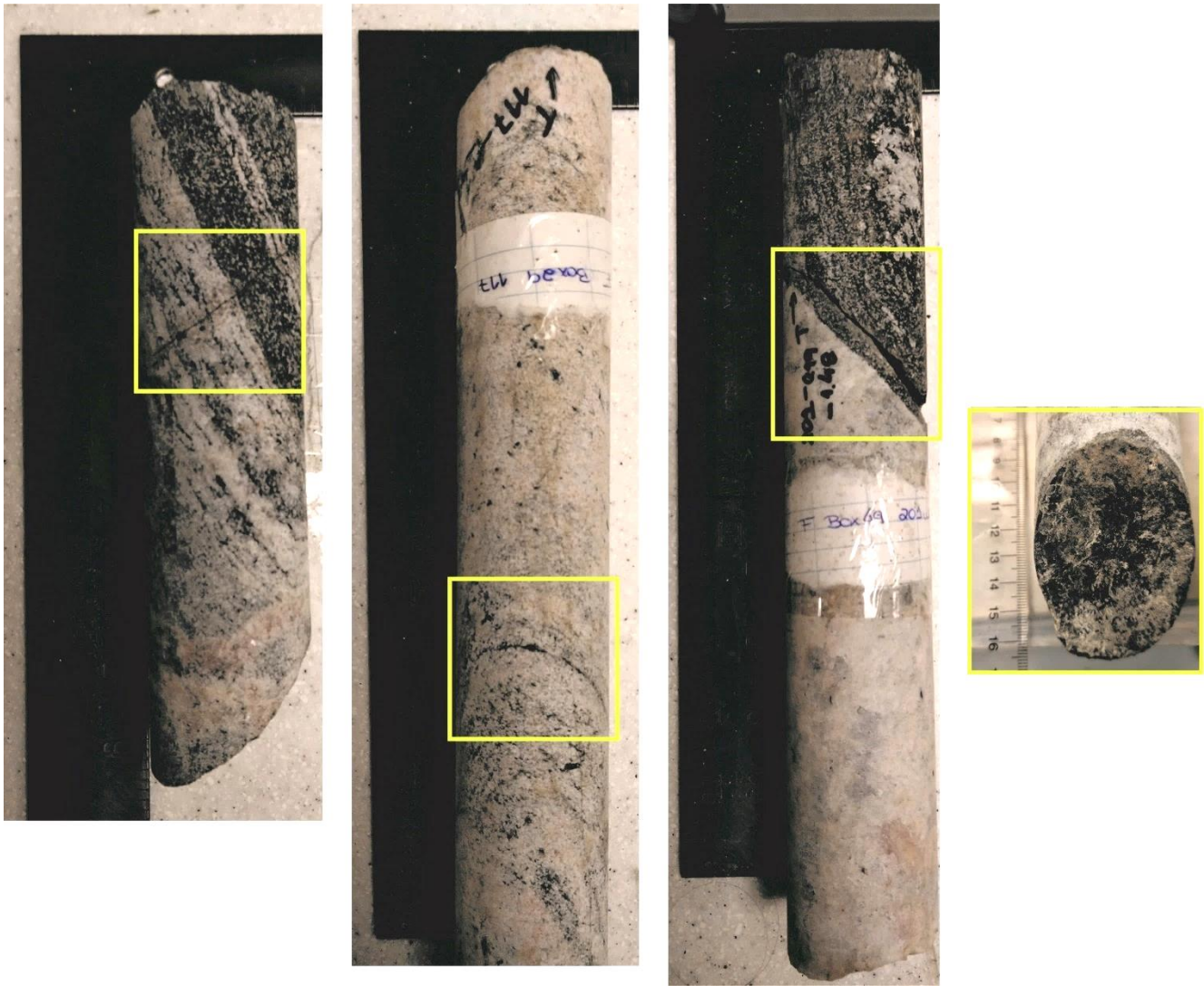
Figure 4.8. Example of inclined fractures (highlighted by the green square) observed along the core.
