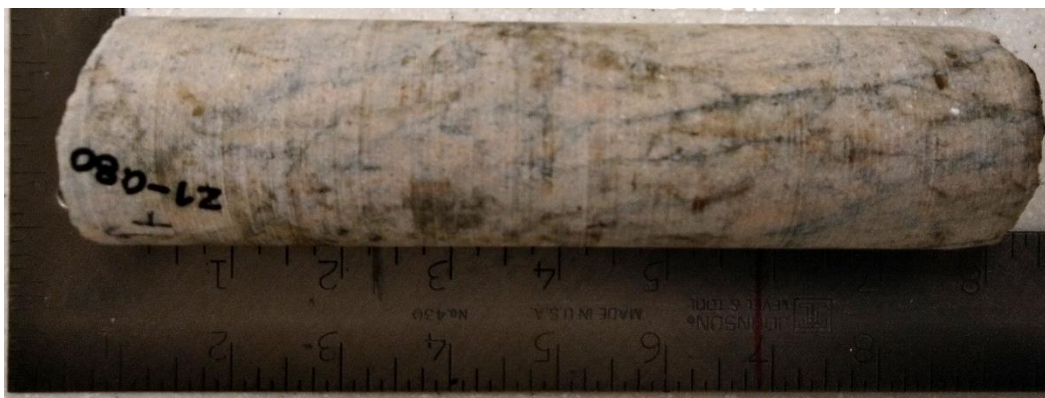
Figure A5.2. Sample F21 - Granitoid sample from 20.20 m depth – Core box #7.
