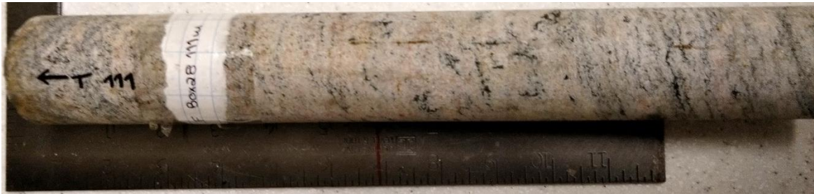
Figure A3.29. Sample F111 – Paragneiss sample from 111 m depth – Core box #28.
