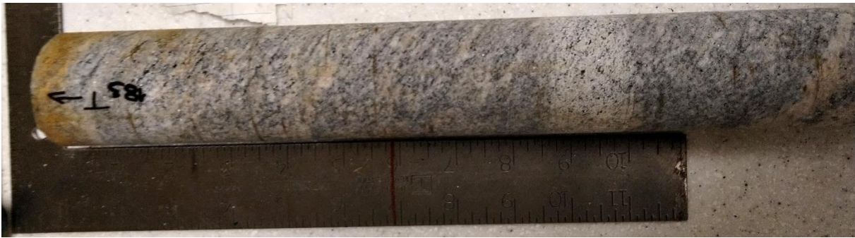
Figure A3.50. Sample F183 – Paragneiss sample from 183 m depth – Core box #45.
