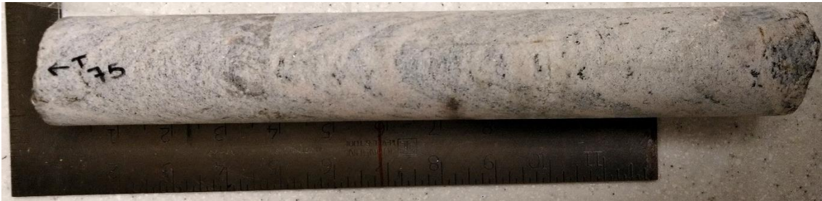
Figure A3.18. Sample F75 - Paragneiss sample from 75 m depth – Core box #19.
