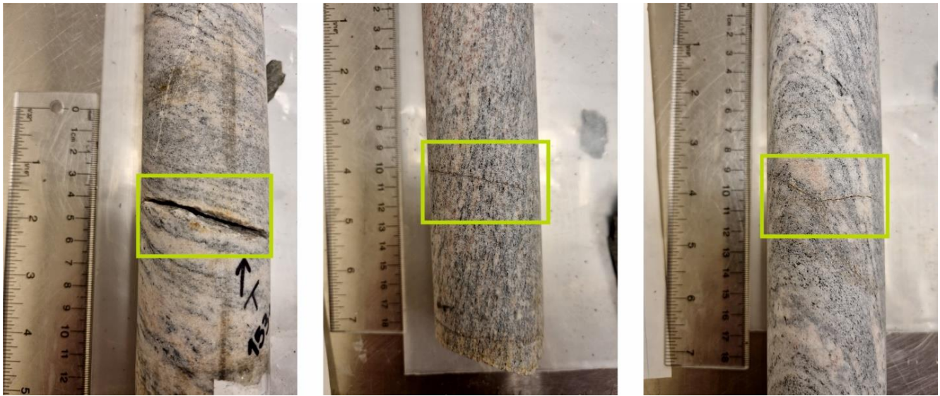
Figure 4.9. Example of horizontal natural fractures (highlighted by the green square) observed along the core.
