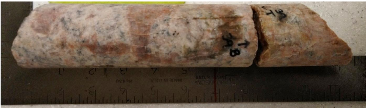
Figure A5.5. Sample F39 - Granitoid sample from 39 m depth – Core box #12.
