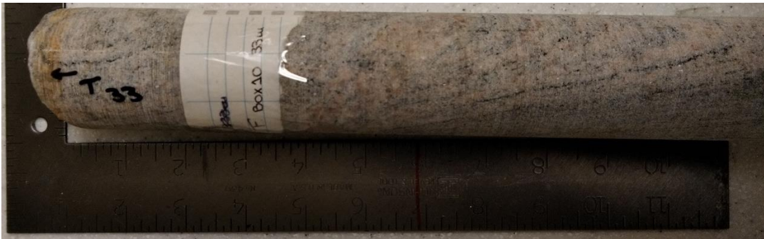
Figure A3.6. Sample F33 – Paragneiss sample from 33 m depth – Core box #10.
