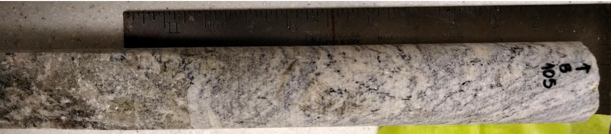
Figure A3.27. Sample F105 – Paragneiss sample from 105 m depth – Core box #26.
