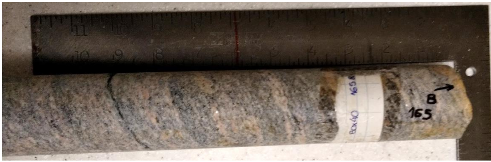
Figure A3.44. Sample F165 – Paragneiss sample from 165 m depth – Core box #40.
