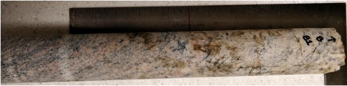
Figure A3.20. Sample F81 – Paragneiss sample from 81 m depth – Core box #21.
