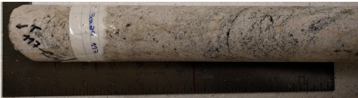
Figure A3.30. Sample F117 – Paragneiss sample from 115.55 m depth – Core box #29.
