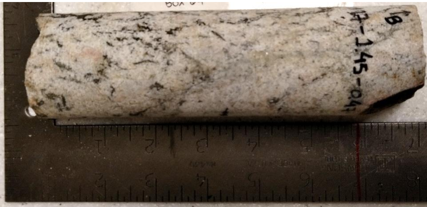
Figure A5.8. Sample F117 - Granitoid sample from 115.08 m depth – Core box #29.
