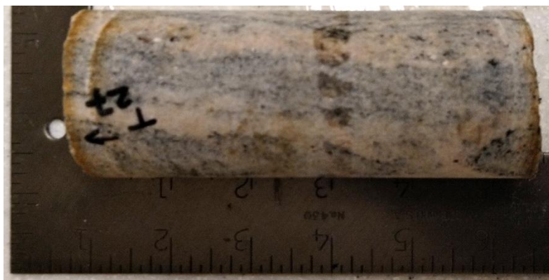
Figure A3.3. Sample F27 – Paragneiss sample from 27 m depth – Core box #9.
