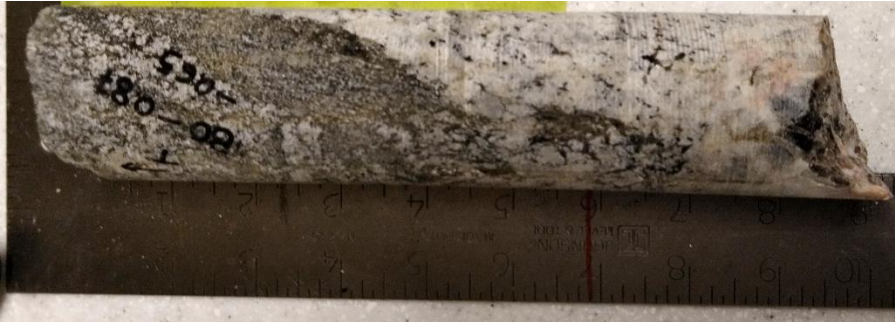
Figure A4.21. Sample F180 - Diorite sample from 178.48 m depth in contact with paragneiss (False Suite) - Core box #44.
