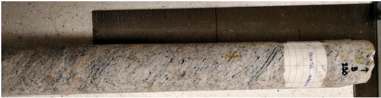
Figure A3.56. Sample F210 – Paragneiss sample from 210 m depth – Core box #51.
