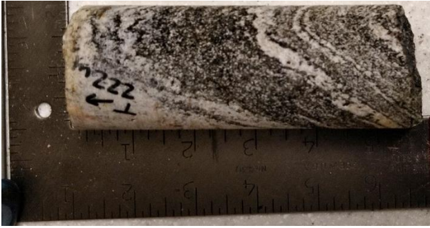
Figure A4.28. Sample F222 - Diorite sample from 222 m depth – Core box #54.
