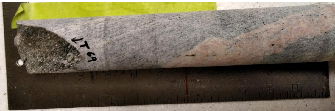
Figure A3.15. Sample F69 - Paragneiss sample from 69 m depth – Core box #18.
