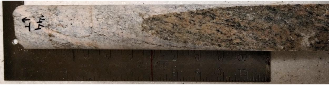
Figure A3.40. Sample F144 – Paragneiss sample from 144 m depth – Core box #35.
