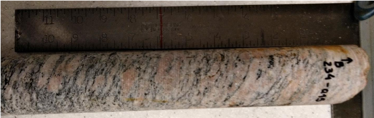
Figure A3.61. Sample F234 – Paragneiss sample from 233.85 m depth – Core box #56.
