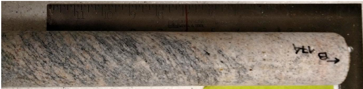
Figure A3.46. Sample F174 – Paragneiss sample from 174 m depth with contact with a tonalitic/granitic intrusion (probably Aveneau or Dancelou suites) – Core box #43.
