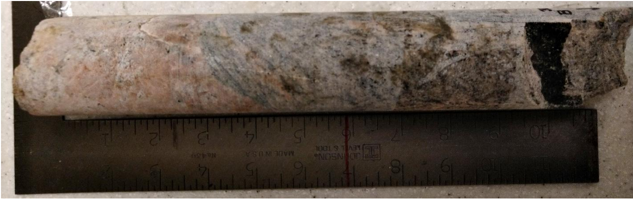
Figure A3.4. Sample F30 – Paragneiss sample from 30 m depth with the contact with a pink pegmatitic granitic intrusion (probably Dancelou Suite) – Core box #10.
