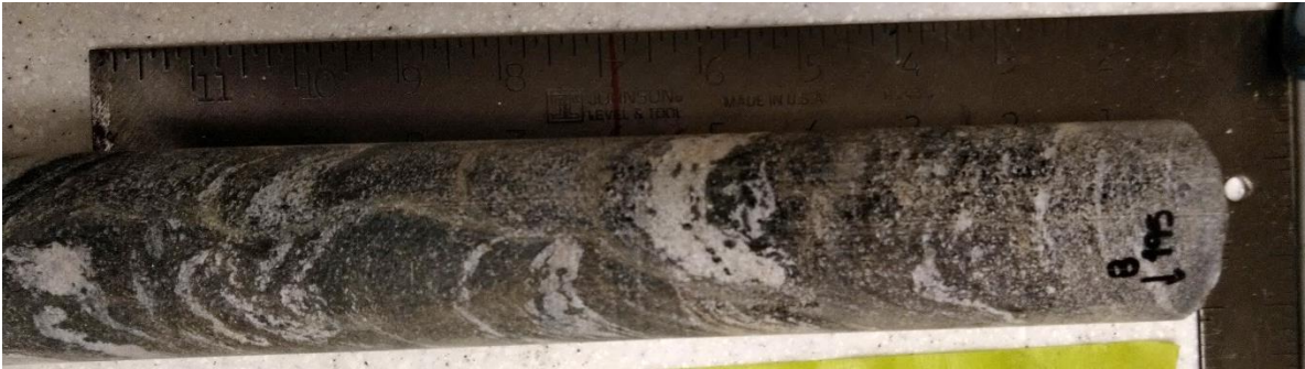
Figure A4.24. Sample F195 - Diorite sample from 195 m depth – Core box #47.
