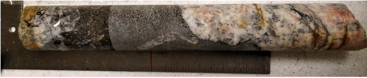
Figure A4.27. Sample F219 - Diorite sample from 219 m depth with tonalitic/granitic intrusion – Core box #53.
