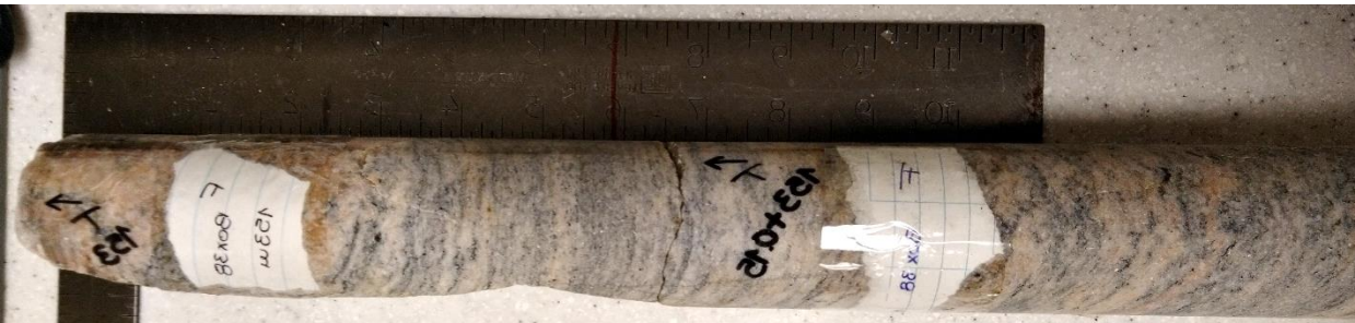
Figure A3.43. Sample F153 – Paragneiss sample from 153 m depth with contact with a pink pegmatitic granitic intrusion (probably Dancelou Suite) – Core box #38.
