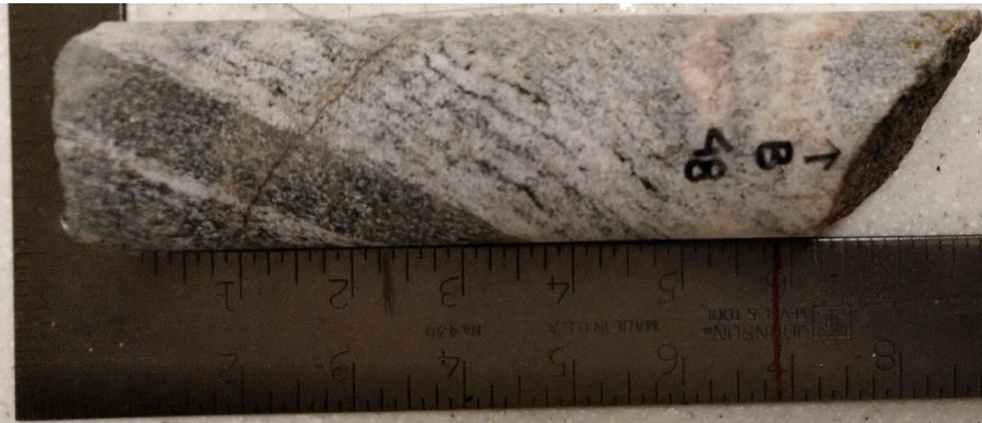
Figure A4.9. Sample F48 - Diorite sample from 48 m depth – Core box #14.
