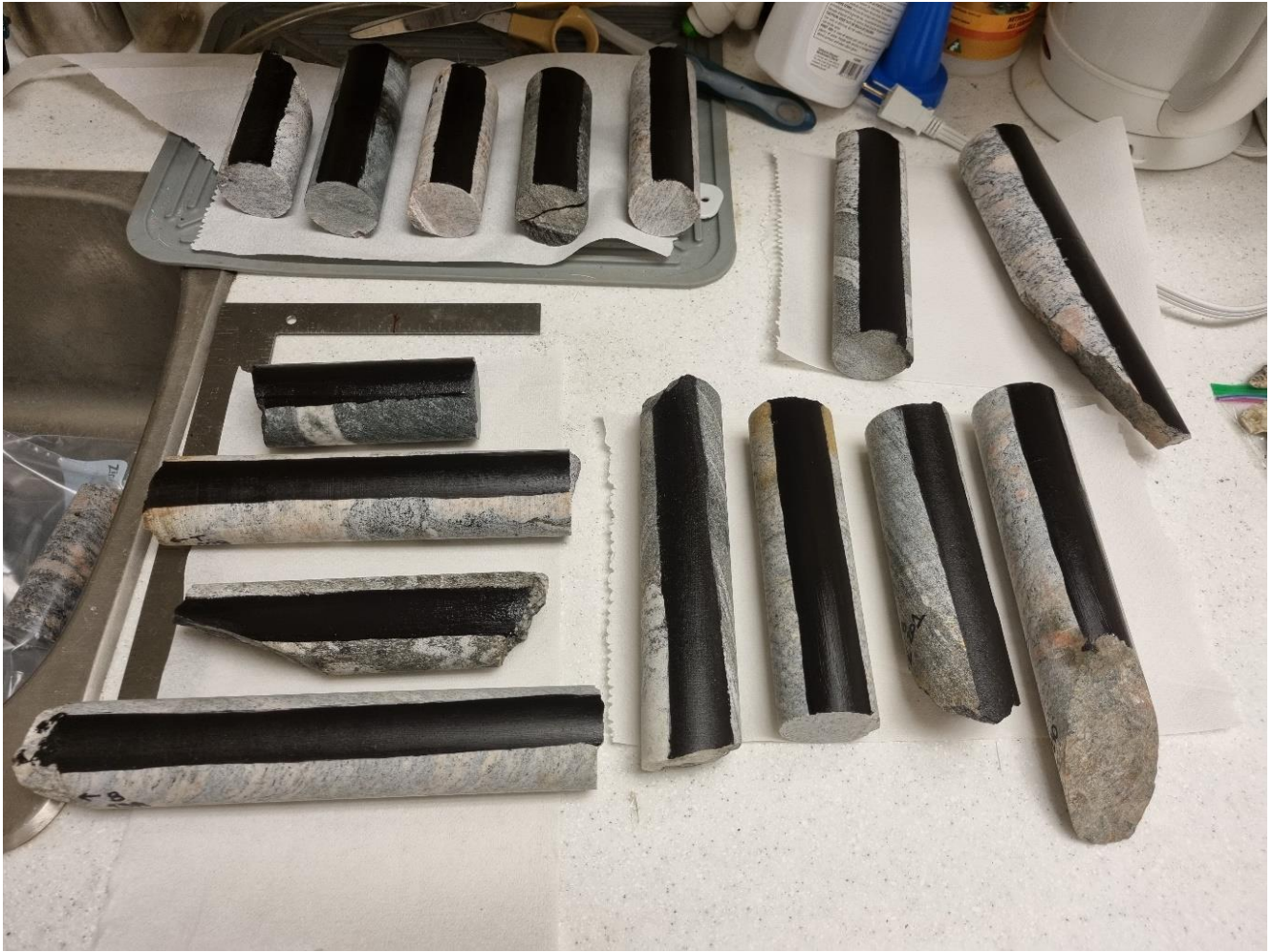
Figure 5.4. Black silicone painted on the samples surface.
