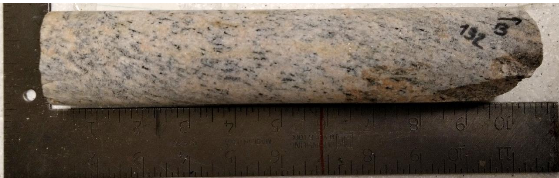
Figure A3.35. Sample F132 – Paragneiss sample from 132 m depth – Core box #33.
