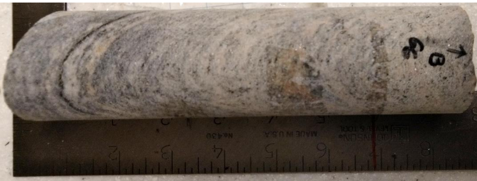
Figure A3.14. Sample F66 - Paragneiss sample from 66 m depth – Core box #17.
