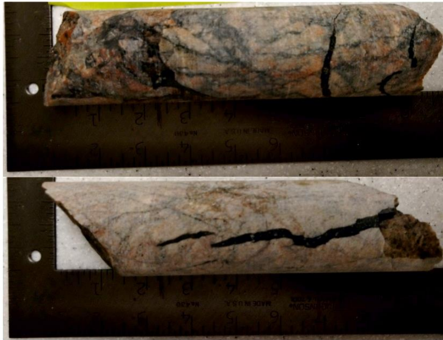
Figure 4.7. Features of the tonalite/granite core samples: a) alignment of biotite schlieren, b) fissures and veins.
