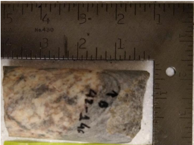
Figure A5.6. Sample F42 - Granitoid sample from 40.54 m depth – Core box #12.
