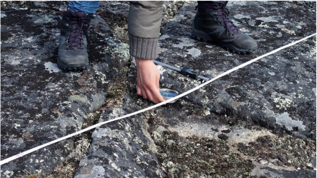
Figure 4.2. Example of the application of the scanline sampling method to acquire fracture geometrical information on an outcrop surface.
