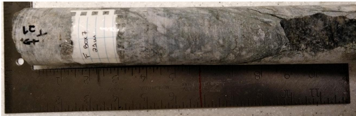
Figure A4.6. Sample F21 – Diorite sample from 21 m depth – Core box #7.
