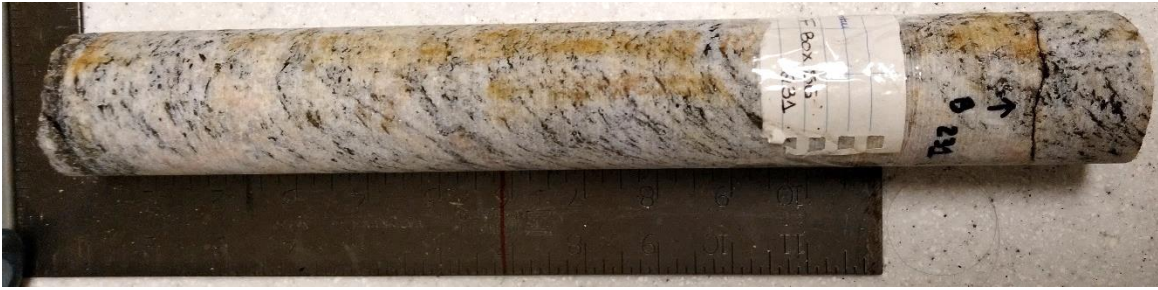
Figure A3.60. Sample F231 – Paragneiss sample from 231 m depth – Core box #56.
