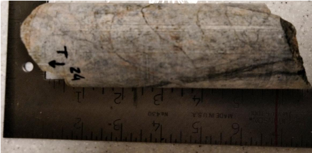
Figure A5.4. Sample F24 - Granitoid sample from 24 m depth – Core box #8.
