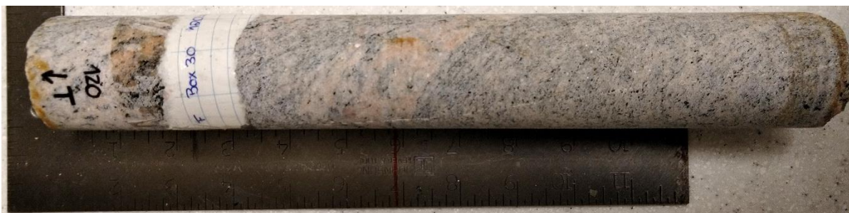
Figure A3.31. Sample F120 – Paragneiss sample from 120 m depth – Core box #30.
