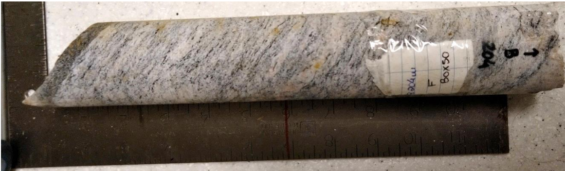
Figure A3.54. Sample F204 – Paragneiss sample from 204 m depth – Core box #50.
