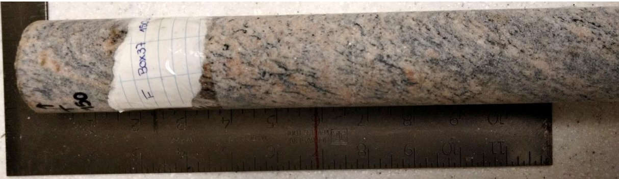
Figure A3.42. Sample F 150 – Paragneiss sample from 150 m depth – Core box #37.
