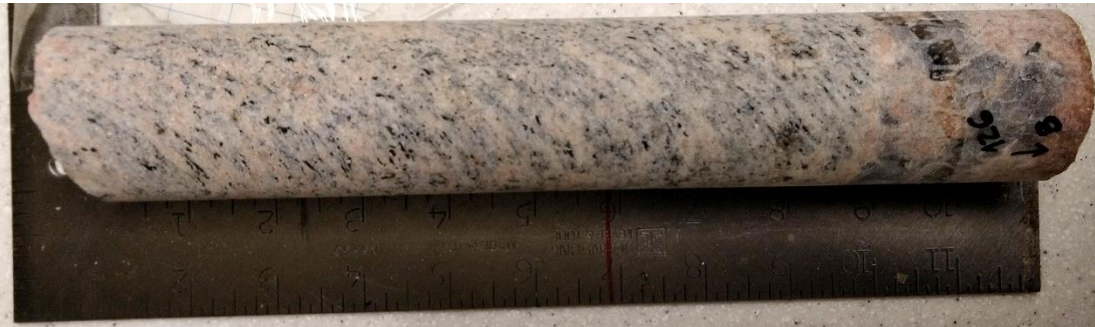
Figure A3.33. Sample F126 – Paragneiss sample from 126 m depth with contact with a pink pegmatitic granitic intrusion (probably Dancelou Suite) – Core box #31.
