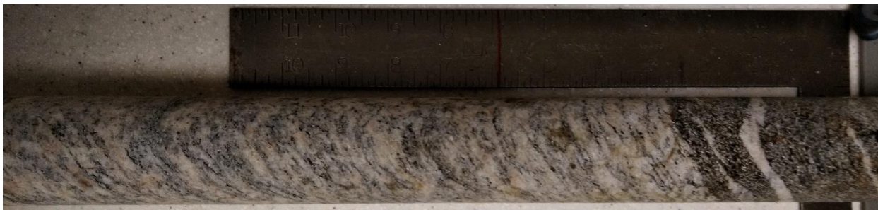
Figure A3.47. Sample F177 – Paragneiss sample from 177 m depth in contact with diorite (probably Kaslac Complex or Ralleau Suite) – Core box #43.
