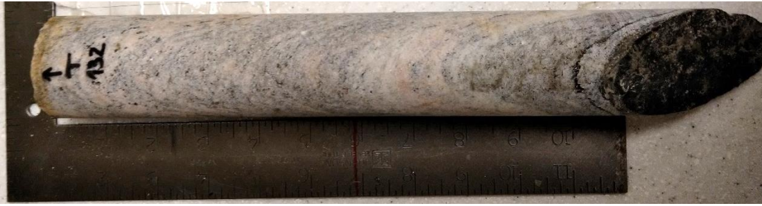
Figure A3.36. Sample F132 – Paragneiss sample from 132 m depth – Core box #33.
