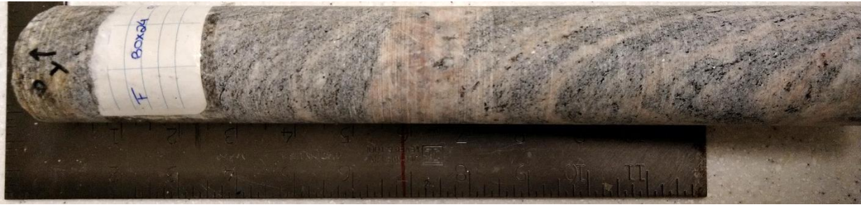
Figure A3.24. Sample F96 – Paragneiss sample from 96 m depth – Core box #24.
