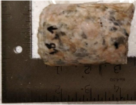
Figure A5.7. Sample F81 - Granitoid sample from 81 m depth – Core box #21.
