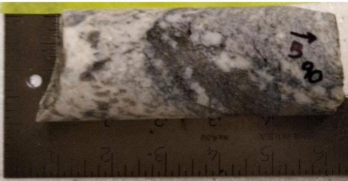
Figure A4.12. Sample F90 - Diorite sample from 90 m depth – Core box #23.
