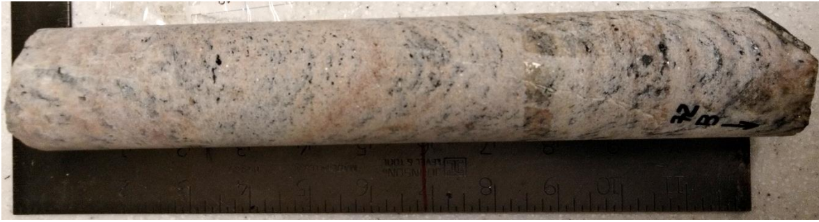
Figure A3.16. Sample F72 - Paragneiss sample from 72 m depth – Core box #19.
