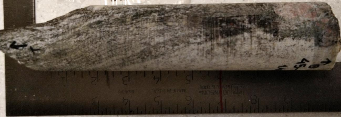
Figure A4.8. Sample F45 - Diorite sample from 41.89 m depth with garnet clusters – Core box #13.
