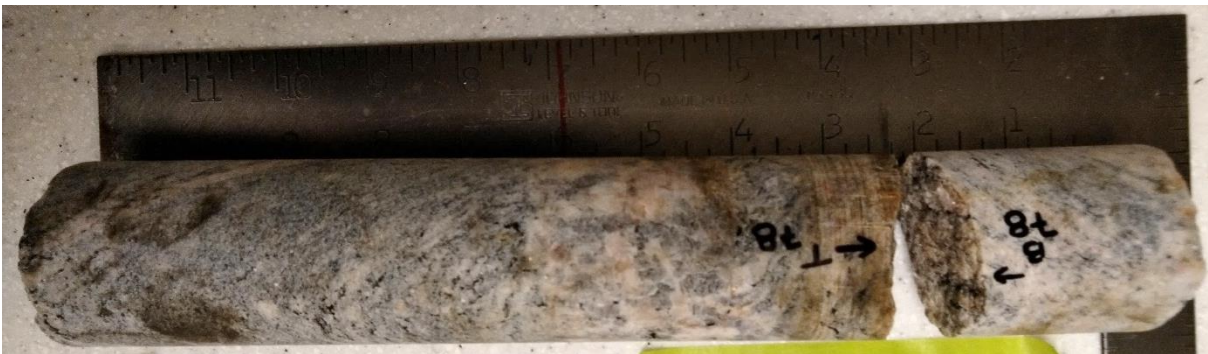
Figure A3.19. Sample F78 – Paragneiss sample from 78 m depth – Core box #20.
