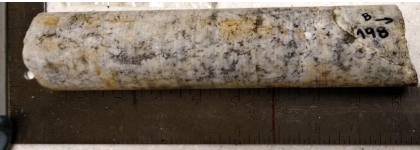
Figure A5.9. Sample F198 - Granitoid sample from 198 m depth – Core box #48.
