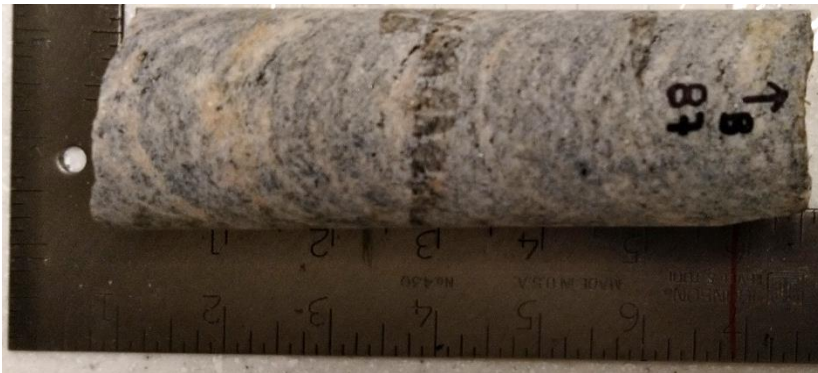
Figure A3.22. Sample F87 – Paragneiss sample from 87 m depth – Core box #22.
