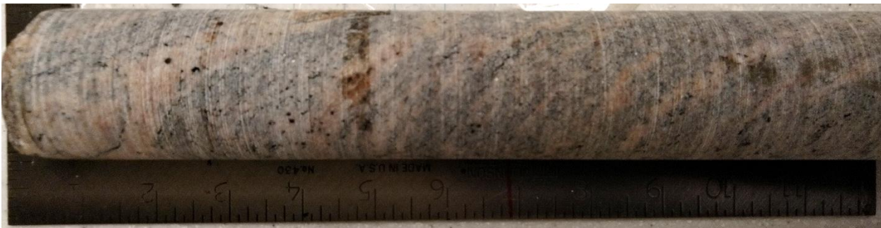
Figure A3.7. Sample F36 – Paragneiss sample from 36.62 m depth – Core box #11.
