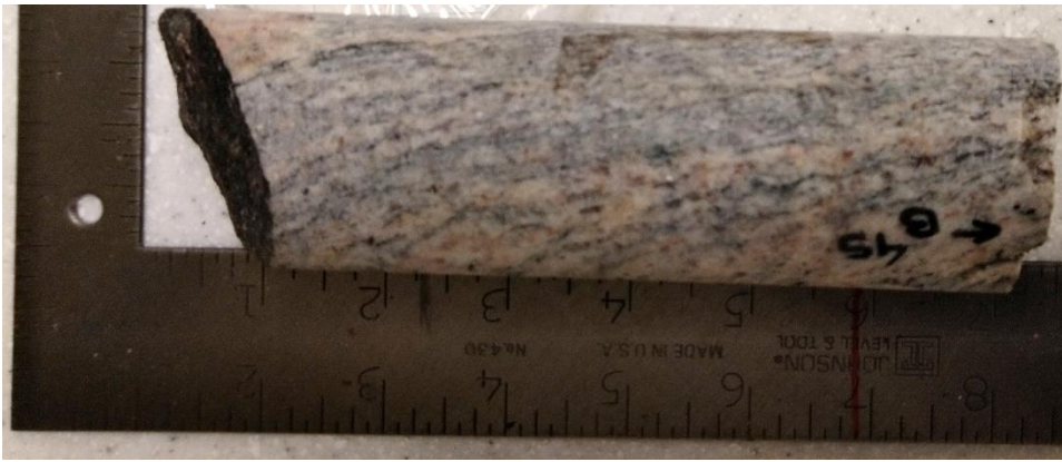
Figure A3.8. Sample F45 – Paragneiss sample from 45 m depth – Core box #13.
