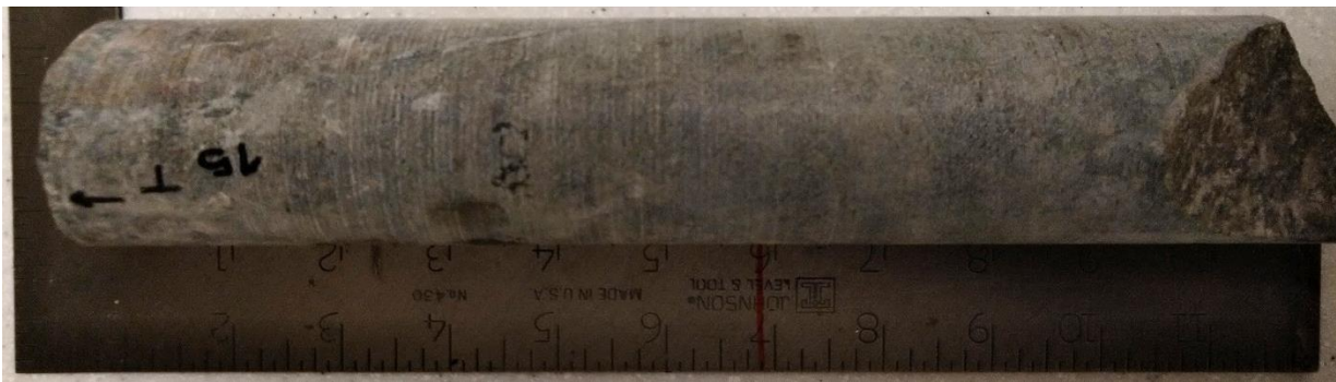
Figure A4.3. Sample F15 – Gabbro sample from 15 m depth – Core box #5.
