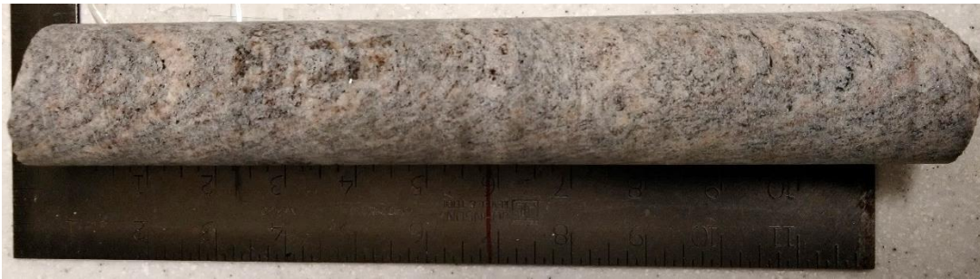
Figure A3.9. Sample F48 - Paragneiss sample from 46.35 m depth – Core box #14.
