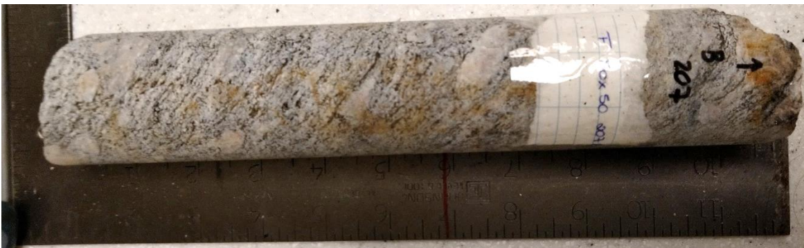
Figure A3.55. Sample F207 – Paragneiss sample from 207 m depth – Core box #50.
