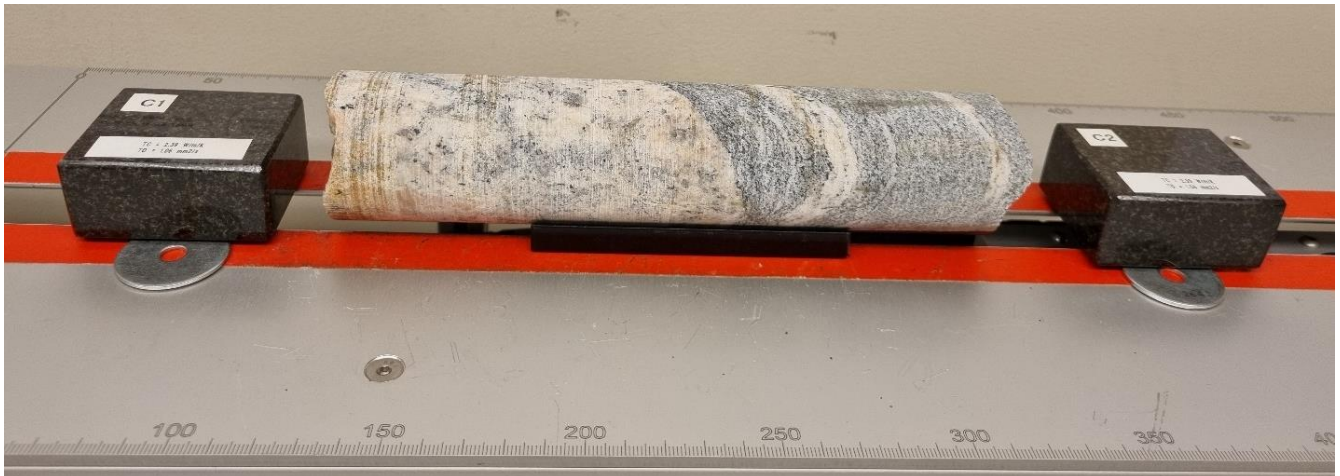
Figure 5.5. Example of the experimental setup for thermal conductivity analysis.
