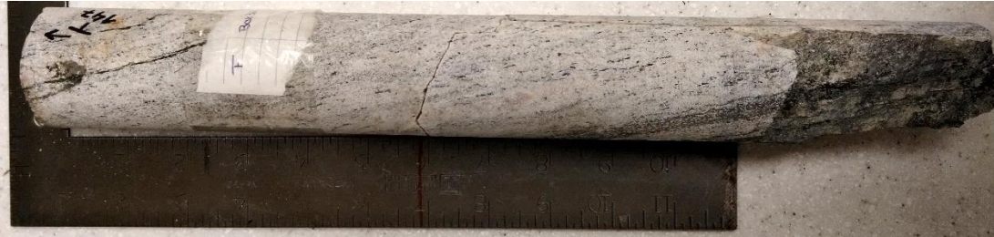
Figure A3.41. Sample F147 – Paragneiss sample from 147 m depth – Core box #36.
