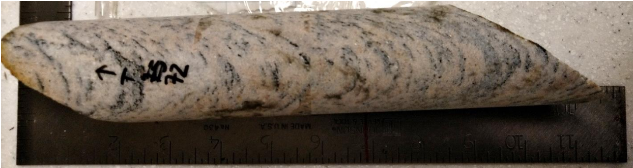
Figure A3.17. Sample F72 - Paragneiss sample from 72 m depth – Core box #19.
