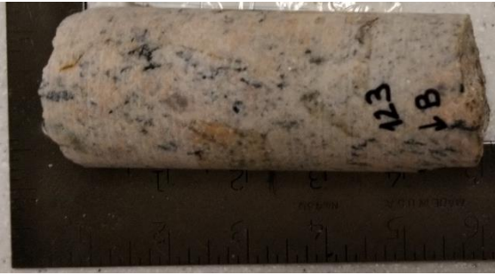
Figure A3.32. Sample F123 – Paragneiss sample from 123 m depth – Core box #31.
