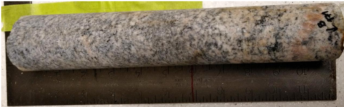
Figure A3.45. Sample F171 – Paragneiss sample from 171 m depth – Core box #42.
