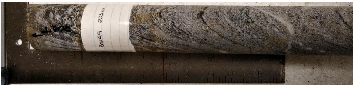
Figure A4.26. Sample F201 – Diorite sample from 201 m depth – Core box #49.
