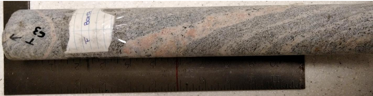
Figure A3.13. Sample F63 - Paragneiss sample from 63 m depth – Core box #17.
