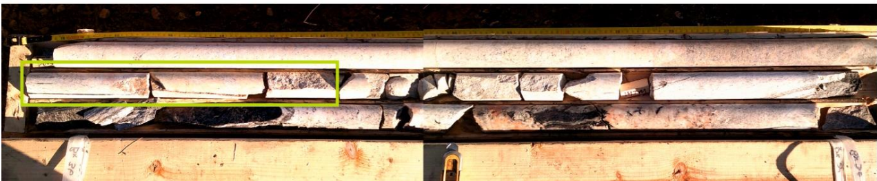
Figure 4.14. Example of drilling-induced centerline and petal-centerline fractures (highlighted by the green squares) observed in several sections of the core (top – 168 m depth; center – 150 m depth; bottom – 147 m depth).
