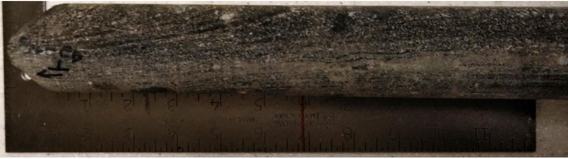
Figure A4.7. Sample F42 – Gabbro sample from 40.55 m depth with garnet clusters – Core box #12.
