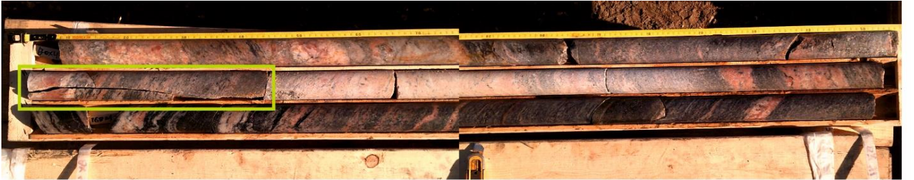
Figure 4.13. Example of coring-induced disc fractures (highlighted by the dashed red lines) observed in a section of the core (180 m depth).
