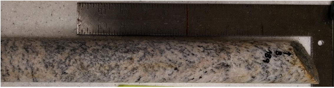
Figure A3.52. Sample F189 – Paragneiss sample from 189 m depth – Core box #46.
