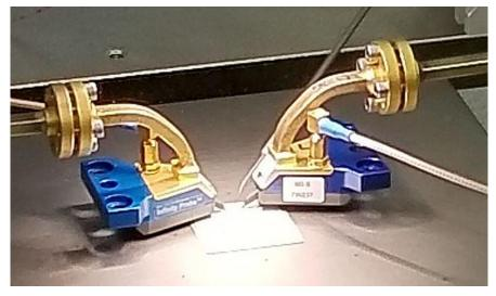
Figure 2.10 A photo of a circuit under test using GSG coplanar probes.
