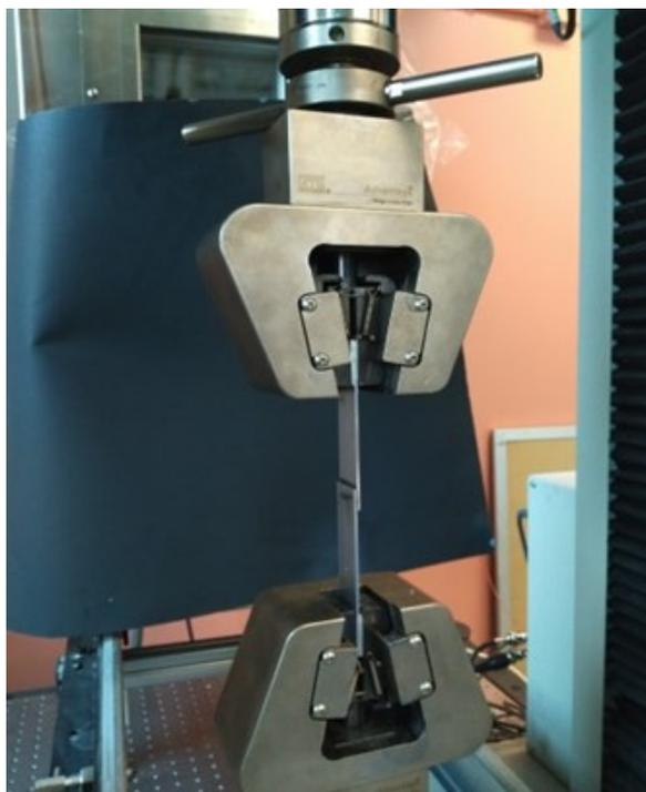
**Figure 5.3** Experimental set-up for single lap shear test
