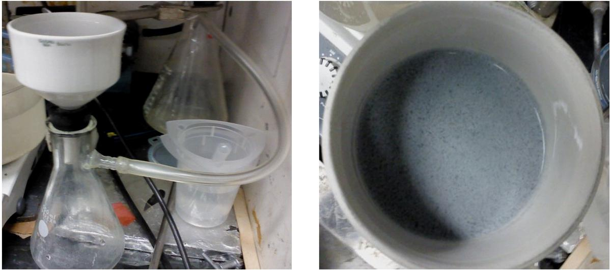
**Figure A 4.      Recuperation step: Vacuum filtration**
