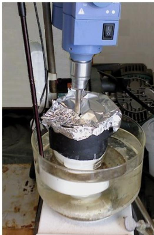
Figure A 3. a) Emulsification b) *In-situ* polymerization reaction
