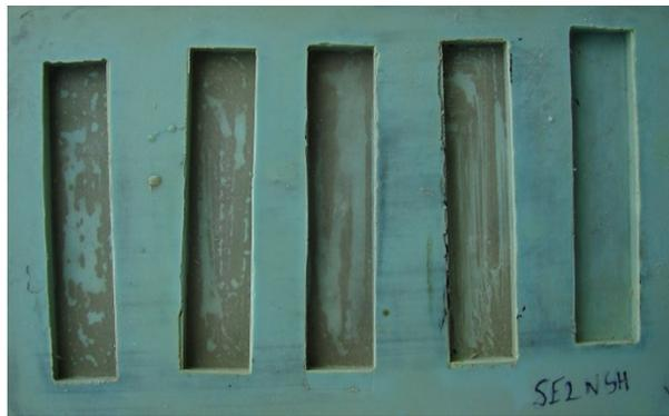
c) After curing and demolding the tool, the mold is ready to use.
