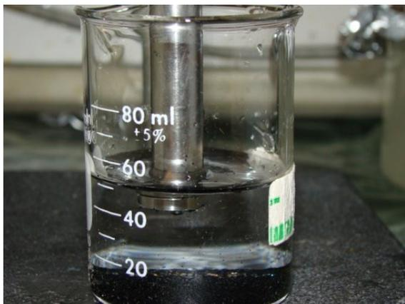
CNT (0.1 wt.%) in 5E2N before ultrasonication
