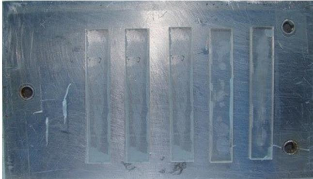
b) Preparation of tools for the desired size of samples. Mold rubber and catalyst in 10:1 ratio are mixed and poured upon these tools, cured at RT for 48 h
