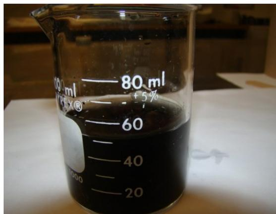
5E2N/CNT suspension after ultrasonication
