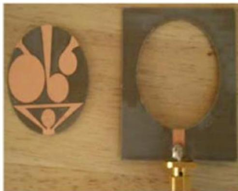
Figure 19 Antennes correctives reconfigurables de type rotatif (Tawk, 2010)
