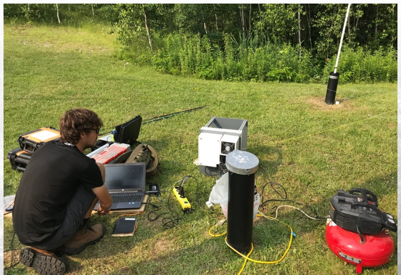
Oscillatory hydraulic tomography tests between wells for the development of a new high-resolution characterization technique for aquifer systems.
