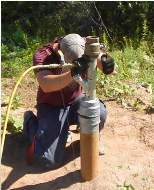
Permeability tests (slug tests) with compressed nitrogen for the evaluation of hydraulic conductivity
