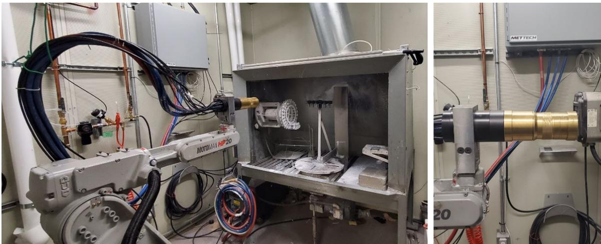
**Figure II.1. Suspension plasma spray with a Mettech's Axial III gun.**
