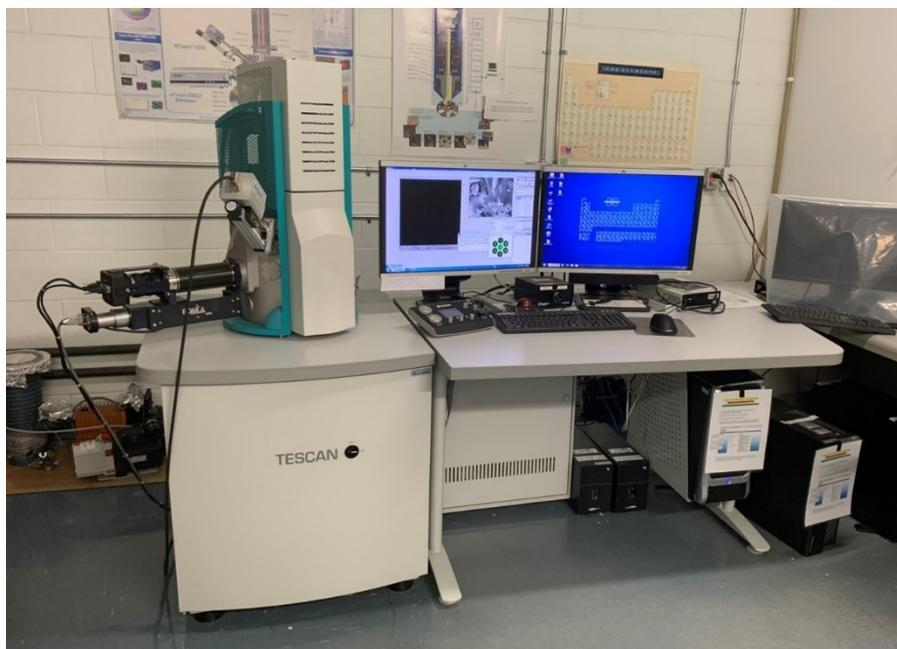
**Figure II.5. Tescan Vega3 scanning electron microscope equipped with a Bruker XFlash® 6 | 10 Detector energy dispersive X-ray spectroscope (EDX) used in this thesis.**
