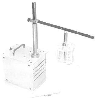
Figure 12. *Vander Kamp Disintegration tester*
