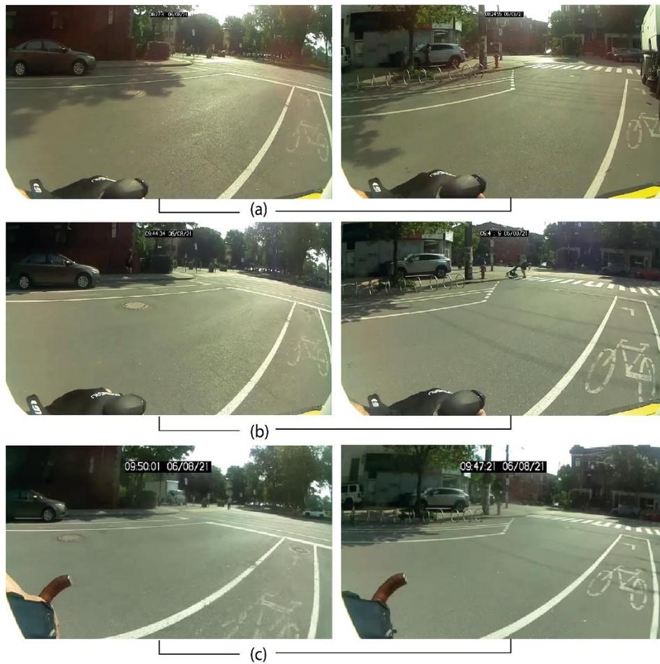
**Figure 4.9 :** Different resolutions of the 1m+ camera sensor (a) 920 x 540 px (b) 720 x 405 px (c) 480 x 270 px
