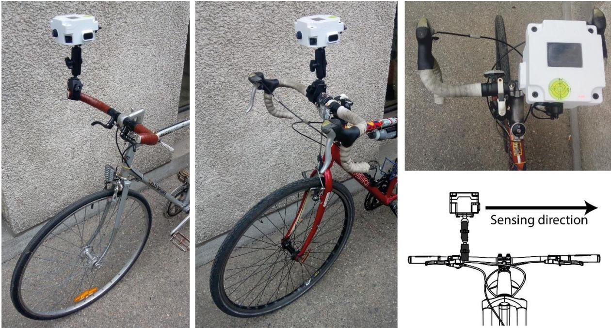
**Figure 4.3 :** Integration of the one metre plus sensor to the bicycles
