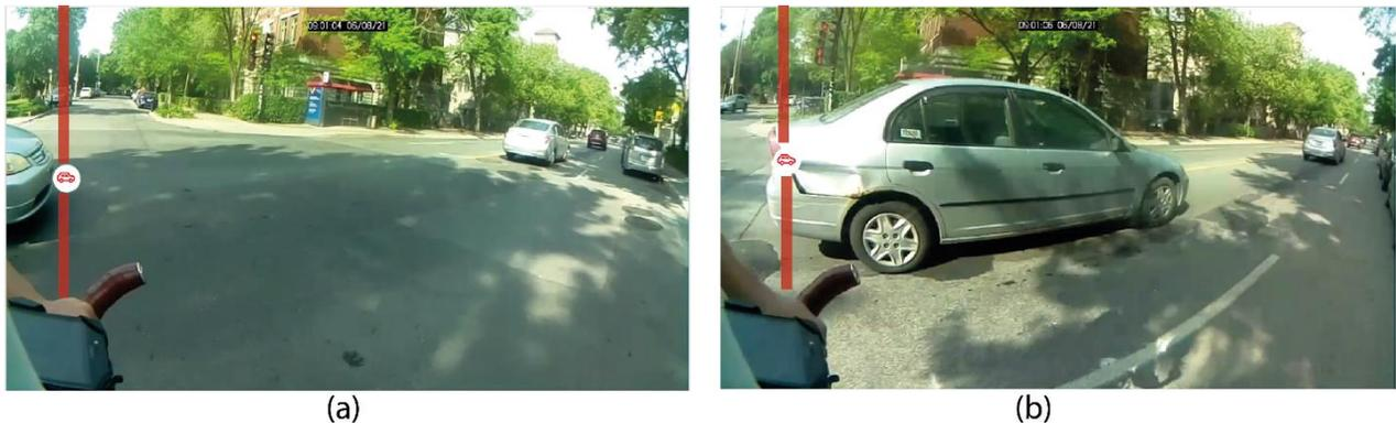
**Figure 4.6 :** Characterization of overtakings on Vifeco. **(a)** beginning of overtaking aligned with cyclist's handlebars; **(b)** end of overtaking.
