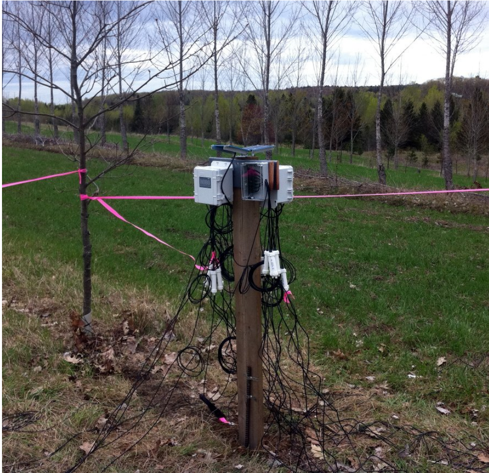
Figure 2.6: Two Onset Hobo U30 monitoring systems mounted on a wooden support firmly attached to the soil.
