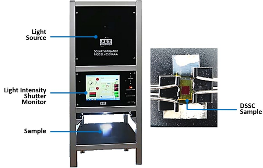
Figure 2-4 Setting for PV measurement and device
